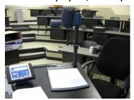
• Located near the working surface area of the Wolf Vision are the brightness and power options. Make sure the power is on as indicated by a green light.
