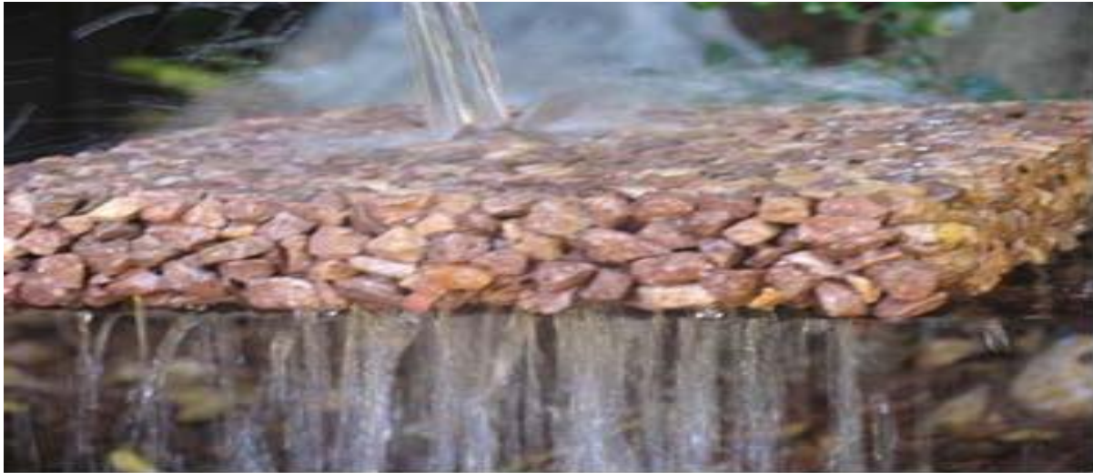
Figure 21: Water flow through permeable pavement
