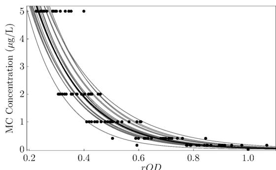
**Figure 3.** Standard curves fitted using BHM show a reduced among test variation (compared to Figure 1(c)). The thick dark line is the mean model characterized by  $\mu_0$  and  $\mu_1$  in eq 4. The thin shaded lines are test-specific models characterized by  $\beta_{0j}$  and  $\beta_{1j}$  where  $j = 1, \dots, 21$ , the index of the 21 tests.
