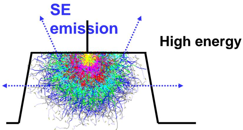
» At high energy the interaction volume fills features on the surface - SE2 emission leads to enhanced SE emission making objects look almost 3-dimensional
