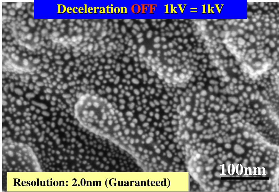
*Image clarity at 500 volts with a decelerated beam is much better than the image from an initial 500-volt beam. The estimated resolution at 500 volts with beam deceleration is equivalent to the guaranteed resolution of a 1kV beam.*
