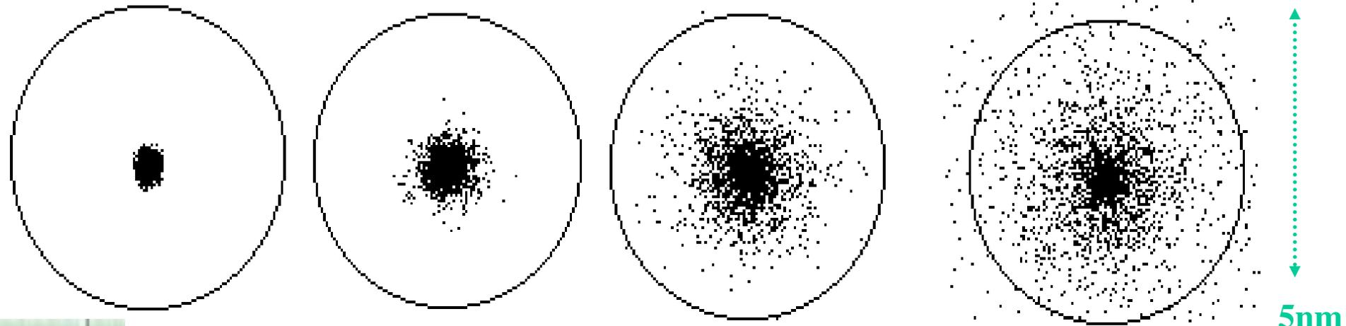
Kenway-Cliff numerical ray-tracing simulations of electron arrivals with a lens  $C_s=3\text{mm}, C_c=3\text{mm}, \alpha =7 \text{ m.rads}$
