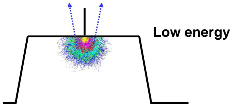
» But at low energies the reduced interaction volume means that only the edges of features are enhanced
