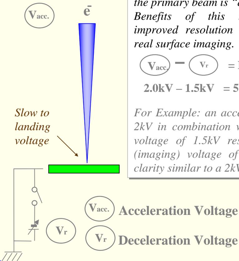
By applying a voltage ( $V_r$ ) to the stage the primary beam is “decelerated”. Benefits of this technique include improved resolution at lower kVs and real surface imaging.
