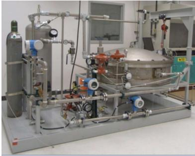
carbon dioxide emissions have led the Department of Energy to solicit ideas for carbon dioxide capture from coal-fired power plants. Professor Lipscomb's group is working with Membrane Technology and Research, Inc. to develop a process based on membrane technology. The process using sheets of plastic to selectively remove carbon dioxide from flue gas. Professor Lipscomb and his students are working to
