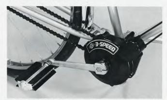
**STEP FOUR:** Attach twist grip, crank arms and existing pedals. Shorten chain and attach.
