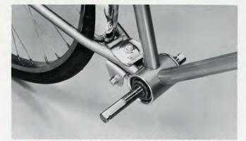
**STEP TWO:** Install new mainshaft utilizing existing bearings and cones.
