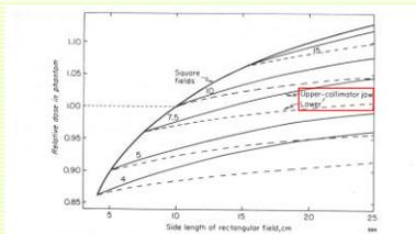
Figure 10-13. Relative output data for a 25 MV linear accelerator. The outputs were measured at a depth of 7 cm in a water phantom and are expressed as fractions of the output for a  $10 \times 10$  cm field.
