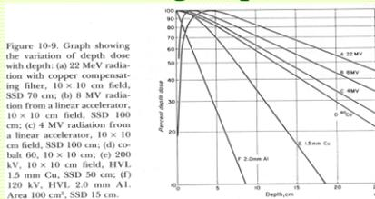
Figure 10-9. Graph showing the variation of depth dose with depth: (a) 22 MeV radiation with copper compensating filter,  $10 \times 10$  cm field, SSD 70 cm; (b) 8 MV radiation from a linear accelerator,  $10 \times 10$  cm field, SSD 100 cm; (c) 4 MV radiation from a linear accelerator,  $10 \times 10$  cm field, SSD 100 cm; (d) cobalt 60,  $10 \times 10$  cm; (e) 200 kV,  $10 \times 10$  cm field, HVL 1.5 mm Cu, SSD 50 cm; (f) 120 kV, HVL 2.0 mm Al, Area 100 cm<sup>2</sup>, SSD 15 cm.
