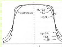
Parameters  $\alpha_1$ ,  $\alpha_2$ , and t are determined by best fit of measured profiles
