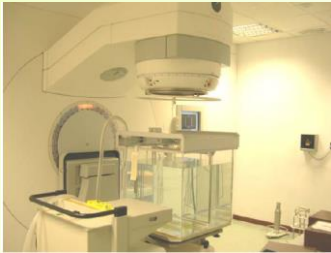
View of the Elekta linac upper head for 6 MeV X-ray beams and the water phantom
