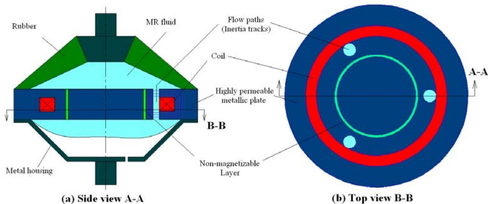
**Figure 1: Schematic of the MR mount (a) Side view, (b) Top view.**
