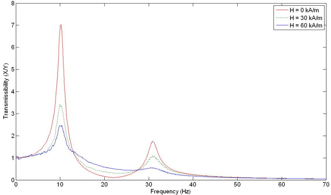
**Figure 7: Displacement transmissibility of the mount with varying field.**
