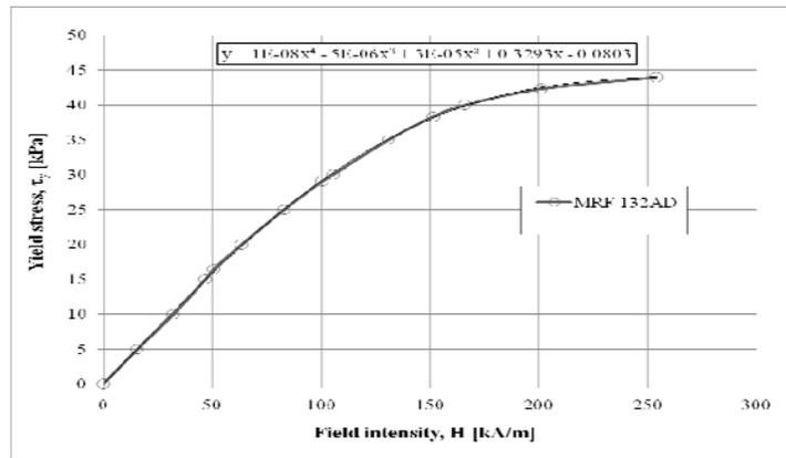
Figure 4: Yield stress as a function of magnetic field intensity for MRF-132AD.
