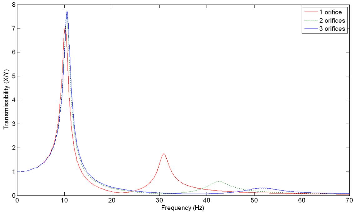
**Figure 6: Displacement transmissibility of the mount with the field off when the number of the inertia tracks change.**
