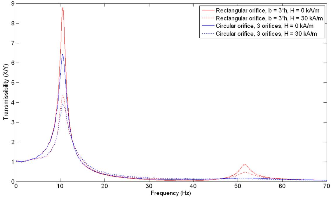
**Figure 10: Comparison of a rectangular orifice with width = 3 x height and 3 circular orifices, the overall areas are equal.**
