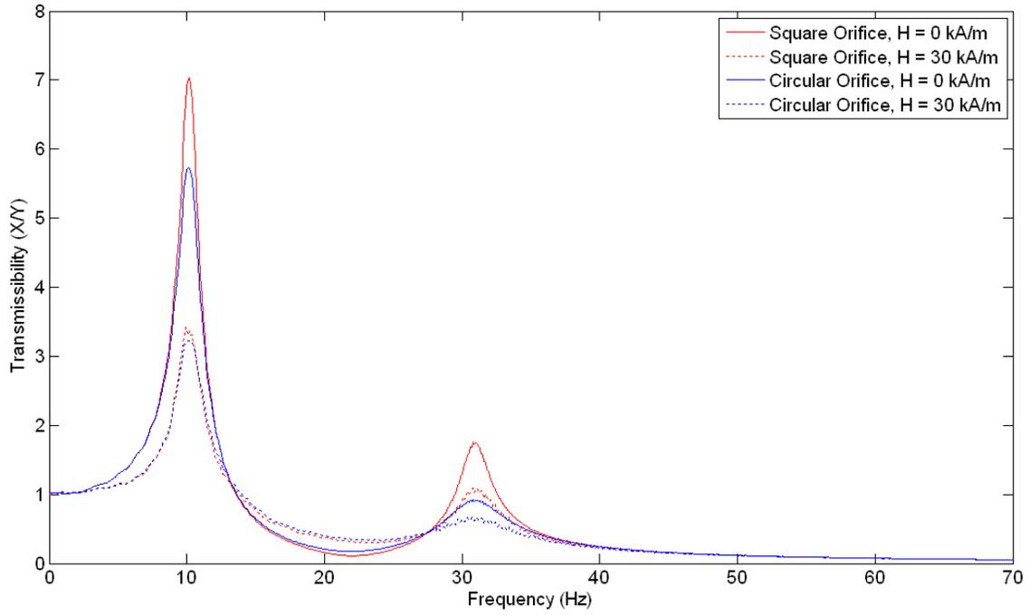
**Figure 8: Comparison of square and circular orifices with equal cross-sectional area.**
