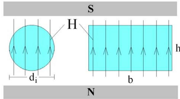
**Figure 3: Geometry of the orifice in relation with the magnetic field direction.**
