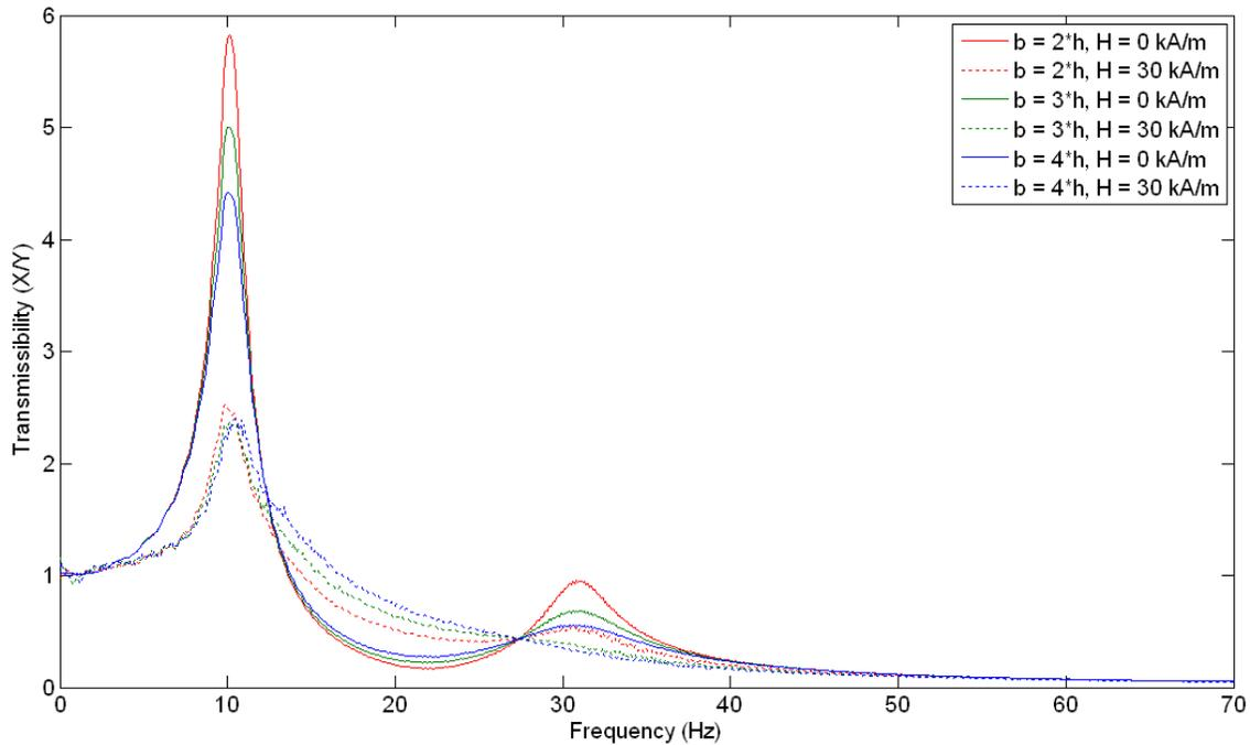
**Figure 11: Comparison of rectangular orifices with different ratio between the width and the height, the overall areas are equal.**
