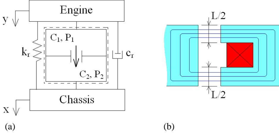
Figure 2: (a) Physical model of the mount; (b) Effective length of the inertia track.
