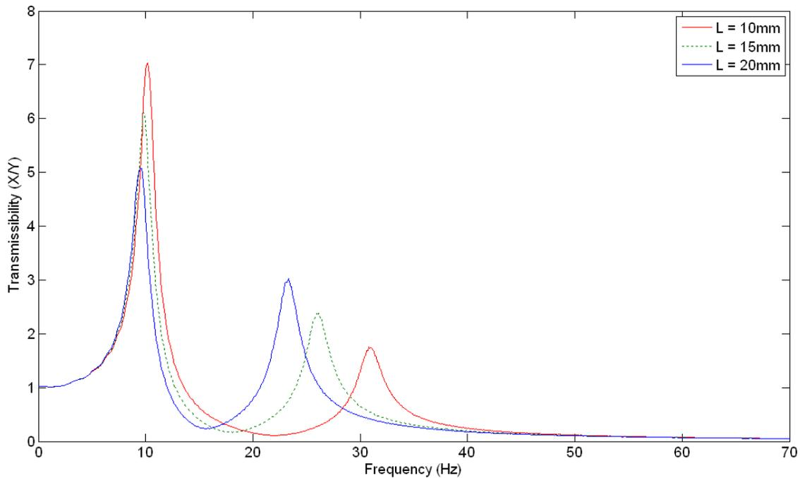
**Figure 5: Displacement transmissibility of the mount with the field off when the length of the inertia track changes.**
