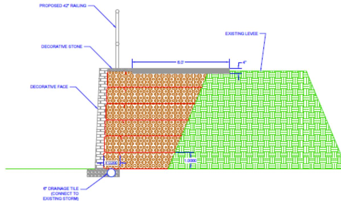
Figure 30: Retaining Wall Cross Section
