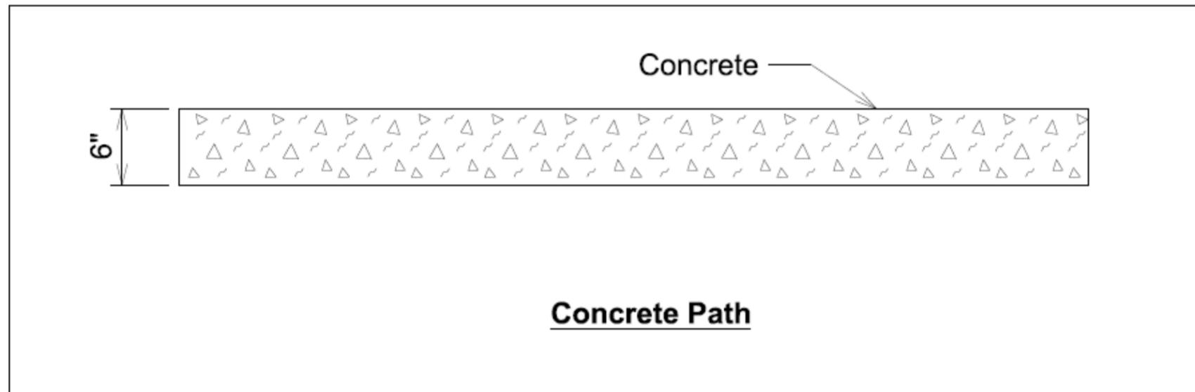
**Figure 28: Regular Concrete Path Cross Section Design**
