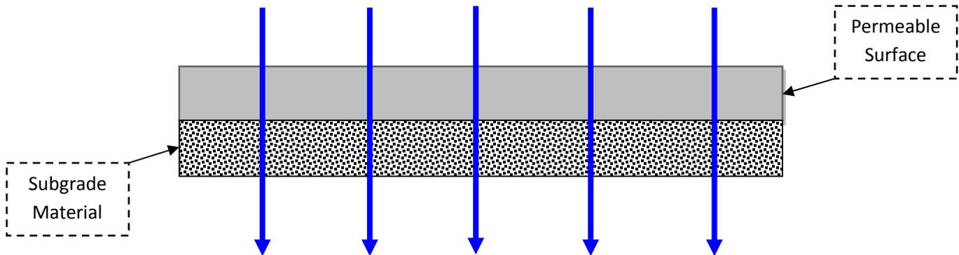
**Figure 3: Permeable Pavement**
