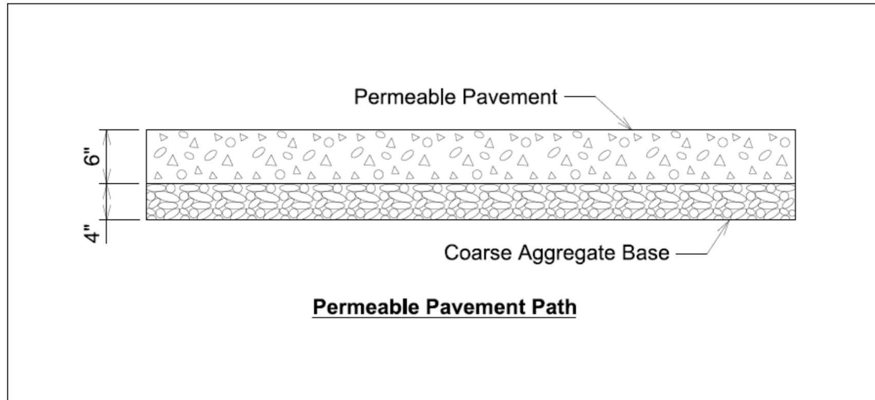
**Figure 29: Permeable Concrete Path Cross Section Design**
