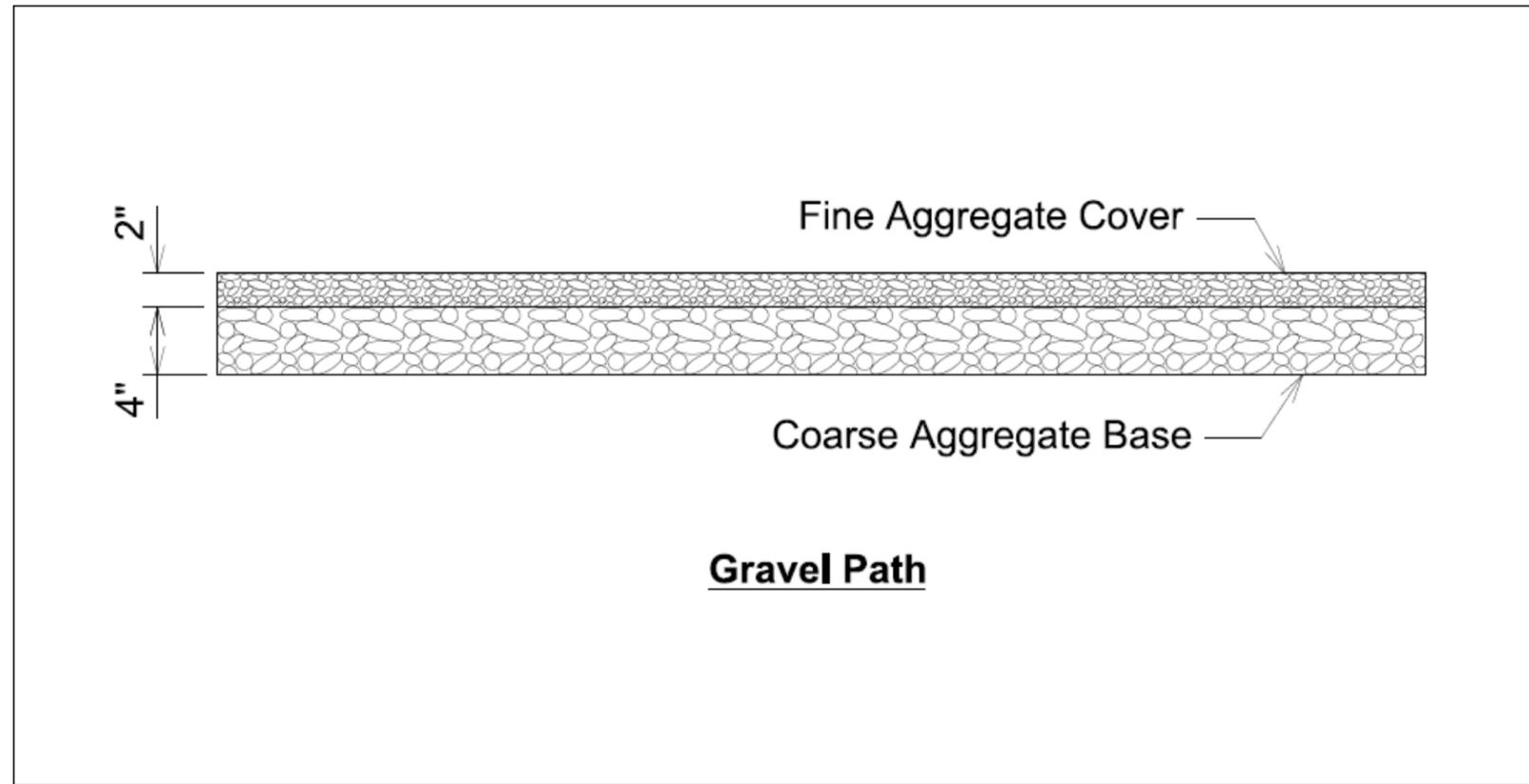
**Figure 27: Gravel Path Cross Section Design**
