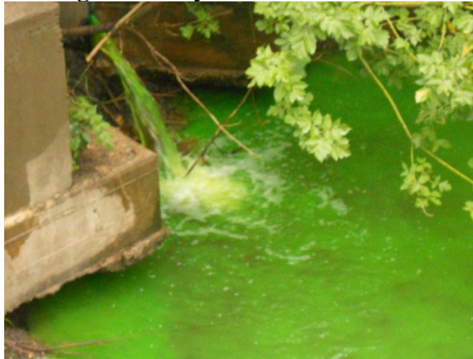
Figure 24: Dye Test Confirmation
