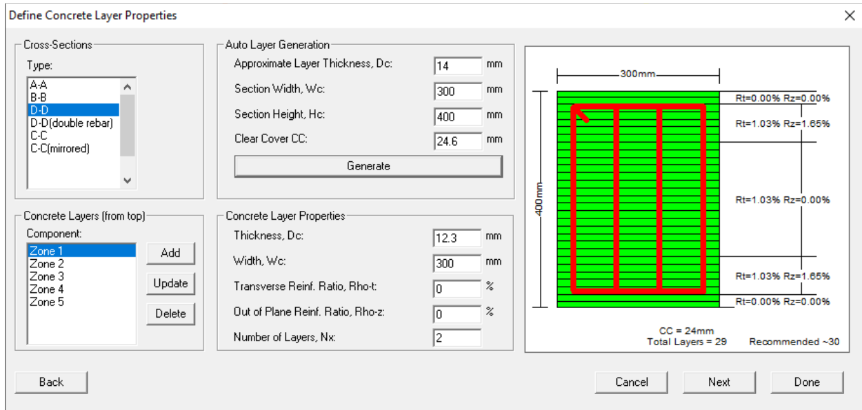
Figure 6 – Second window of the “Define Materials” section where all of the details of the concrete layers are input or generated for each section.
