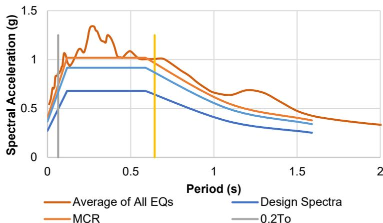
Fig. 1 Design response spectrum, MCER plot and the average design spectra of the considered earthquakes satisfying the given condition.
