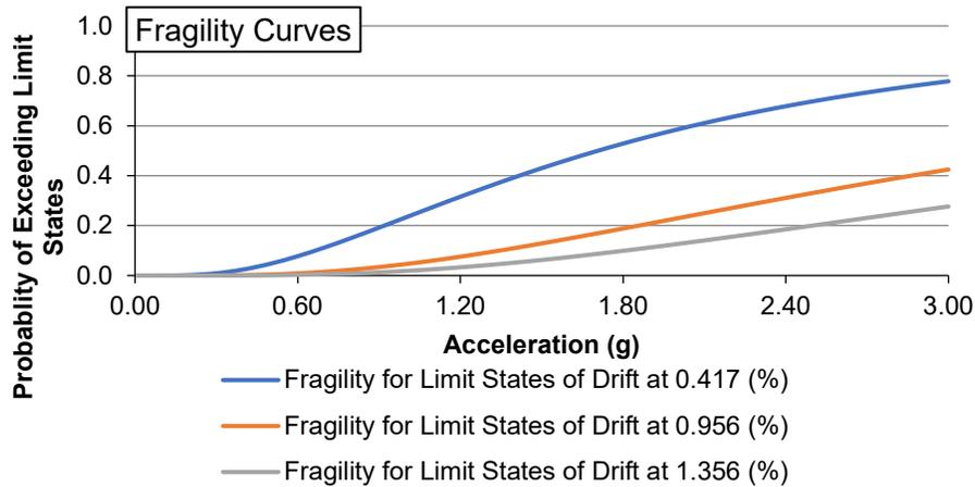
Fig. 3 Fragility plot for Wall 1.2 from 11 strong ground motion records and 10 intensities per record.
