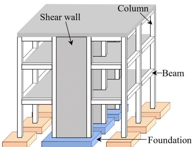
Fig. 2. Shear wall alternative.
