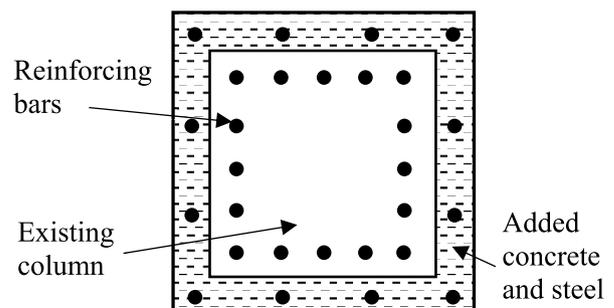
Fig. 1. RC column jacketing alternative.
