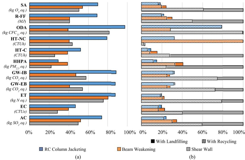
**Fig. 10.** (a) Recycle/landfill ratio of environmental impacts for the disposal phase of each retrofit alternative and (b) total environmental impact comparison with and without consideration of recycling.
