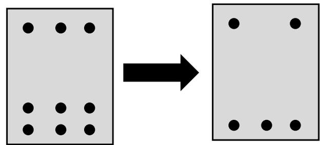
Fig. 3. Beam weakening alternative.
