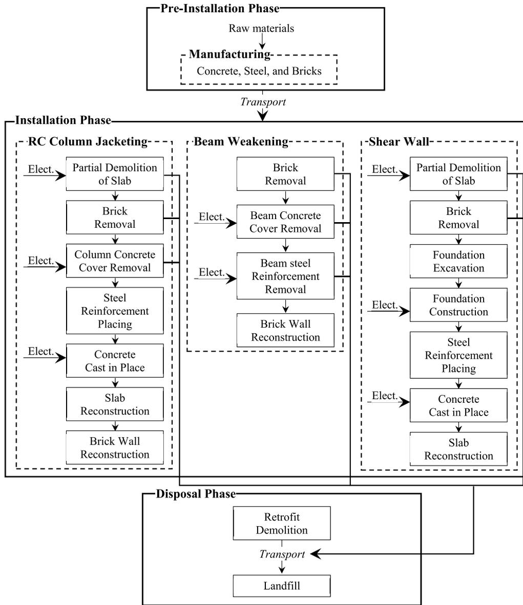
Fig. 6. Flowchart for the RC column jacketing (A), shear wall (B) and beam weakening (C) alternatives.
