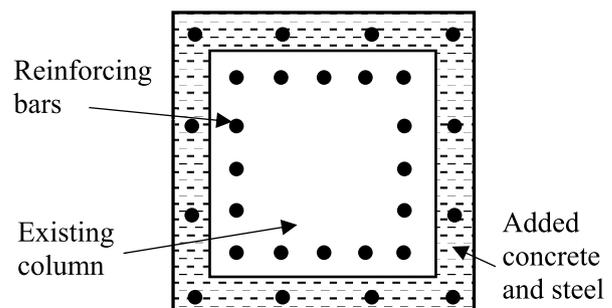
Fig. 1. RC column jacketing alternative.
