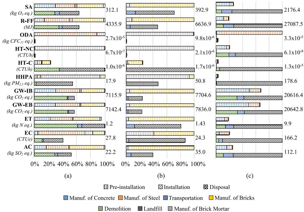
Fig. 7. Detailed environmental impacts of the (a) RC column jacketing, (b) beam weakening, and (c) shear wall alternative.
