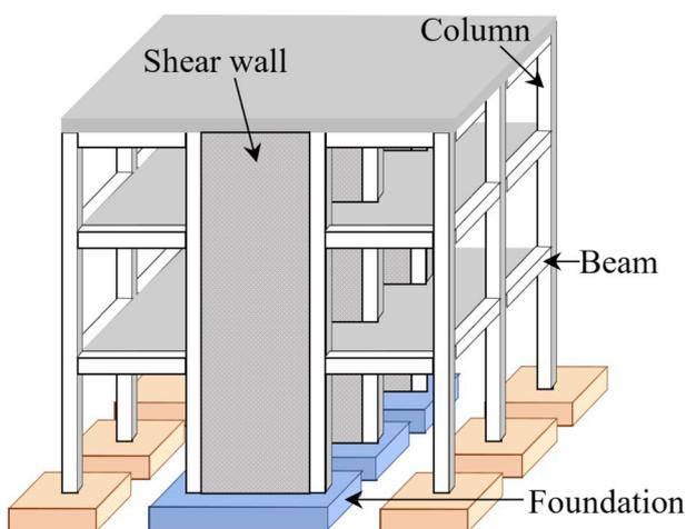
Fig. 2. Shear wall alternative.
