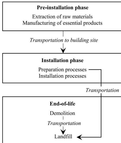
Fig. 5. LCA phases considered.
