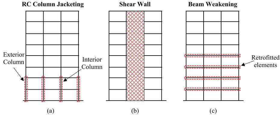
**Fig. 4.** Affected elements of the original structure in the calculated design of (a) RC column jacketing, (b) shear wall, and (c) beam weakening retrofit alternatives for the collapse prevention limit state.
