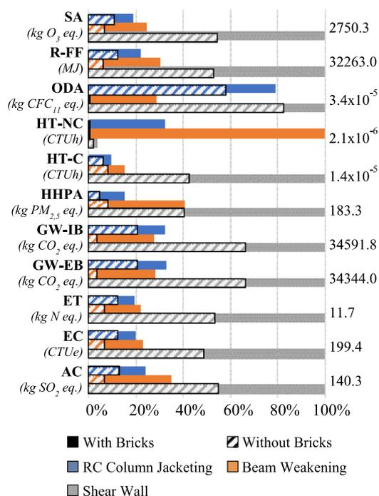
Fig. 9. Total environmental impacts of the three retrofit alternatives with and without concrete bricked walls.
