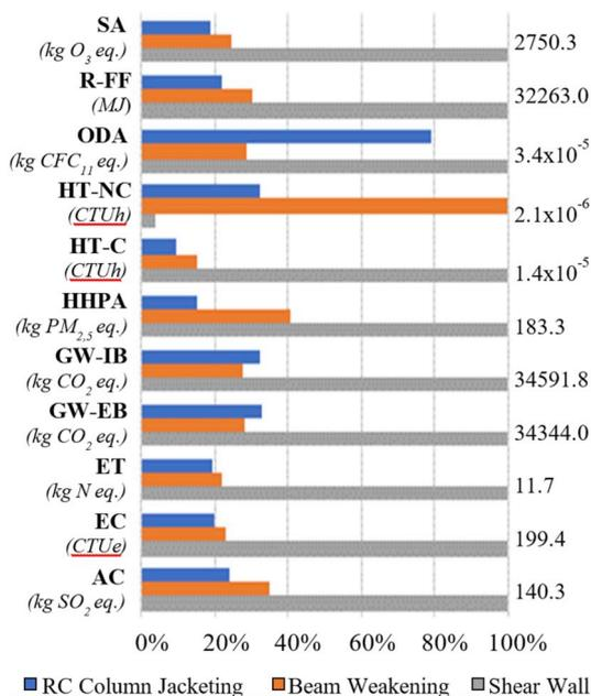
Fig. 8. Total environmental impacts of the three retrofit alternatives.
