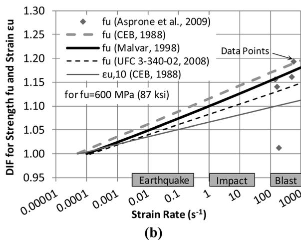
Fig. 3—Strain rate-DIF relationships for reinforcement in tension.
