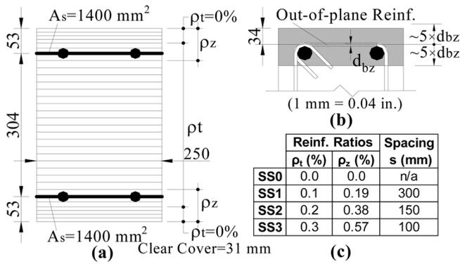
Fig. 5—SS beams: (a) sectional models used; (b) determination of tributary area for out-of-plane reinforcement; and (c) smeared reinforcement ratios used. (Note: 1 mm<sup>2</sup> = 0.00155 in.<sup>2</sup>)
