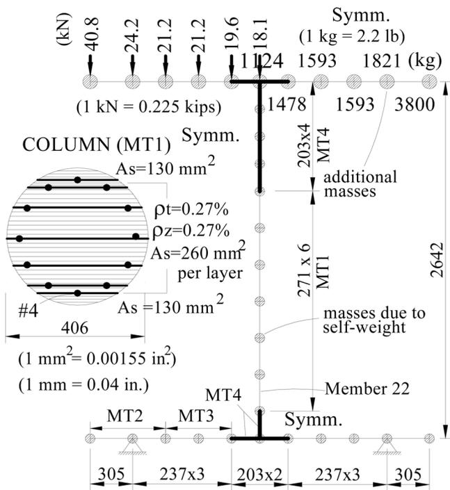
Fig. 10—Specimens A1 and B1: frame model used.
