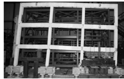
(a) Experiment failure mode (Ghannoum and Moehle, 2012)
