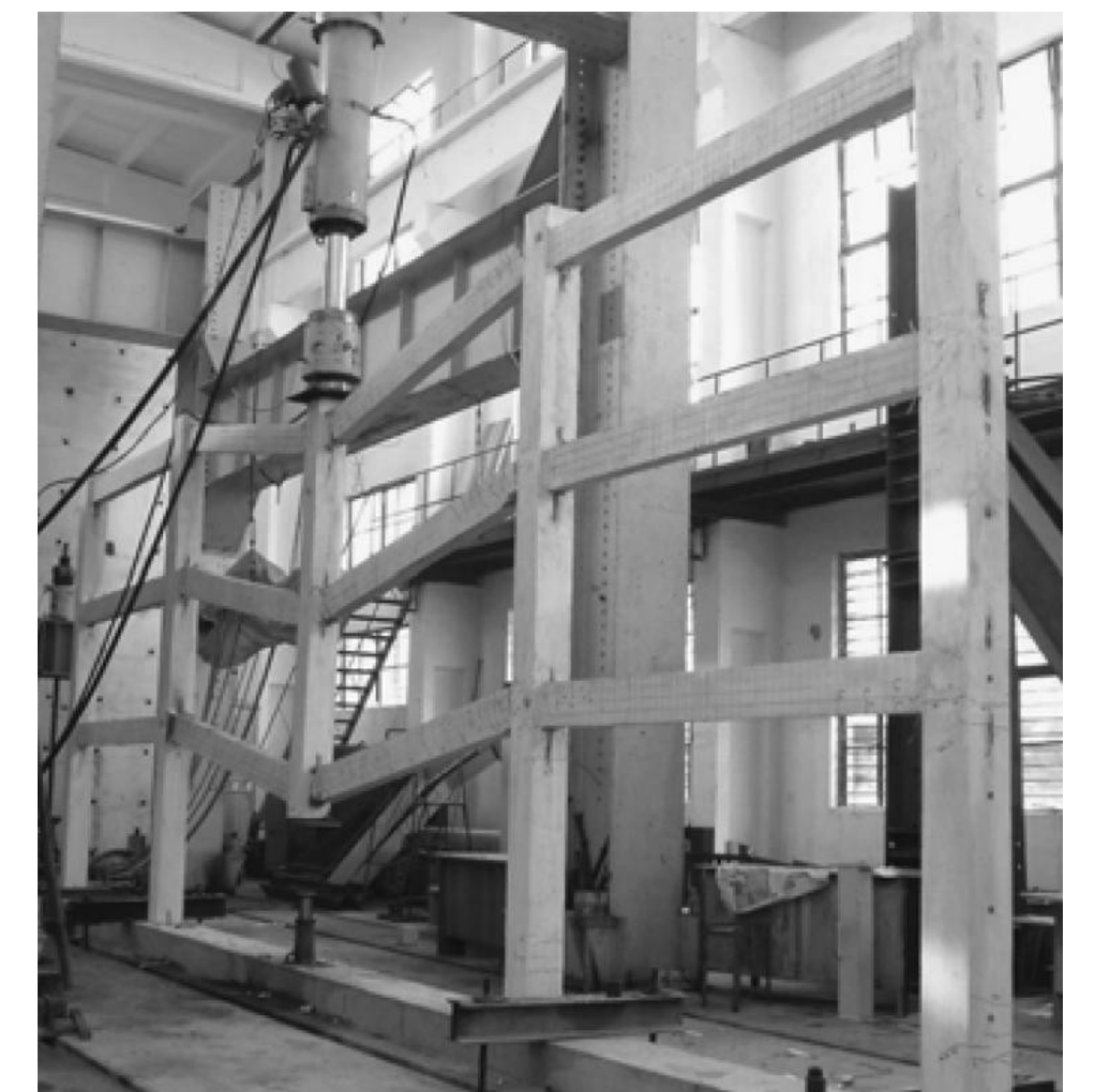
Fig. 6. Experiment: Collapse Limit State (Yi et al., 2008)
