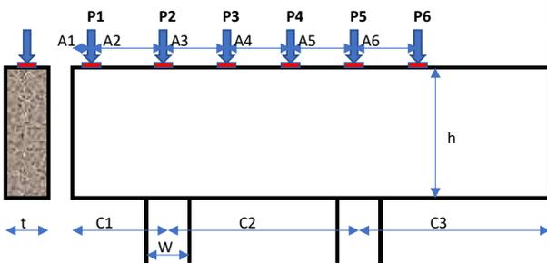
**Note:** Input for Section 3 and Section 4 is based on the above-generated sketch. The loads shown in the above sketch are not the actual loads; these are shown for representation only.
