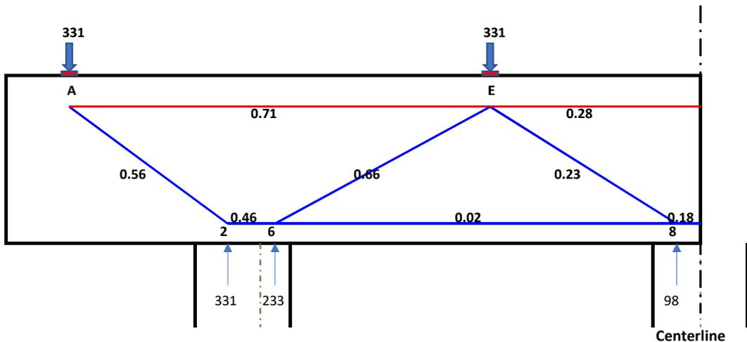
**Note:** The above figure shows the output model with Utilization Ratio along with the member which are color coded. The node numbers are also printed for every node. This output model is based on below calculation details.
