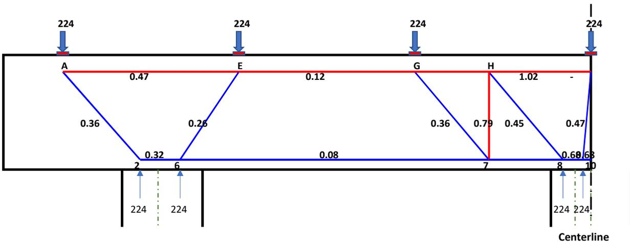
**Note:** The above figure shows the output model with Utilization Ratio along with the member which are color coded. The node numbers are also printed for every node. This output model is based on below calculation details.
