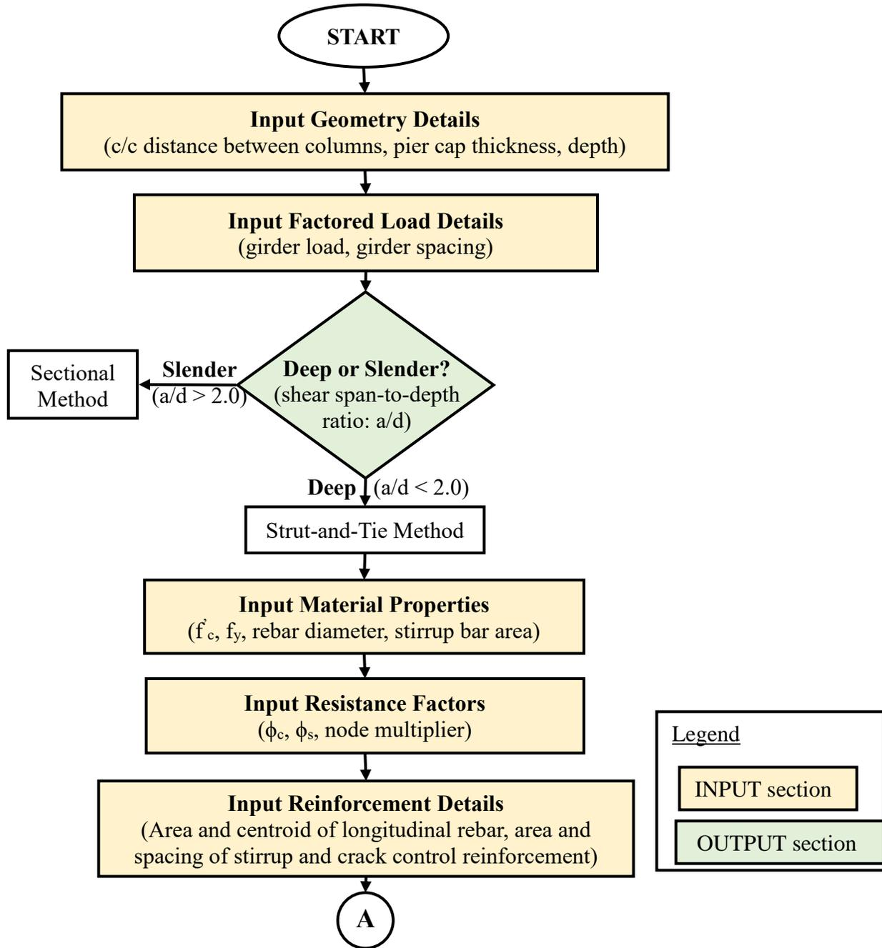
**Figure 3** Flowchart for the STM-CAP solution procedure (part A).
