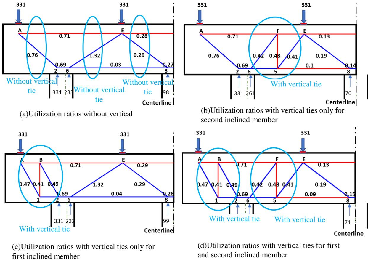
**Figure 6** Optimization of utilization ratios with various truss models.
