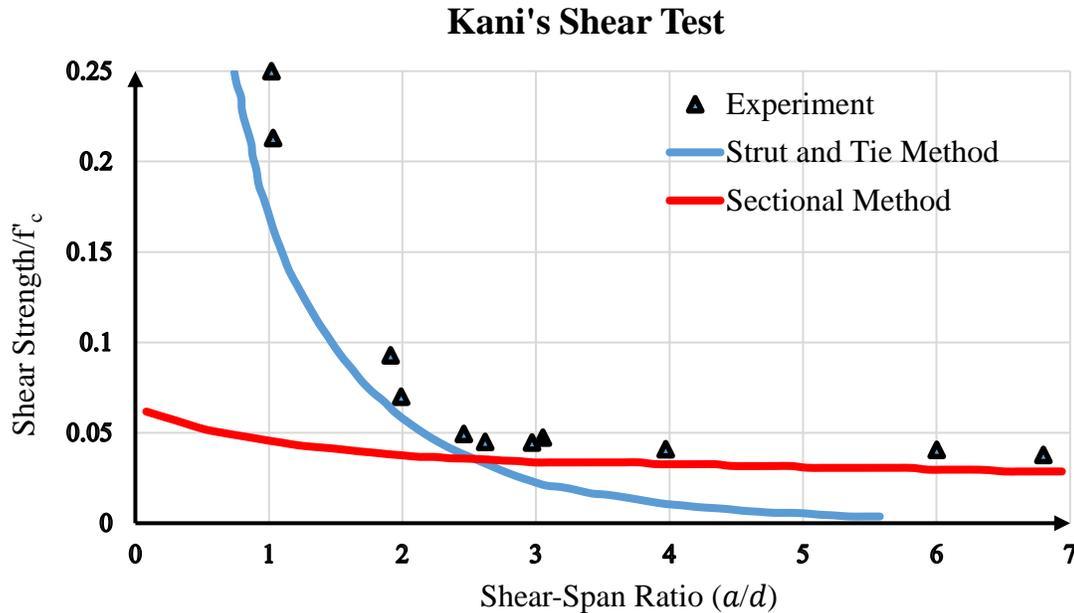
**Figure 1** Shear strength vs  $a/d$  ratio (Kani, 1964).
