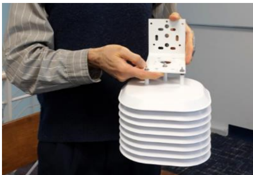
(a) External logger-radiation shield bundle
