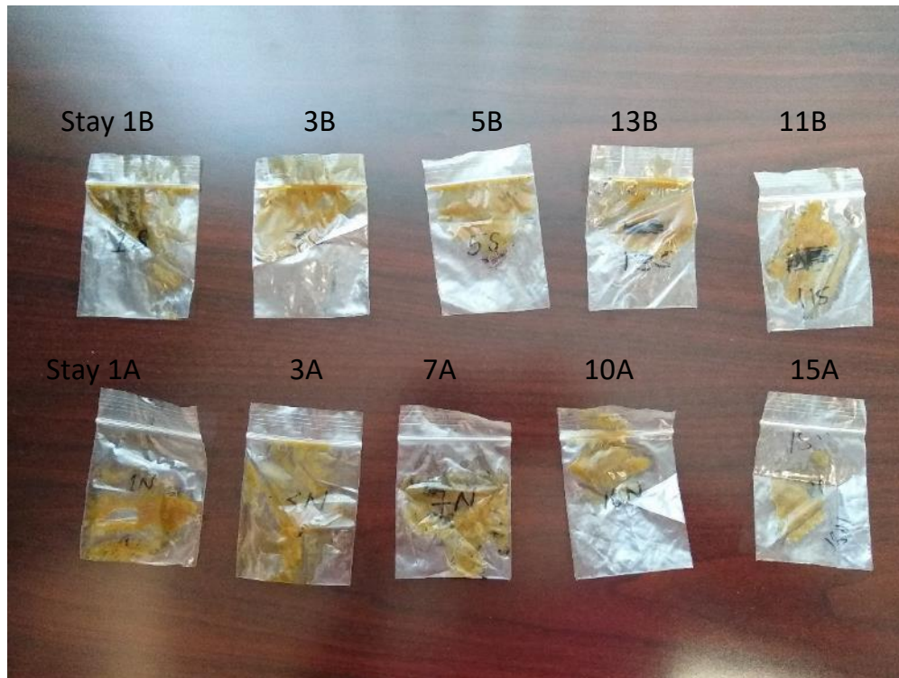
Figure 9 Grease samples collected from the lower anchorage zones.
