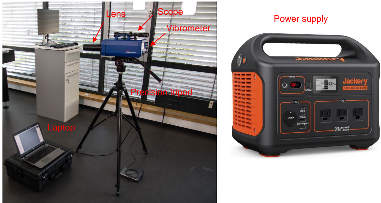
Figure 26 Laser Vibrometer test setup used.
