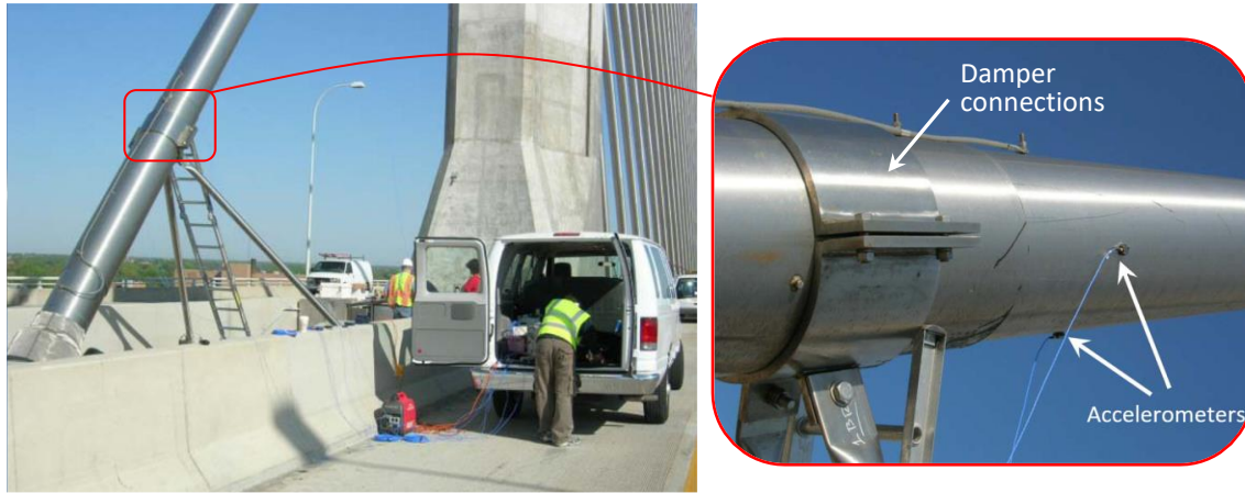
Figure 24 Accelerometer testing performed on VGCS stays after construction.
