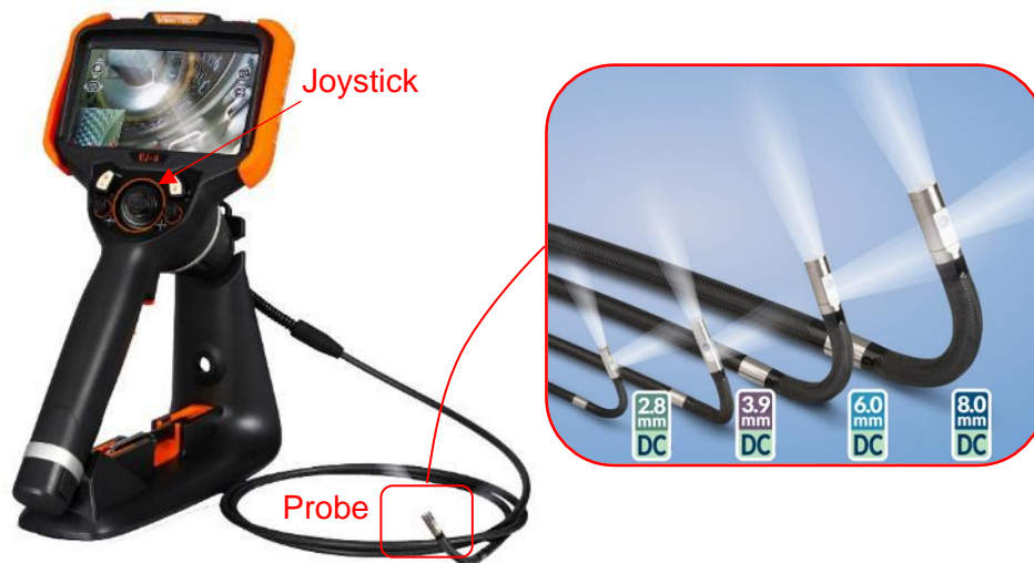
Figure 6 Sample borescope with a dual-view camera.
