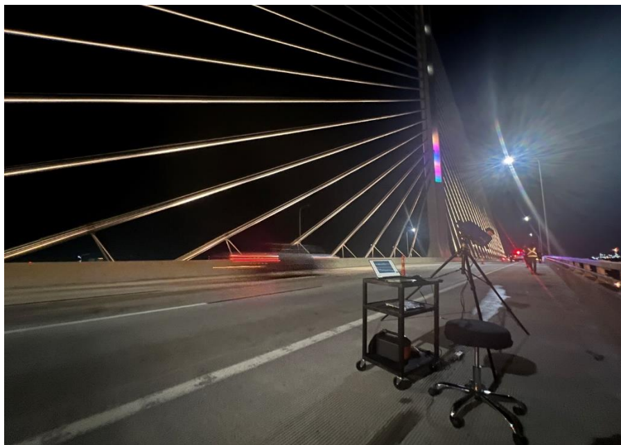
Figure 31 Test setup on the deck of VGCS at the north of the pylon.
