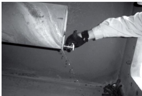
(b) Water exiting the end cap of the anchorage
