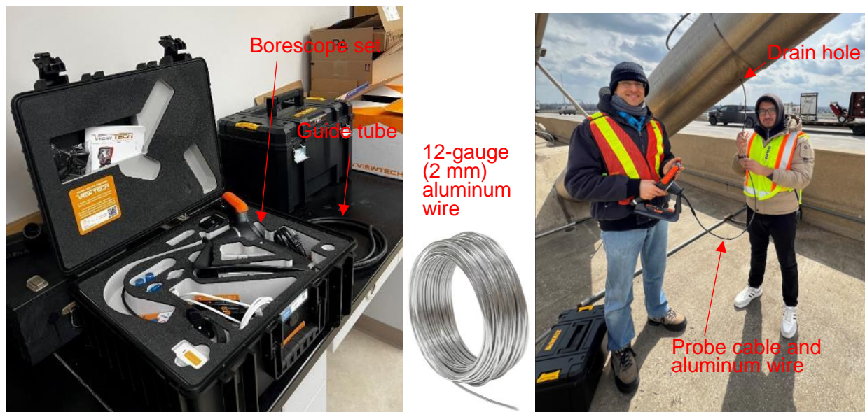
Figure 7 Boreoscope setup used for the inspection.
