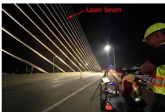
Fig. 4 (a) Stay 16B is aimed with a laser vibrometer;
