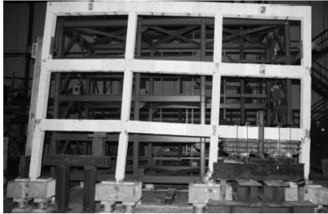
**Figure 5.55:** Failures of Ghannoum and Moehle frame (Ghannoum and Moehle, 2012)
