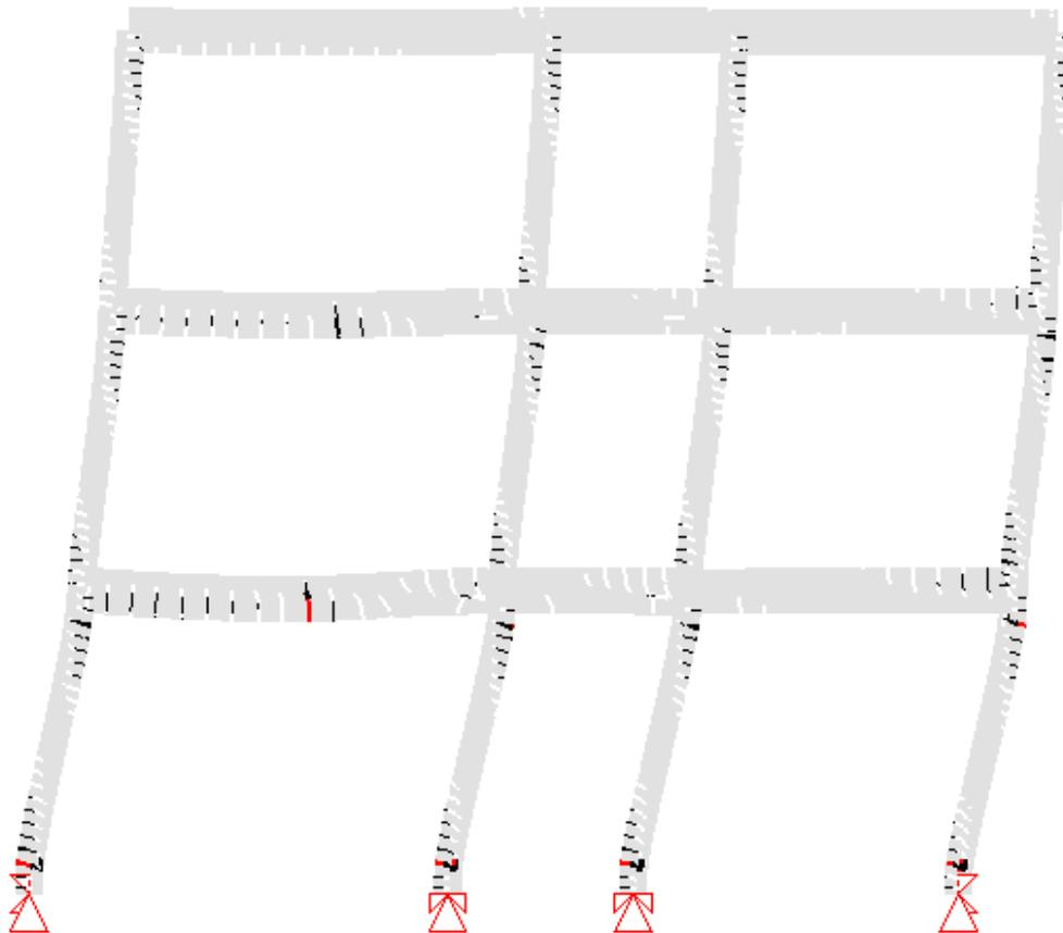
**Figure 5.64:** Deformed shape and cracking pattern of Pampanin et al. Frame
