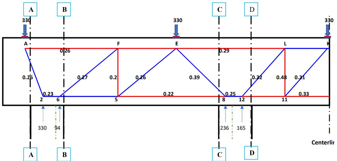
**Figure 7-19:** Utilization ratios calculated from STM-CAP for Bridge 5
