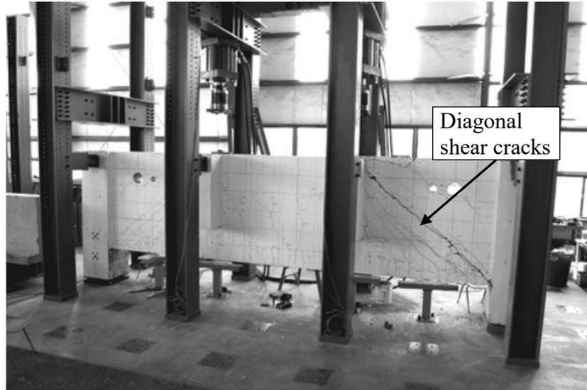
**Figure 2-5:** Shear crack in bridge pier cap (Higgins et al., 2008)
