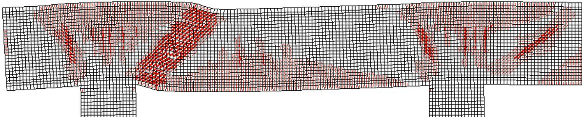
**Figure 6-52:** Cracking pattern at failure load for Bridge 4
