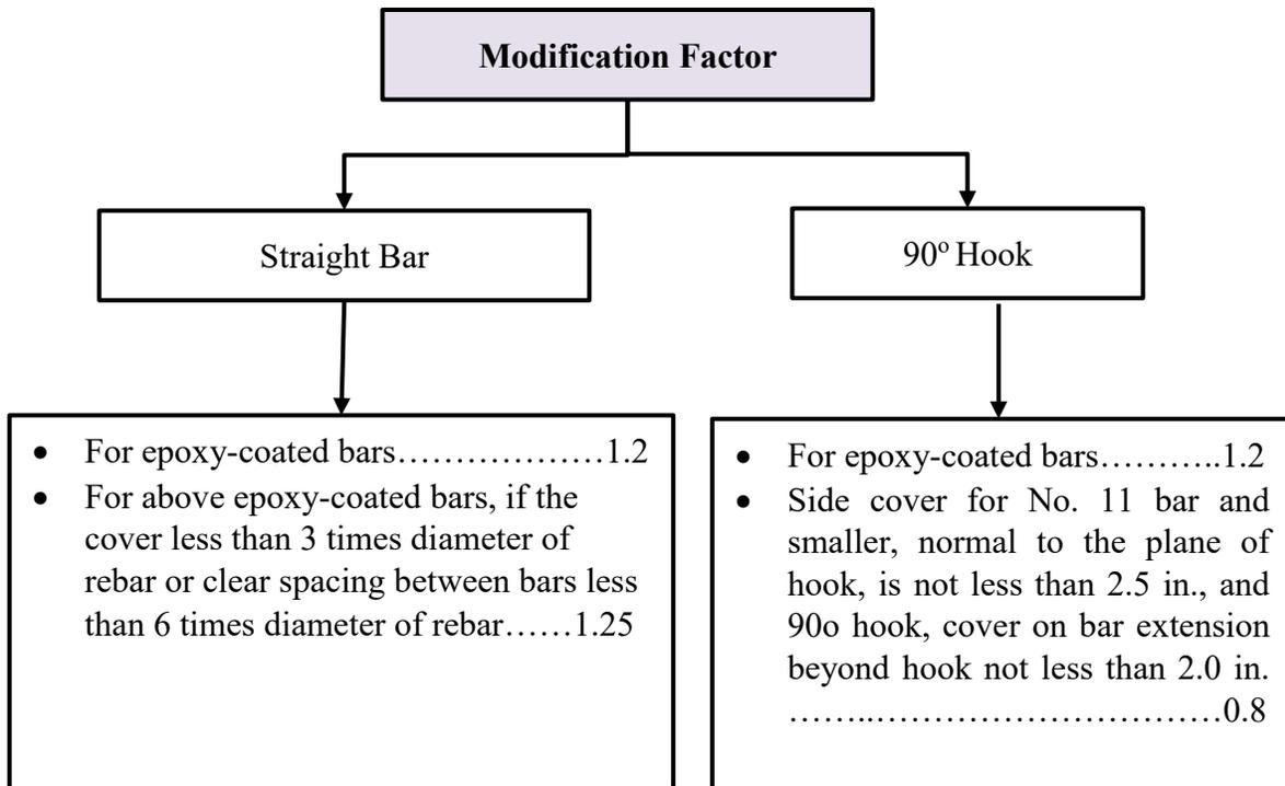
**Figure 4-20:** Modification factors for reinforcement development (AASHTO, 2017)
