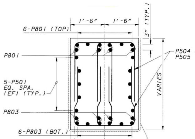
**Figure 6-56: Section of the beam for Bridge 5**
