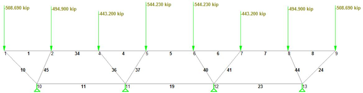
**Figure 9-1: STAAD Pro STM model for Pier Cap I**
