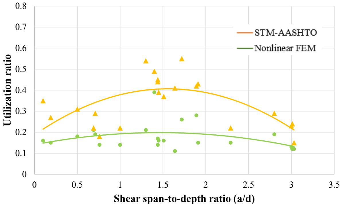
**Figure 6-64:** Comparison of utilization ratios from analysis methods with  $a/d$  ratio
