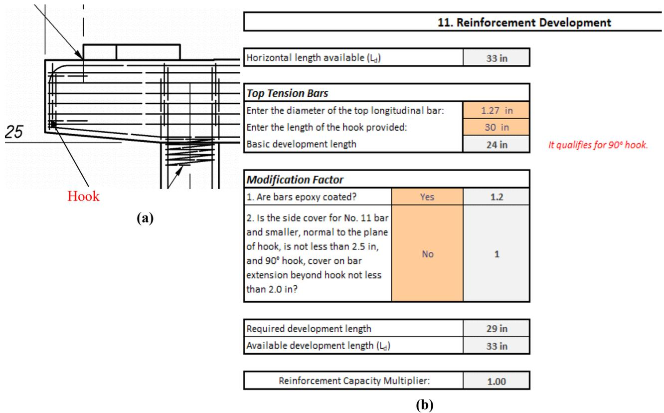
**Figure 4-21:** Sample reinforcement development input
