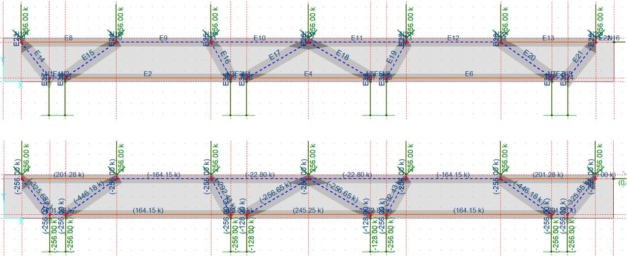
Figure 5-23: CAST model for the strut-and-tie method for Bridge 4
