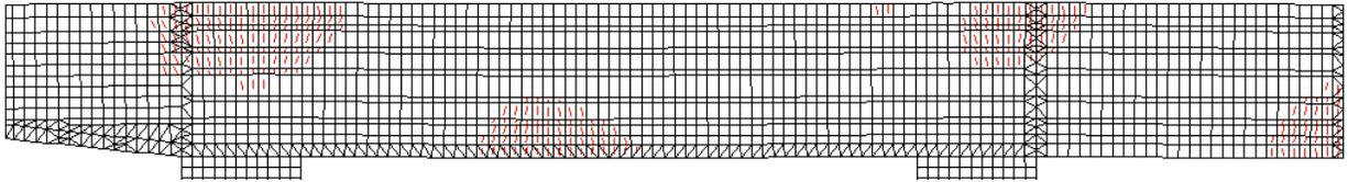
**Figure 6-44:** Cracking pattern at factored load for Bridge 3
