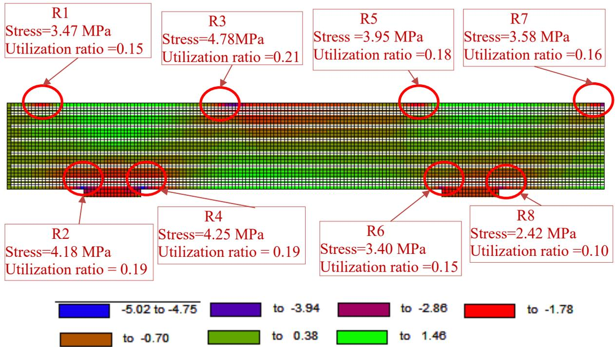
Figure 6-49: Concrete stress and utilization ratio at factored load for Bridge 4
