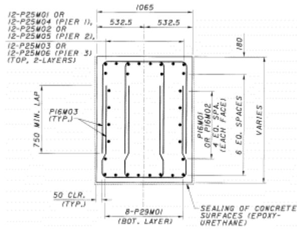
Figure 6-28: Section A-A for Bridge 2
