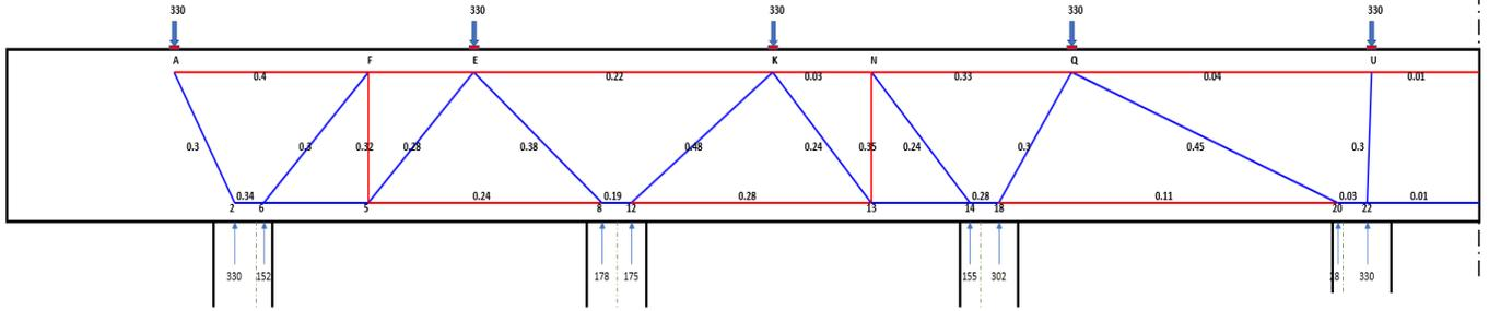
Figure 5-45: STM-CAP output model with utilization ratios for Bridge 8
