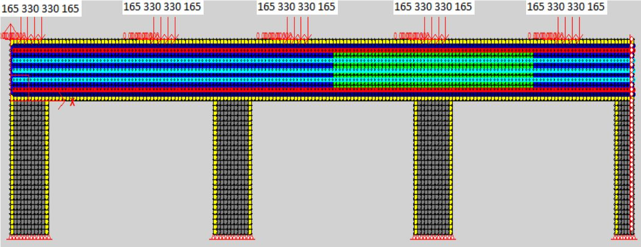
Figure 6-57: Cap beam model in VecTor2 for Bridge 5
