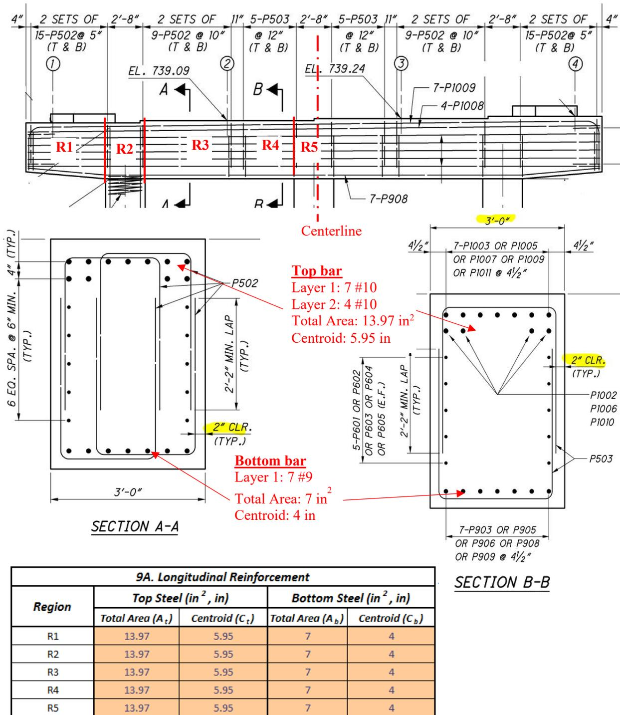
Figure 4-14: Sample longitudinal reinforcement input
