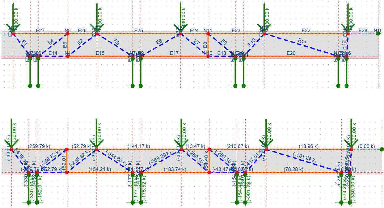
**Figure 5-47:** CAST model for the strut-and-tie method for Bridge 8
