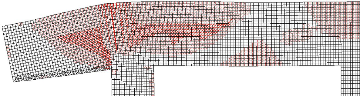
**Figure 6-15:** Cracking pattern at failure load for Bridge 1
