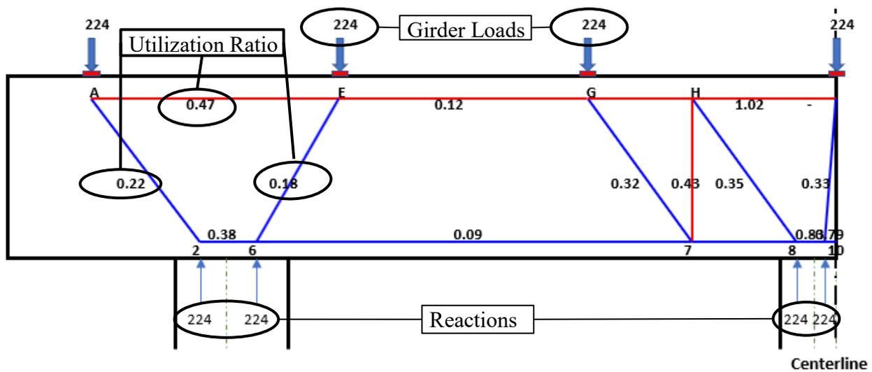
Figure 5-9: STM-CAP output model with utilization ratios for Bridge 2
