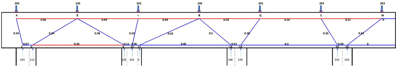
Note: The above figure shows the output model with Utilization Ratio along with the member which are color coded. The node numbers are also printed for every node. This output model is based on below calculation details.
