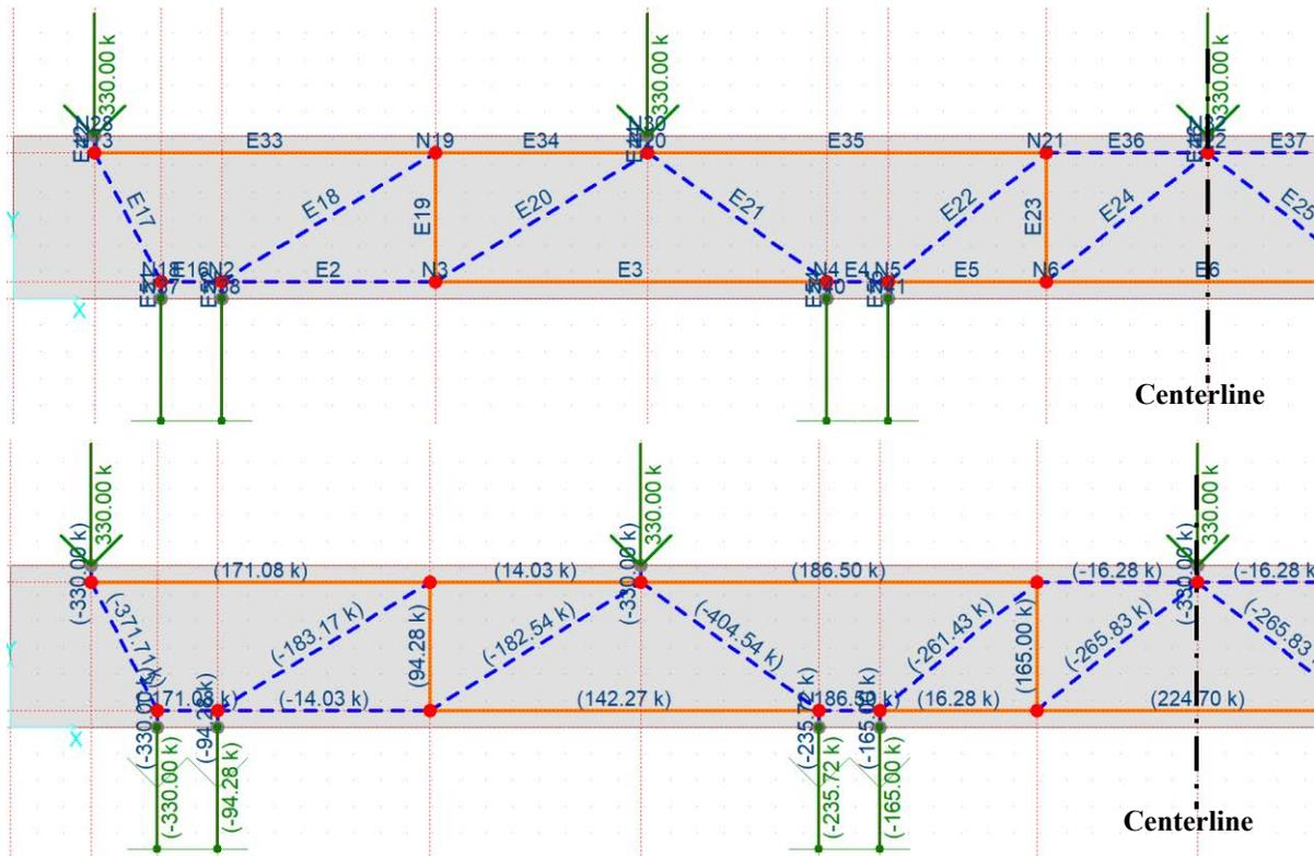
Figure 5-41: CAST model for the strut-and-tie method for Bridge 7
