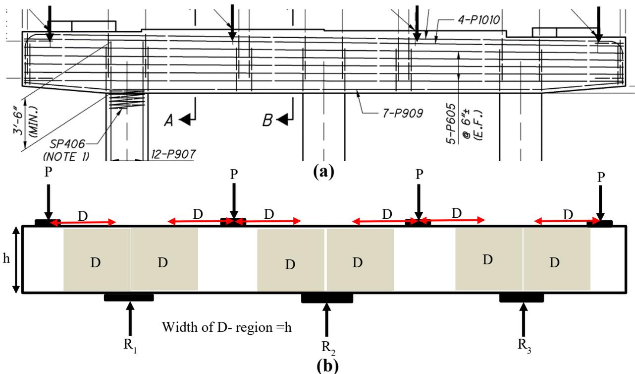
**Figure 3-2:** Illustration of D-region and B-region on pier cap of a typical cap
