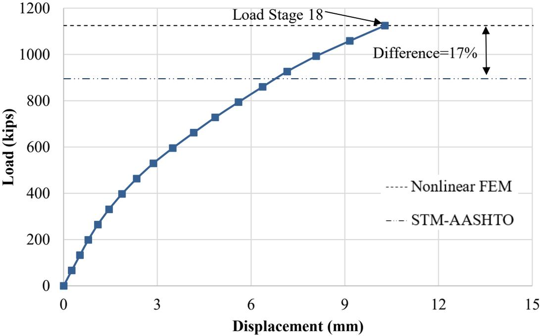
**Figure 6-26:** Load vs displacement response of cap beam for Bridge 1
