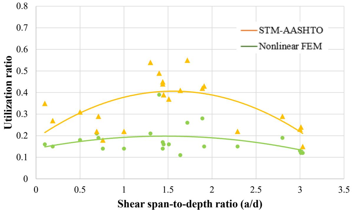
**Figure 6-1:** Utilization ratio from STM-AASHTO and Nonlinear FEM vs  $a/d$  ratio
