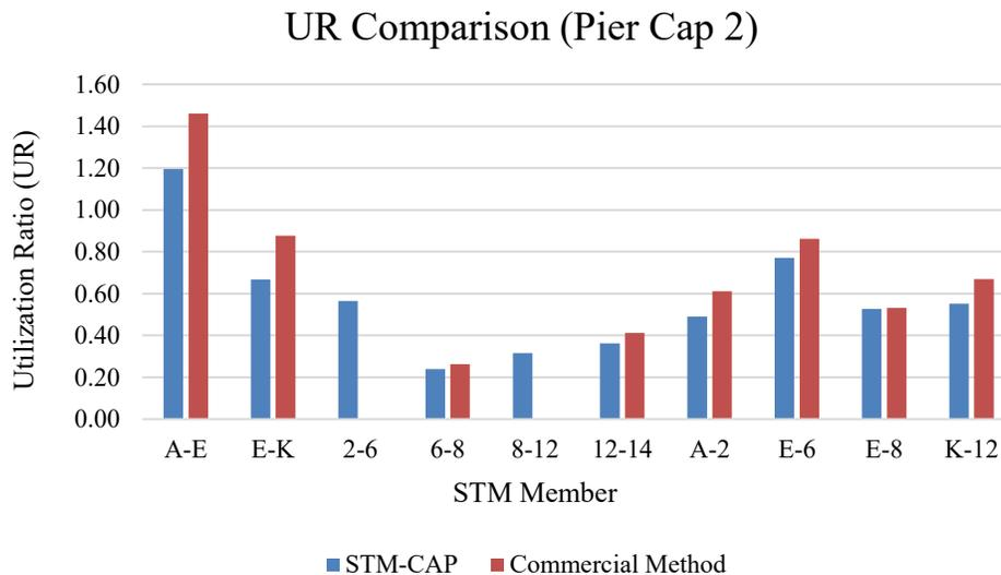
**Figure 9-5:** STM-CAP and commercial method UR comparison Pier Cap 2
