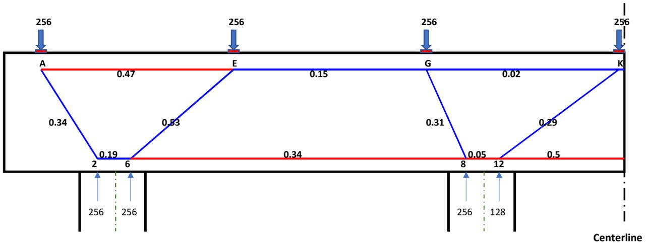
**Note:** The above figure shows the output model with Utilization Ratio along with the member which are color coded. The node numbers are also printed for every node. This output model is based on below calculation details.
