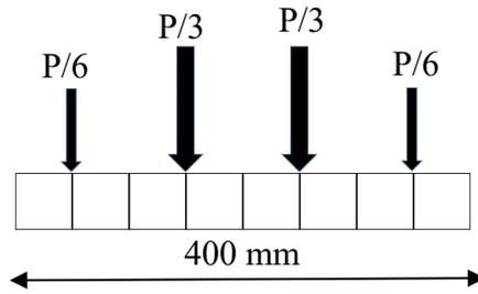
**Figure 6-6:** Loading condition for Bridge 1
