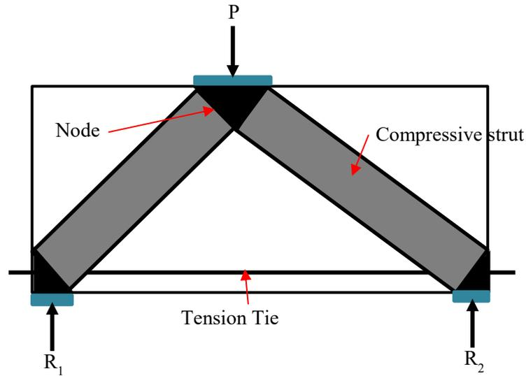
**Figure 3-3:** Strut-and-tie model in a beam
