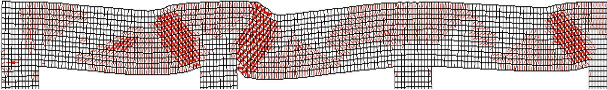
**Figure 6-61:** Cracking pattern at failure load for Bridge 5
