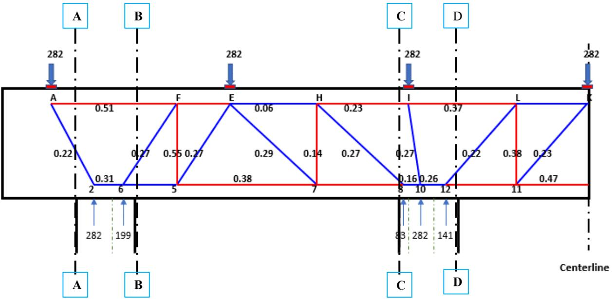
**Figure 7-13:** Utilization ratios calculated from STM-CAP for Bridge 3
