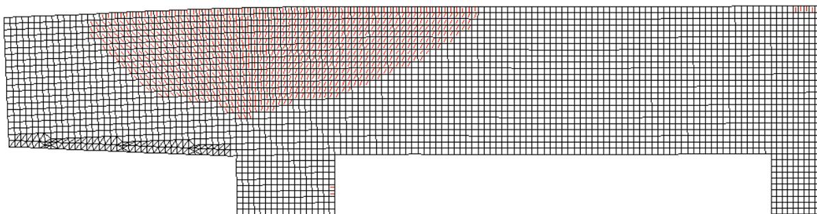
**Figure 6-16:** Cracking pattern at factored load for Bridge 1
