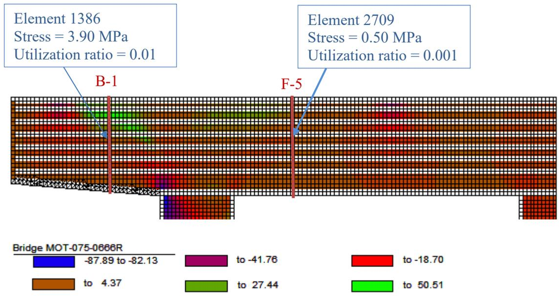
**Figure 6-13:** Smearing reinforcement stress at factored load for Bridge 1
