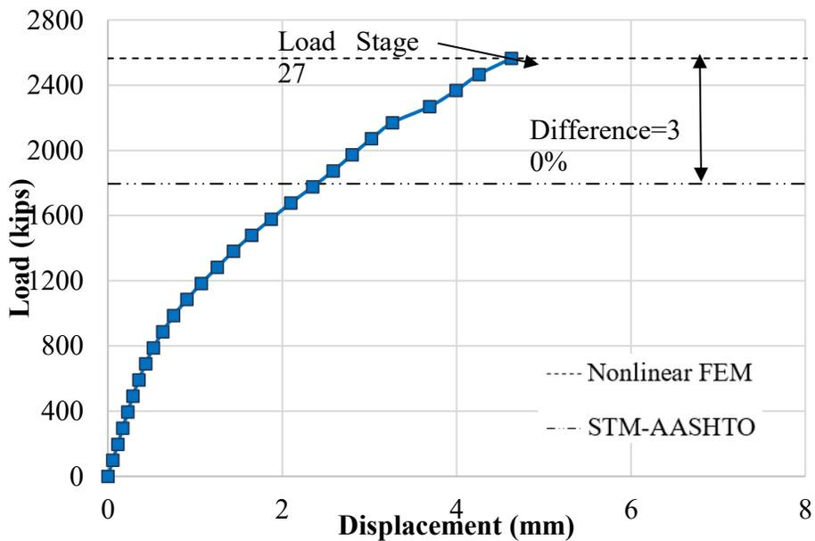
**Figure 6-45:** Load vs displacement response of cap beam for Bridge 3
