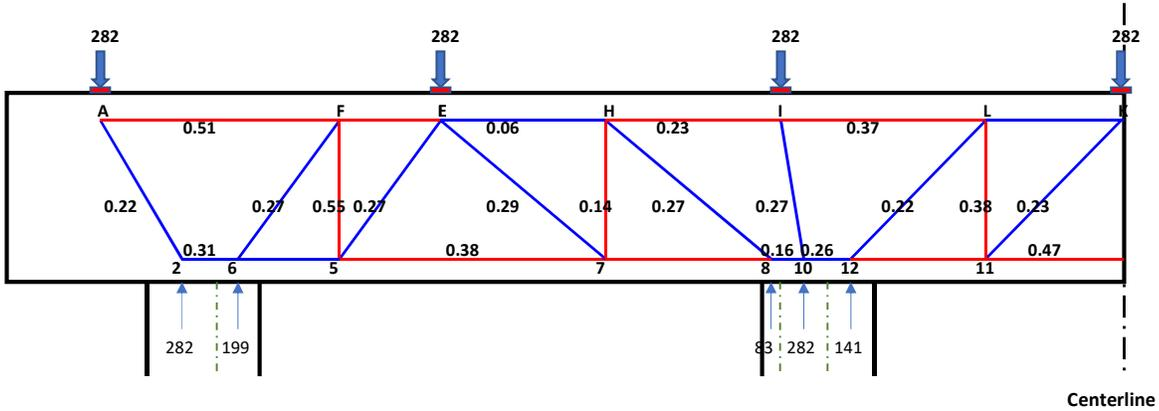
**Note:** The above figure shows the output model with Utilization Ratio along with the member which are color coded. The node numbers are also printed for every node. This output model is based on below calculation details.
