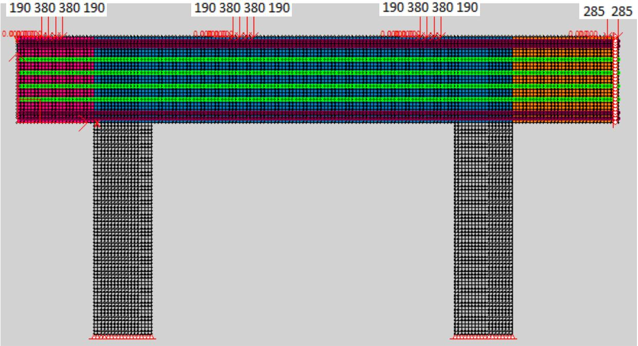
**Figure 6-48:** Cap beam model in VecTor2 for Bridge 4
