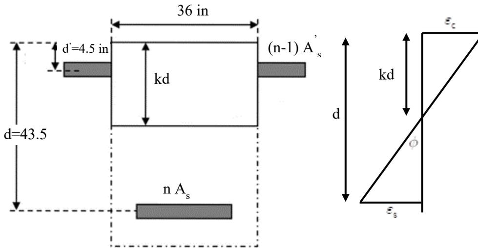
**Figure 7-5:** Strain distribution
