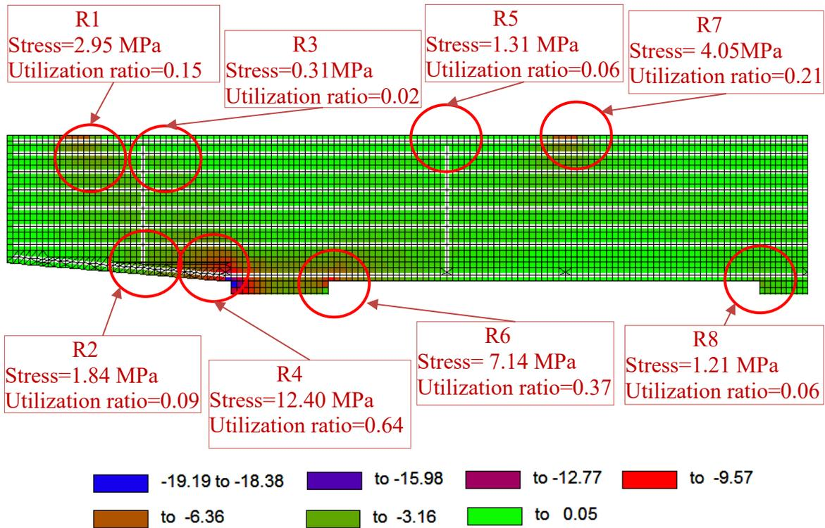
**Figure 6-20:** Concrete stress at factored load for Bridge 1
