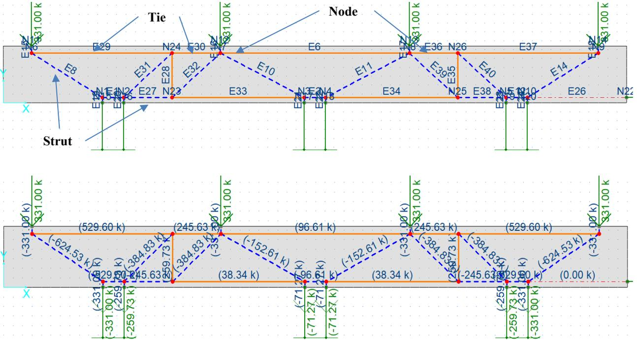
Figure 5-5: CAST model for strut-and-tie method for Bridge 1
