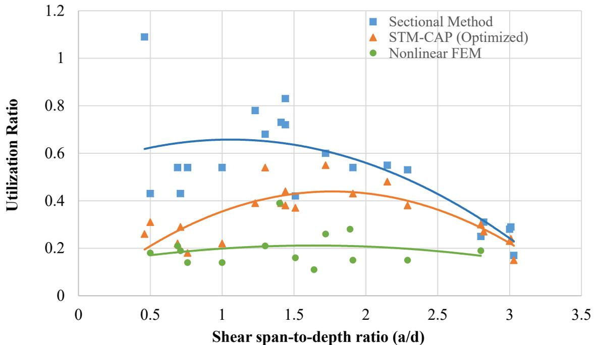
**Figure 7-20:** Comparison of results from analysis methods
