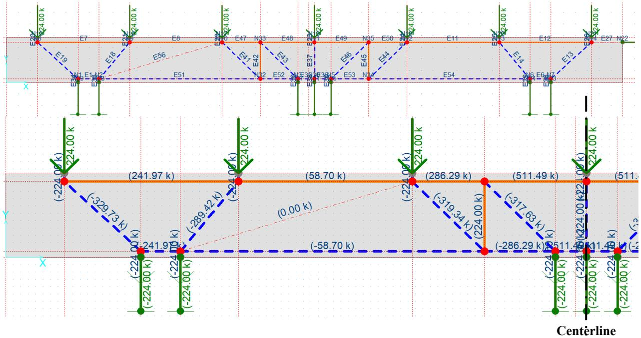
Figure 5-11: CAST model for the strut-and-tie method for Bridge 2
