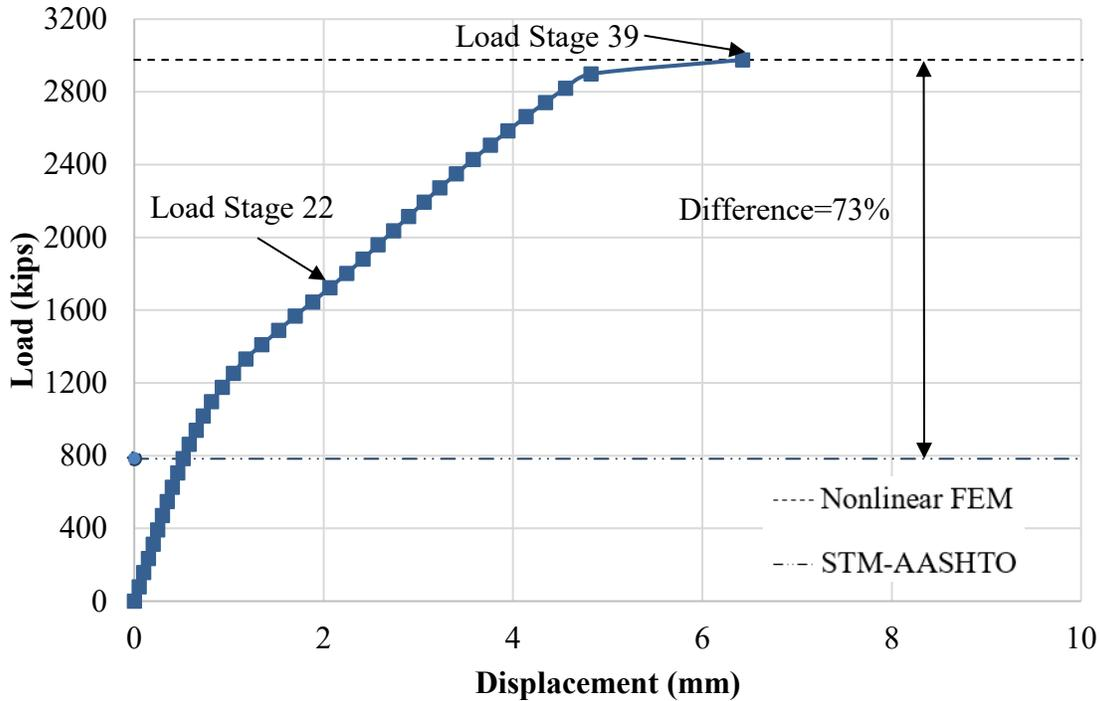
**Figure 6-36:** Load vs displacement response of cap beam for Bridge 2
