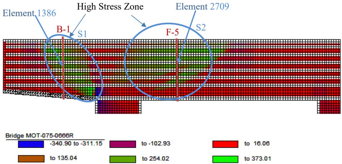
**Figure 6-12:** Smearing reinforcement stress at failure load for Bridge 1
