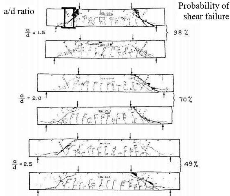
**Figure 2-1:** Probability of shear failure for corresponding  $a/d$  ratio (Kani, 1964)
