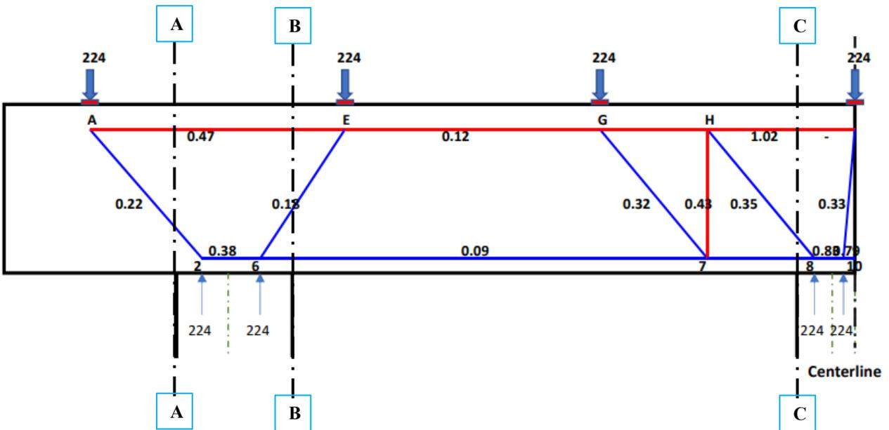
**Figure 7-10:** Utilization ratios calculated from STM-CAP for Bridge 2
