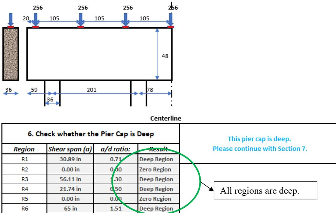
Figure 5-20: STM-CAP deep beam check (all units are in inches) for Bridge 4
