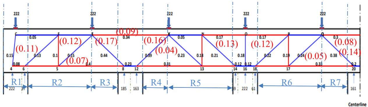
**Figure 6-60:** Utilization ratio from the STM-AASHTO and nonlinear FEM for Bridge 5
