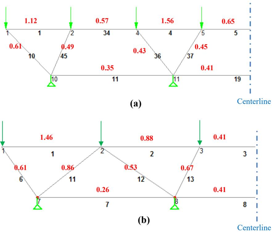
**Figure 9-2:** Utilization ratios for sample (a) Pier Cap 1; (b) Pier Cap 2
