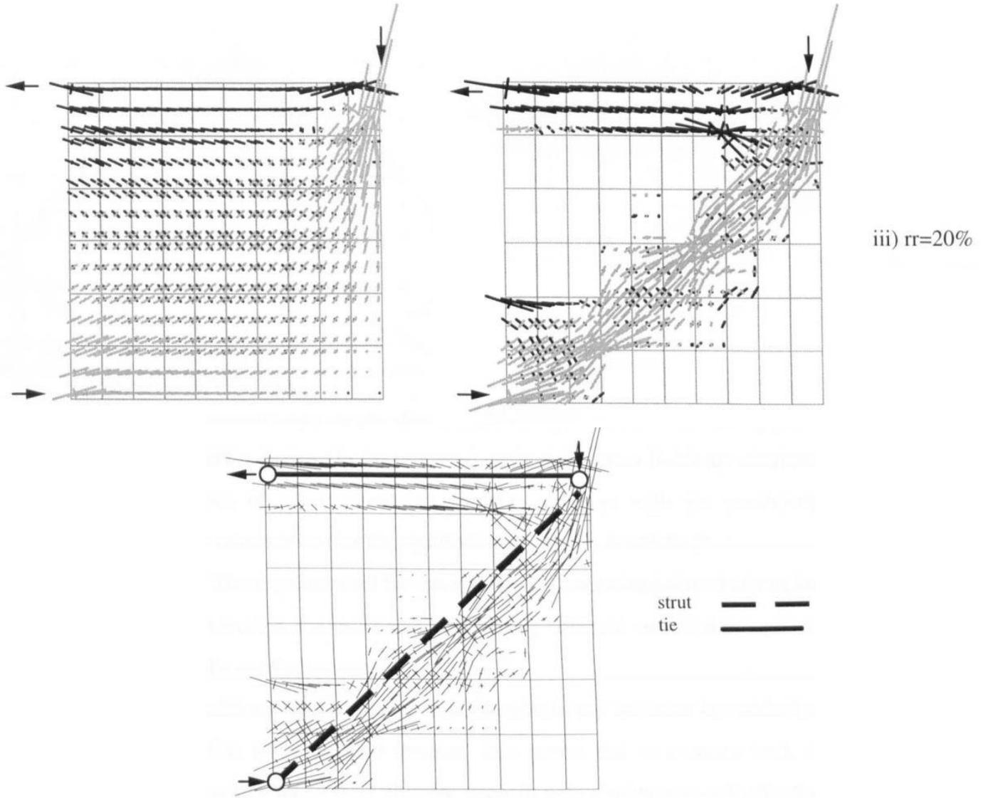
**Figure 2-7:** Deep cantilever beam of  $a/d$  ratio = 1.00 visualizing STM model
