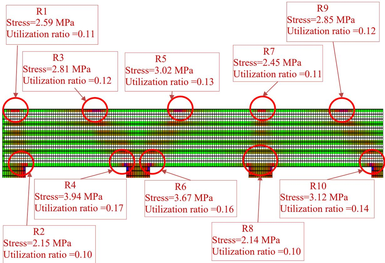
**Figure 6-58:** Concrete stress and utilization ratio at factored load for Bridge 5
