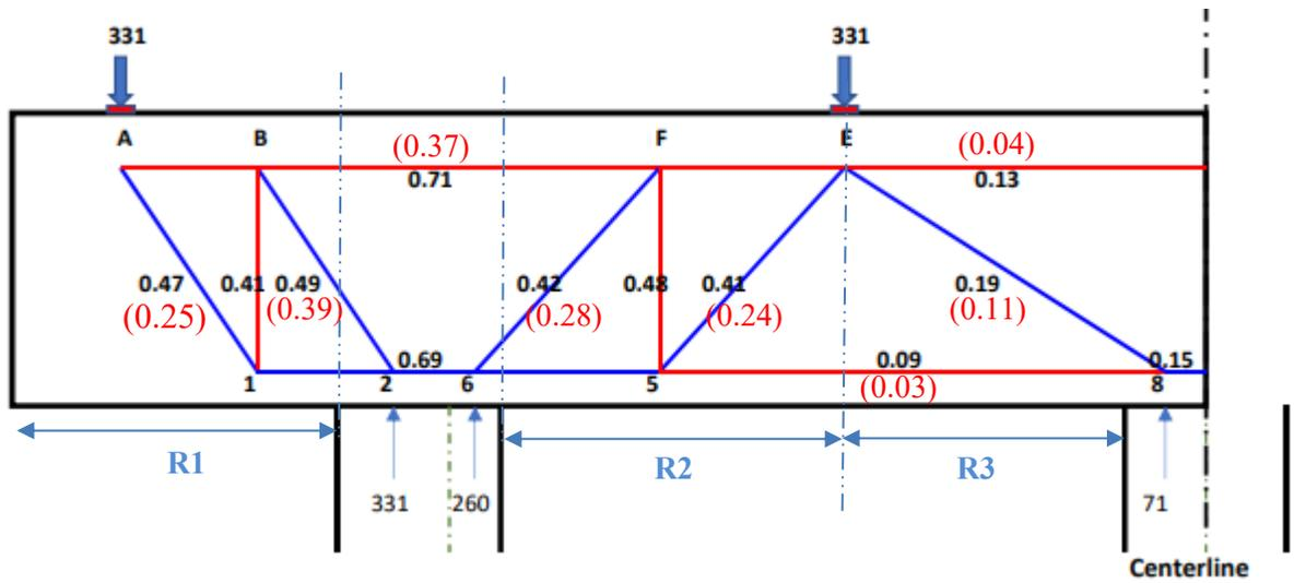
**Figure 6-14:** Utilization ratio from STM-AASHTO and nonlinear FEM for Bridge 1
