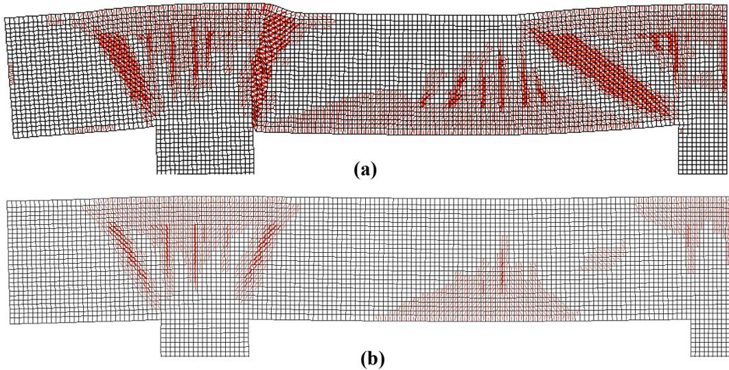
**Figure 6-34:** Cracking pattern (a) at failure load (b) when rebar yields first for Bridge 2
