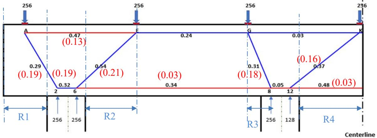
**Figure 6-51:** Utilization ratio from the STM-AASHTO and nonlinear FEM for Bridge 4
