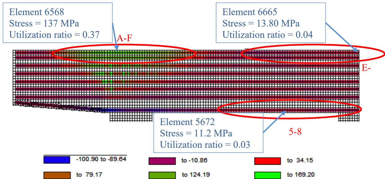
**Figure 6-11:** Average Reinforcement stresses at factored load for Bridge 1
