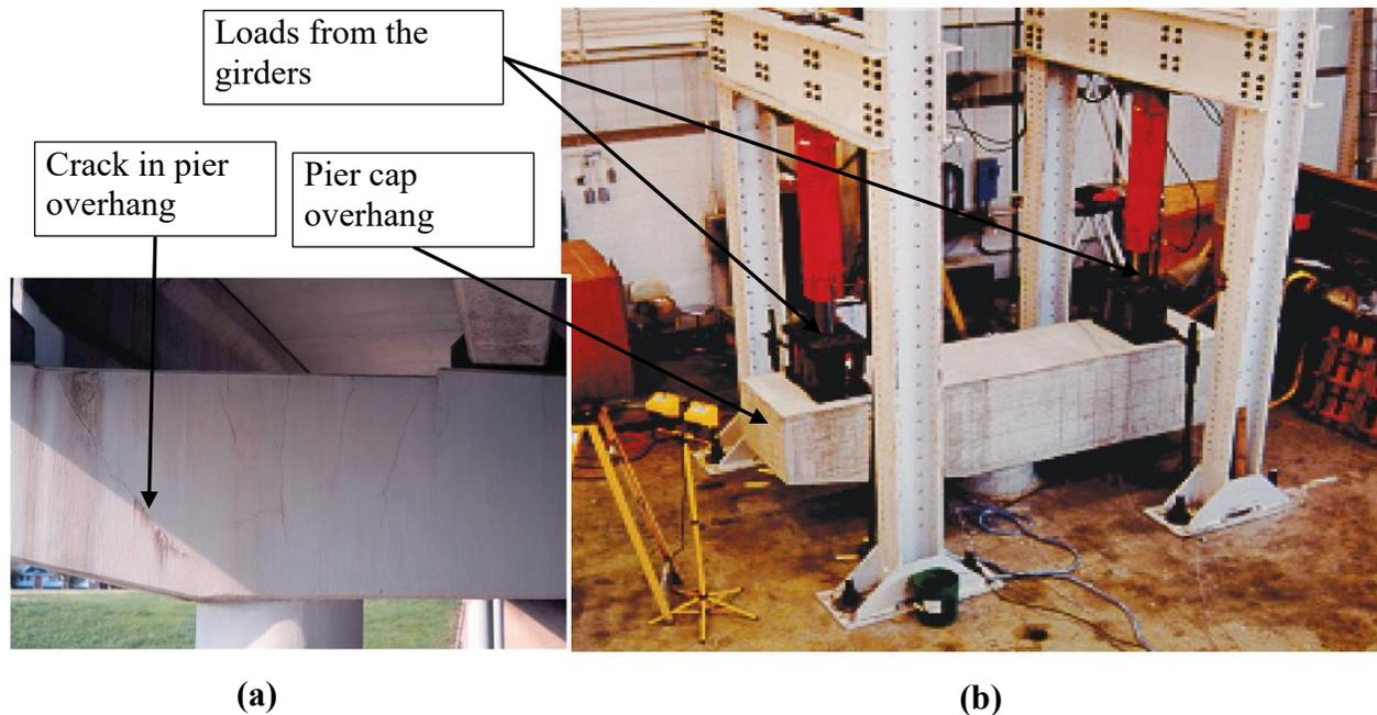
**Figure 2-4:** (a) Crack in pier cap; (b) experimental setup (Young et al., 2000 and 2002)
