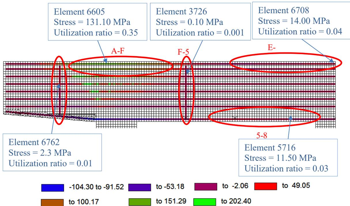
**Figure 6-22:** Average reinforcement stresses at factored load for Bridge 1
