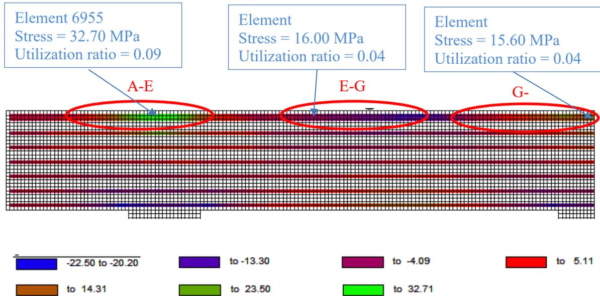
**Figure 6-31:** Average reinforcement stresses and utilization ratio at factored load, Bridge 2
