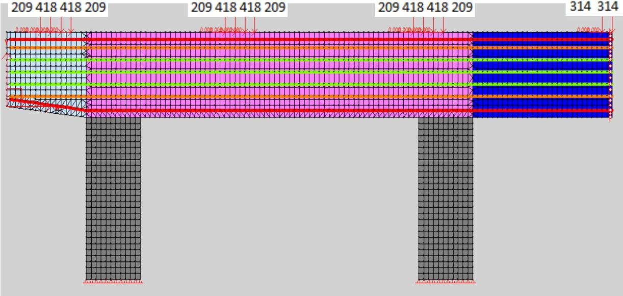
**Figure 6-39:** Cap beam model in VecTor2 for Bridge 3
