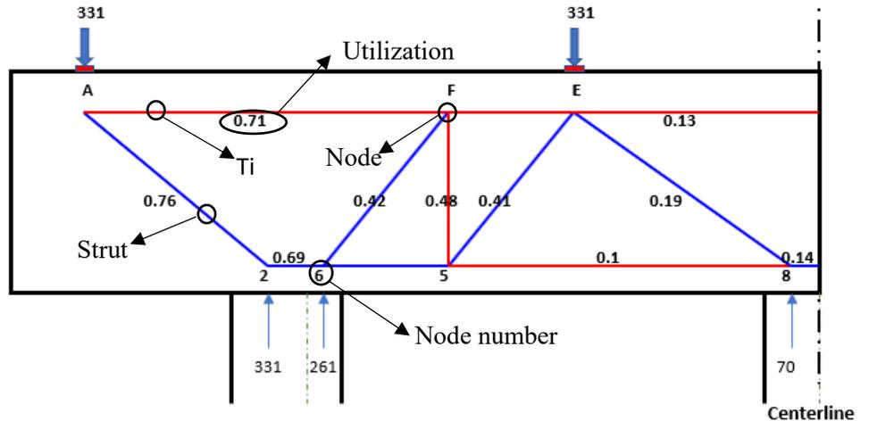
**Figure 4-22:** Sample output model with utilization ratios
