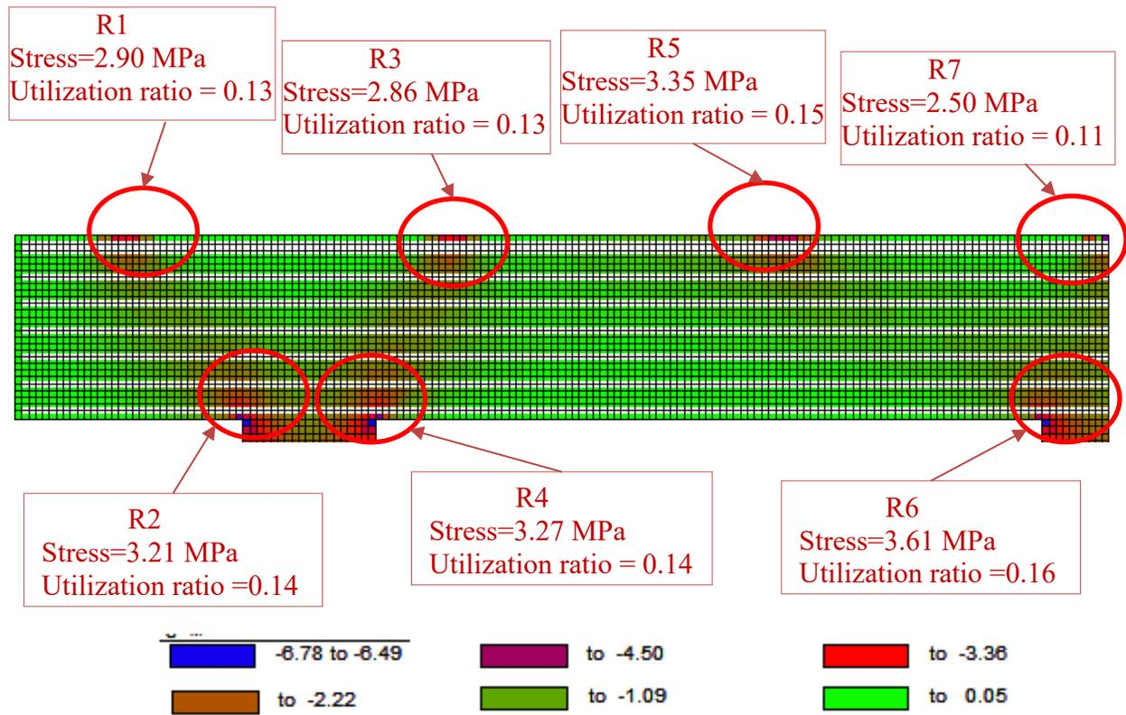
**Figure 6-30:** Concrete stress and utilization ratio at factored load for Bridge 2
