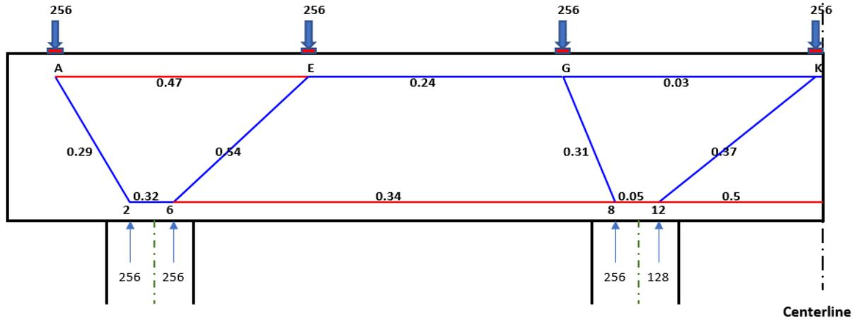
Figure 5-21: STM-CAP output model with utilization ratios for Bridge 4
