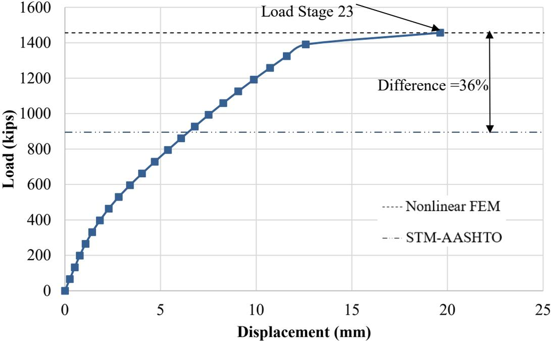
**Figure 6-17:** Load vs displacement response of cap beam for Bridge 1
