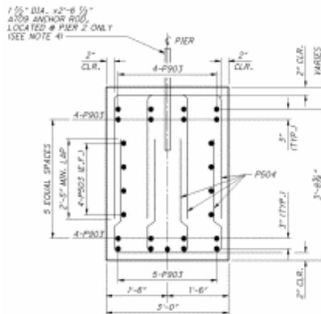
**Figure 6-47:** Section of the beam for Bridge 4
