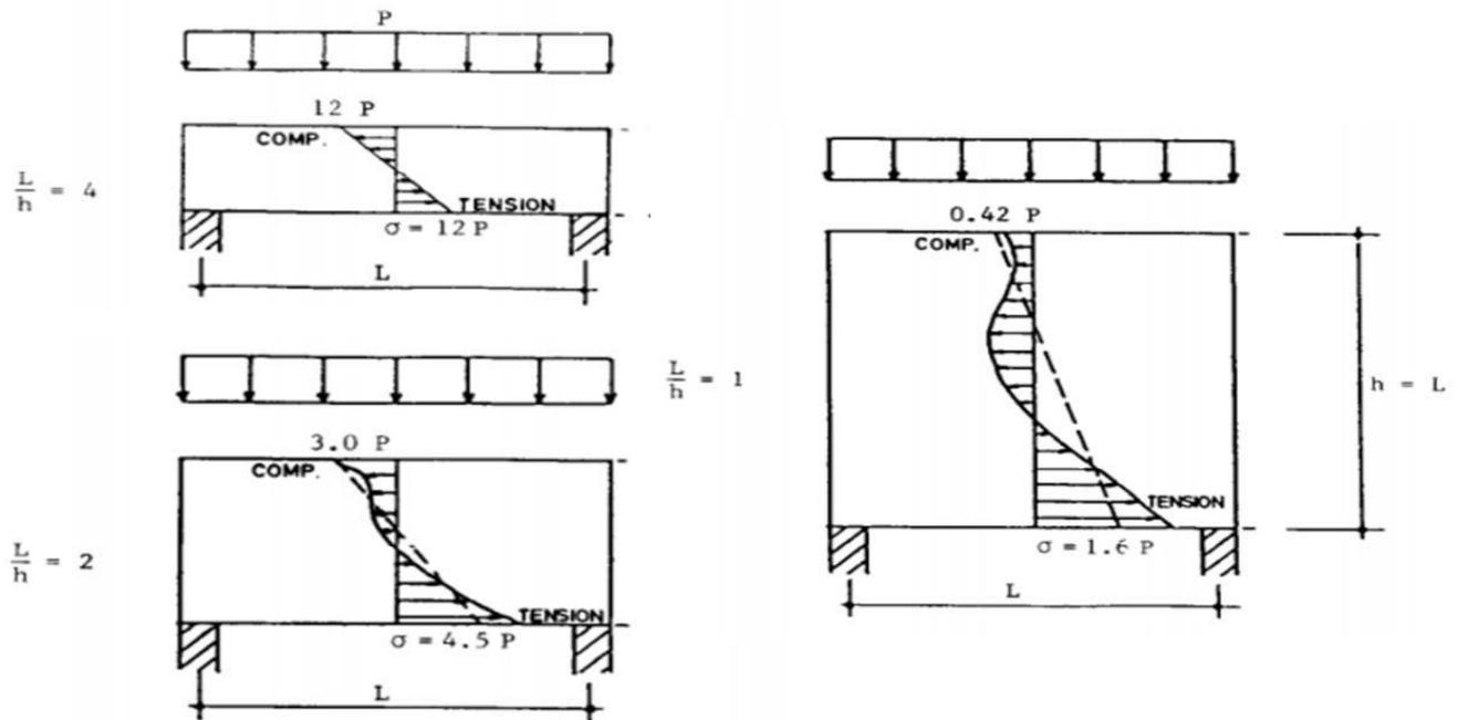
**Figure 2-8:** Nonlinear strain distribution for different  $a/d$  ratio (Lafta et al., 2016)
