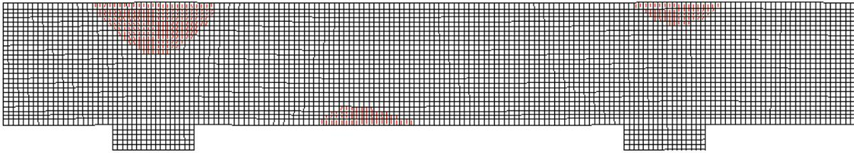
**Figure 6-53:** Cracking pattern at factored load for Bridge 4
