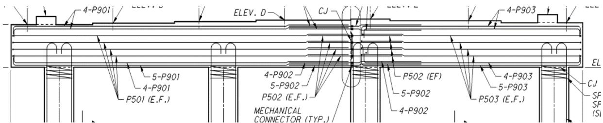
**Figure 6-46:** Pier cap details for Bridge 4
