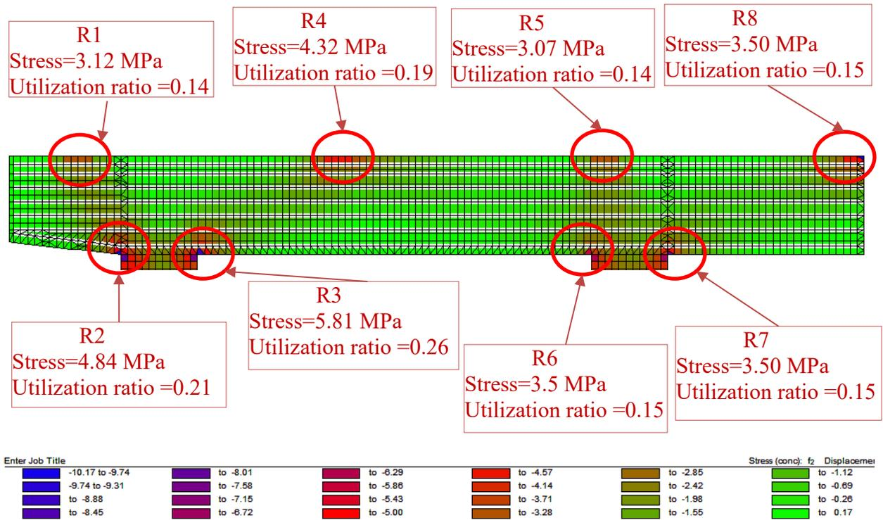
**Figure 6-40:** Concrete stresses and utilization ratio at factored load for Bridge 3
