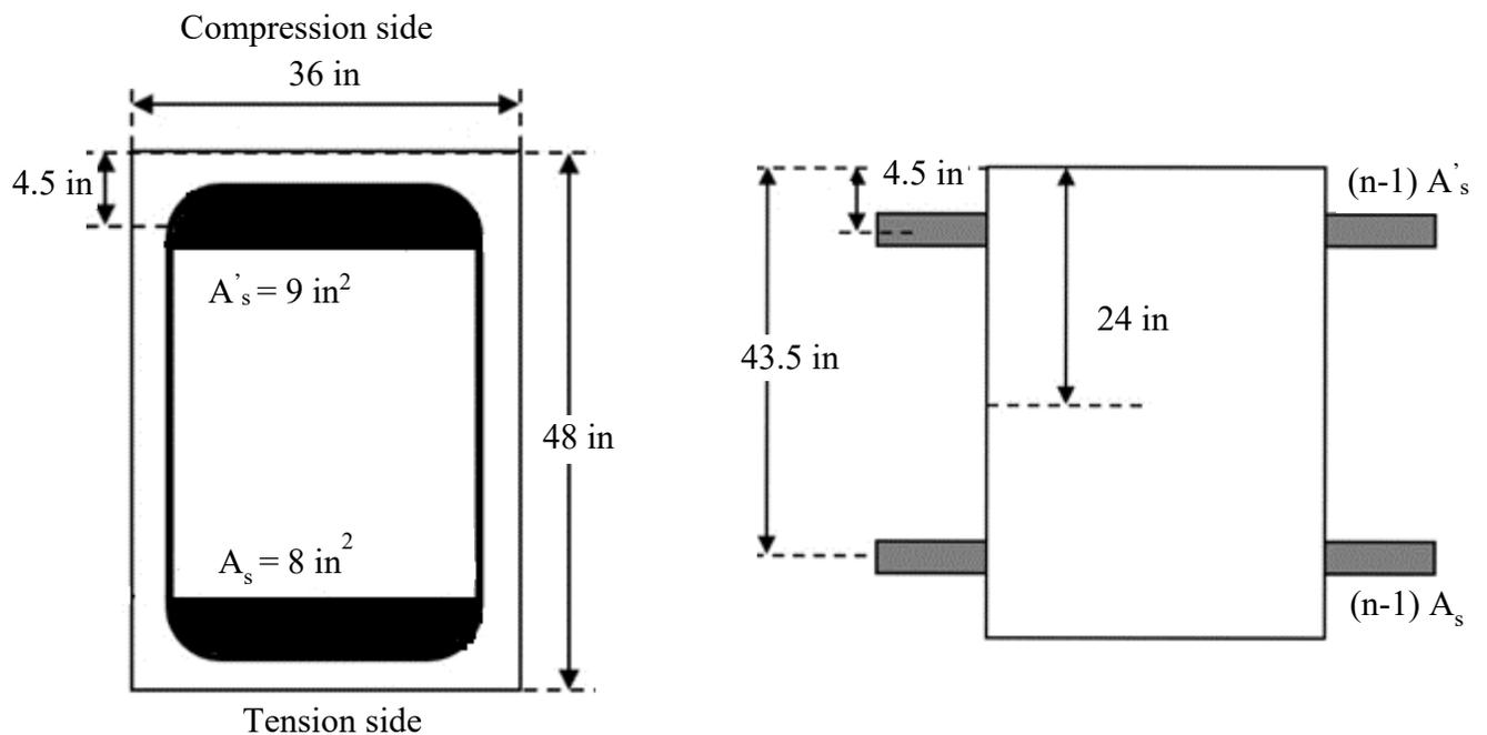
**Figure 7-3:** Section details and un-cracked transformed section properties
