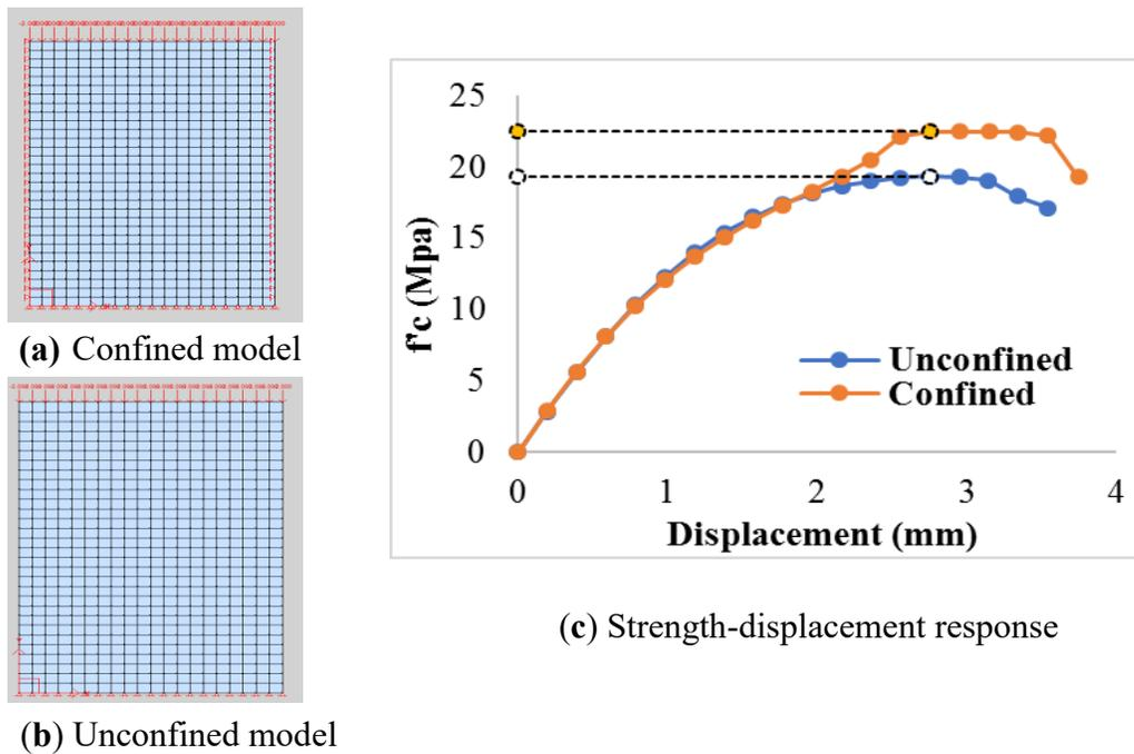
**Figure 6-7:** Confined compressive strength of concrete for Bridge 1
