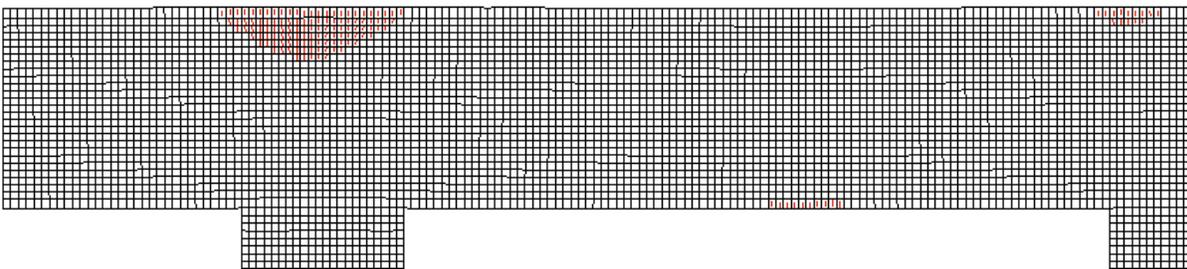
**Figure 6-35:** Cracking pattern at factored load for Bridge 2
