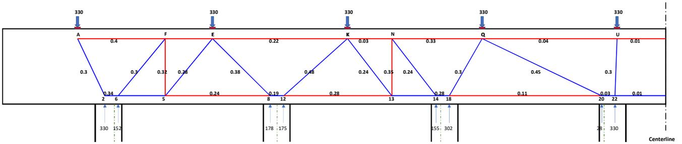
**Note:** The above figure shows the output model with Utilization Ratio along with the member which are color coded. The node numbers are also printed for every node. This output model is based on below calculation details.
