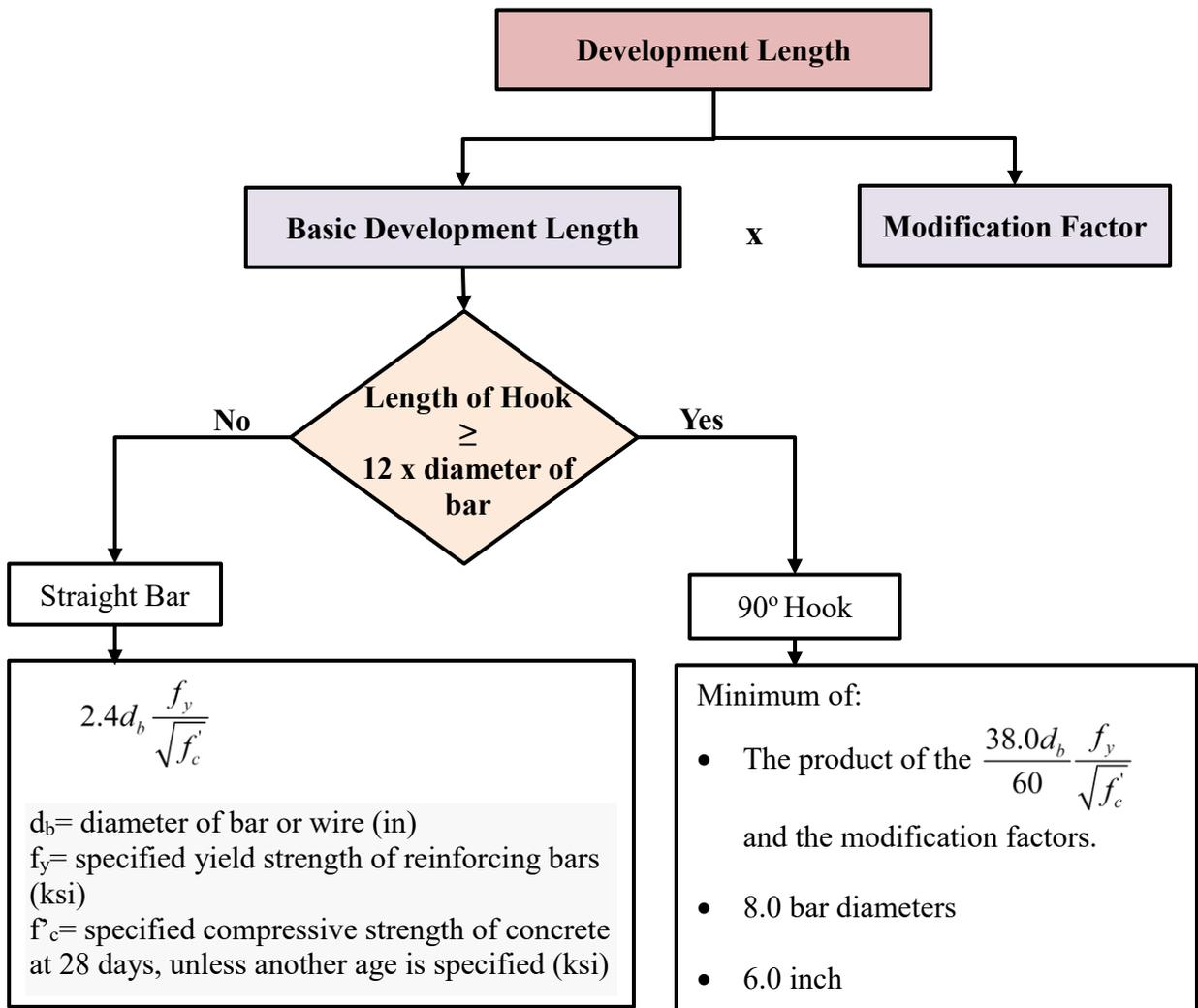
**Figure 4-19:** Flowchart for reinforcement development (AASHTO, 2017)
