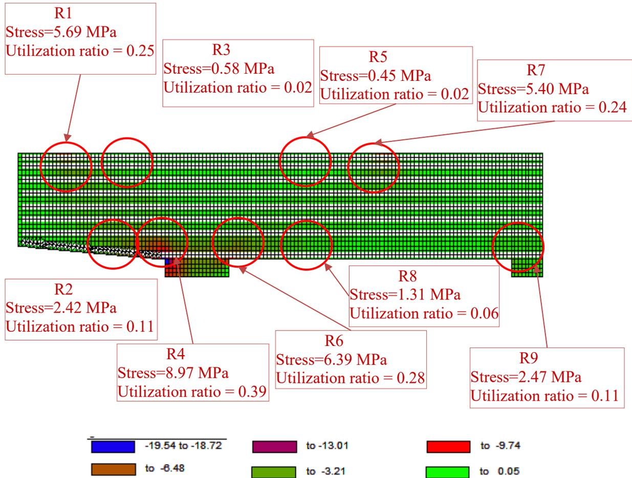
**Figure 6-9:** Concrete stress at factored load for Bridge 1
