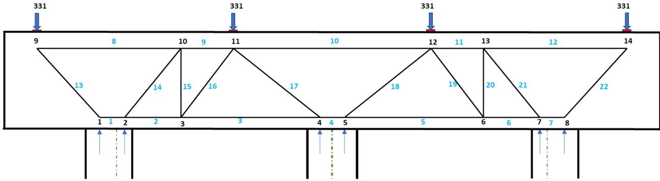
**Figure 4-26:** Assumed labeling for matrix stiffness method
