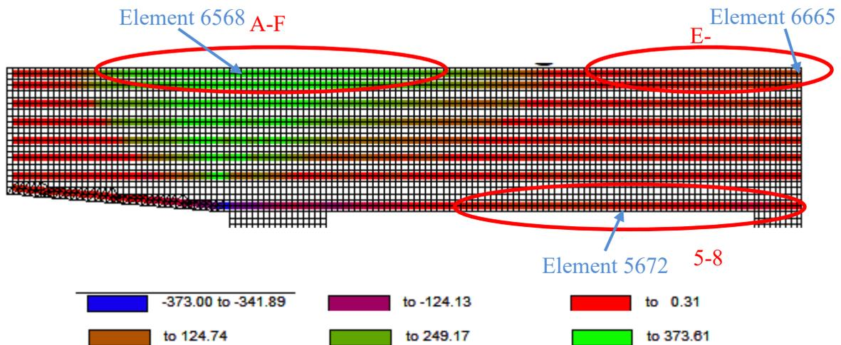
**Figure 6-10:** Average Reinforcement stresses at failure load for Bridge 1
