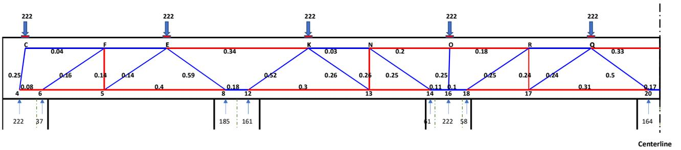
**Note:** The above figure shows the output model with Utilization Ratio along with the member which are color coded. The node numbers are also printed for every node. This output model is based on below calculation details.
