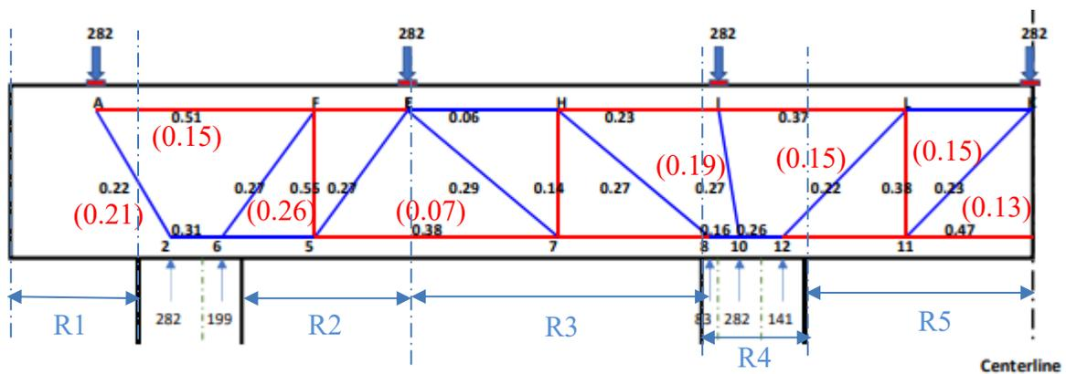
**Figure 6-42:** Utilization ratio from the STM-AASHTO and nonlinear FEM for Bridge 3
