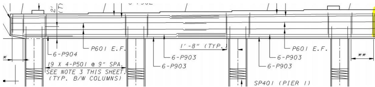
**Figure 5-37:** Pier cap elevation for Bridge 7
