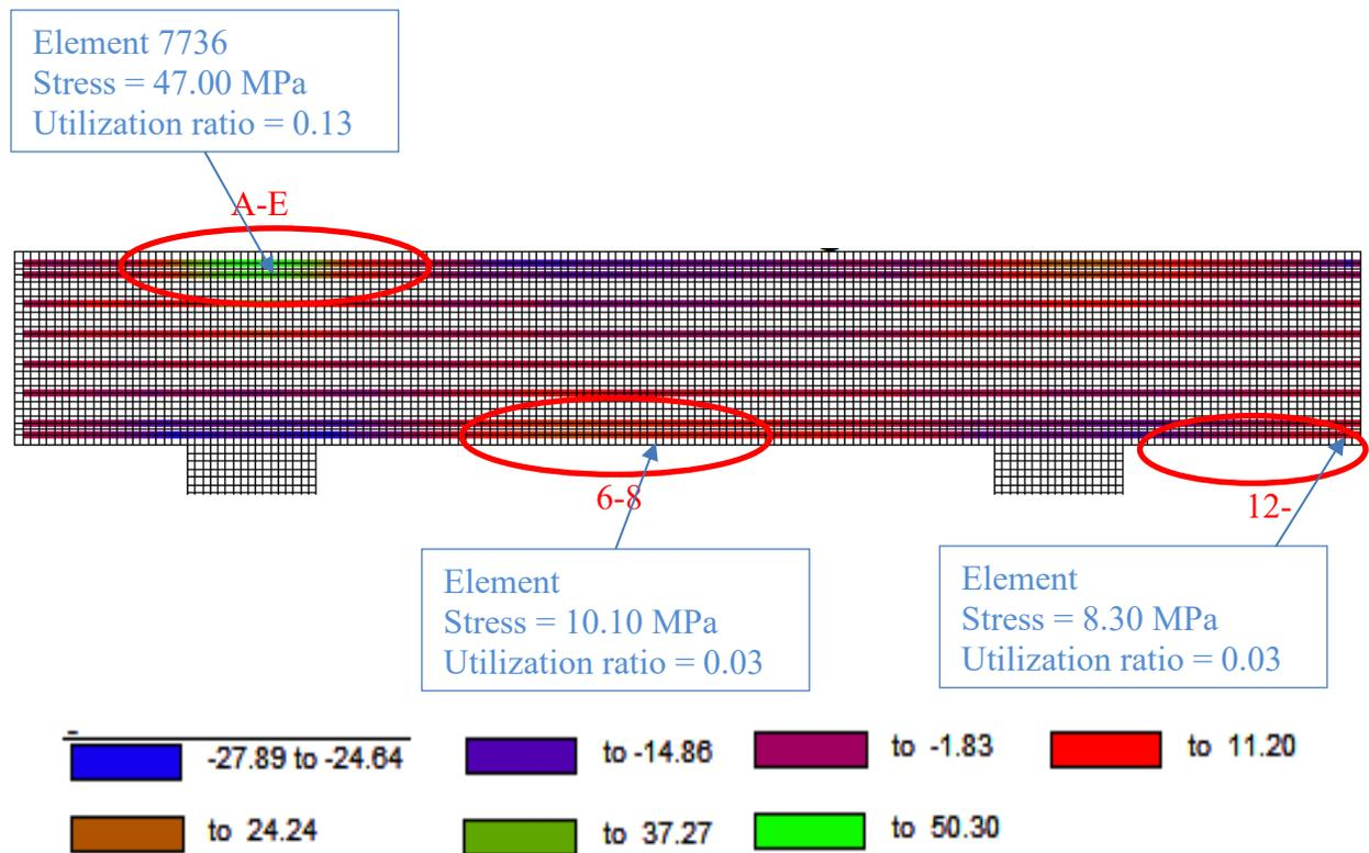
Figure 6-50: Average reinforcement stresses and utilization ratio at factored load, Bridge 4
