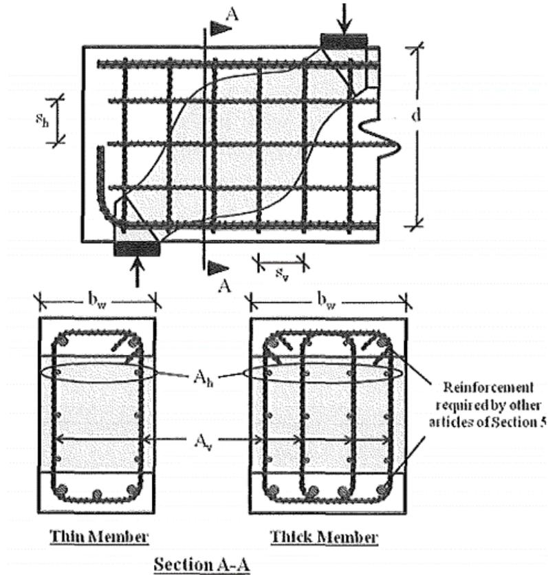
**Figure 3-7:** Distribution of crack control reinforcement (AASHTO Figure C5.6.3.6-1)
