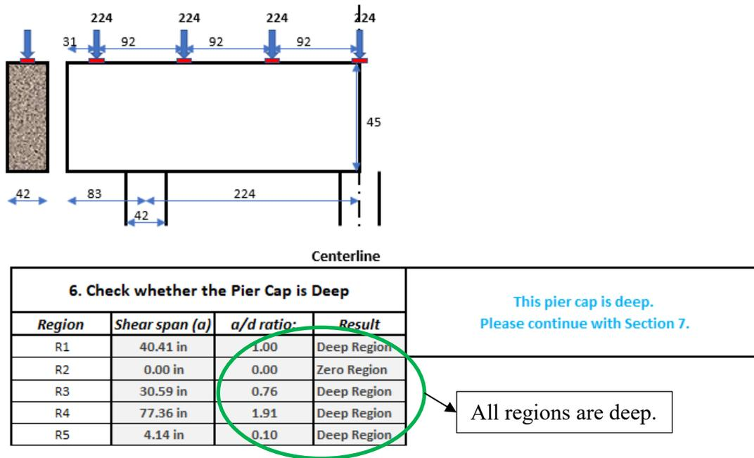
Figure 5-8: STM-CAP deep beam check (all units are in inches) for Bridge 2
