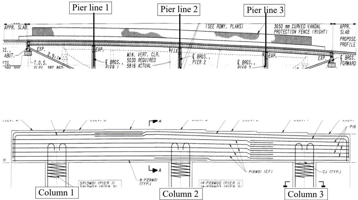
Figure 6-27: Pier cap details for Bridge 2
