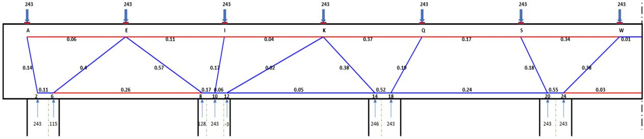
Figure 5-33: STM-CAP output model with utilization ratios for Bridge 6
