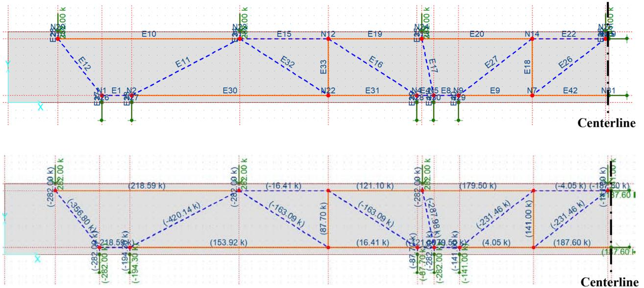
**Figure 5-17:** CAST model for the strut-and-tie method for Bridge 3
