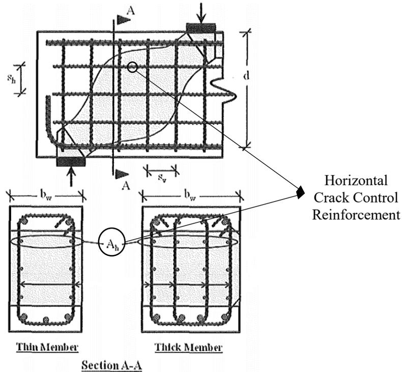
Figure C5.6.3.6-1—Distribution of Crack Control Reinforcement in Compression Strut
