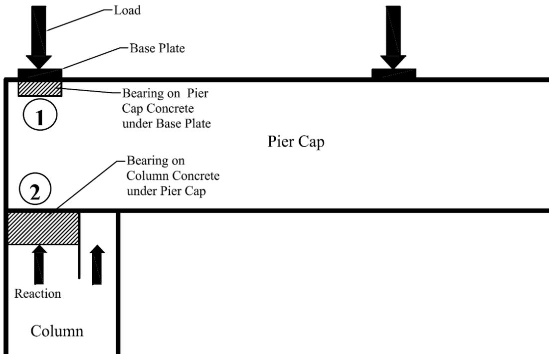
**Figure 4-25:** Bearing check concrete areas
