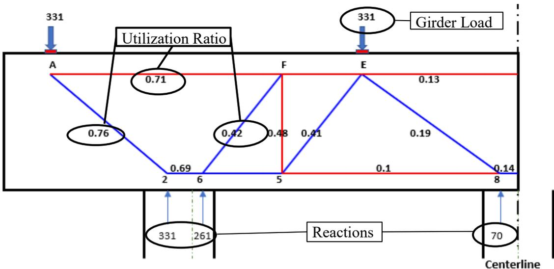
**Figure 5-3:** STM-CAP output model with utilization ratios for Bridge 1
