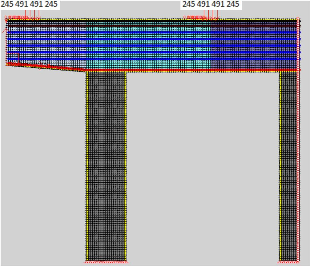
**Figure 6-5:** Cap beam model in VecTor2 for Bridge 1
