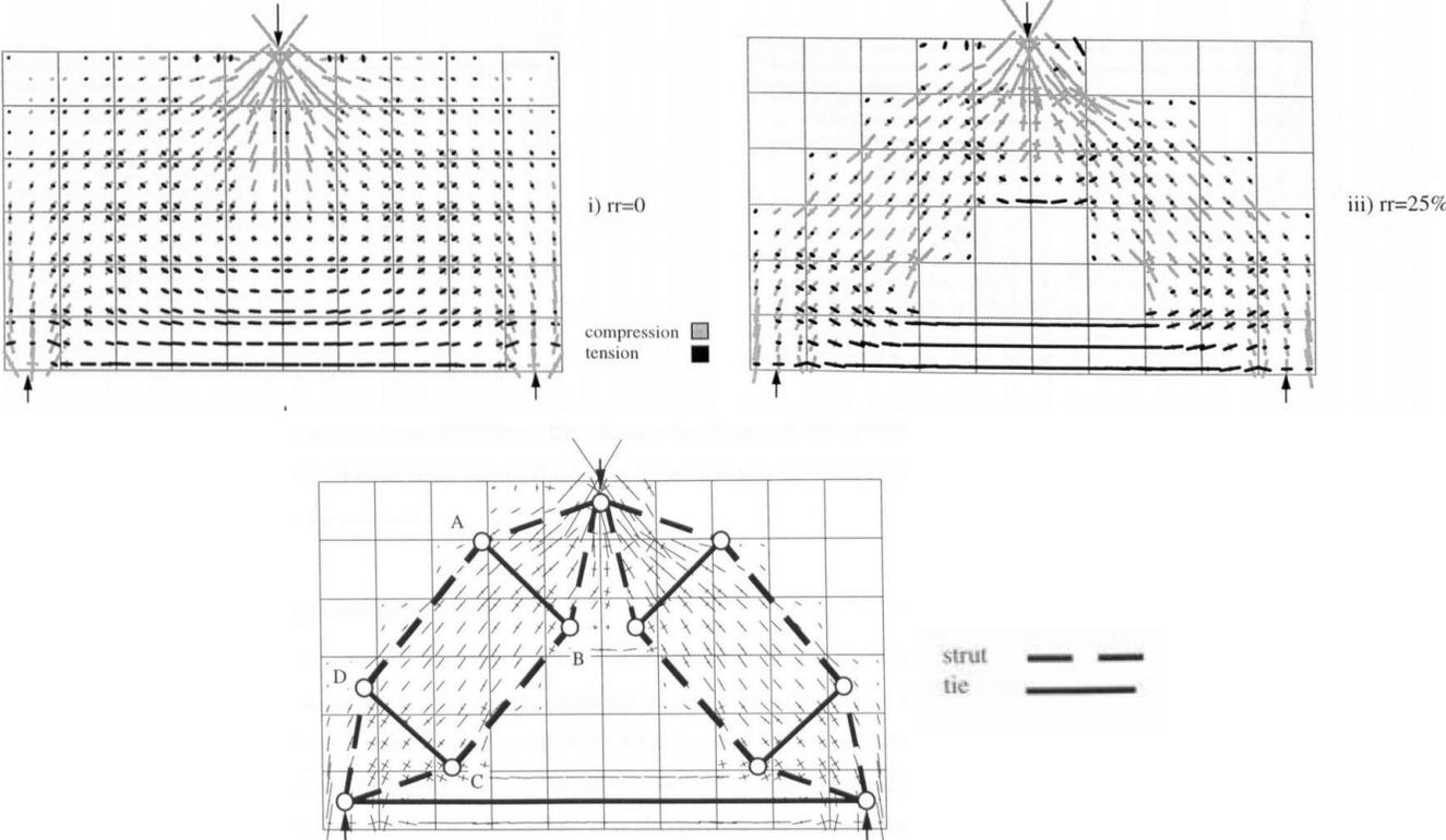
**Figure 2-6:** Deep simply supported beam of  $a/d=1.67$  visualizing STM model
