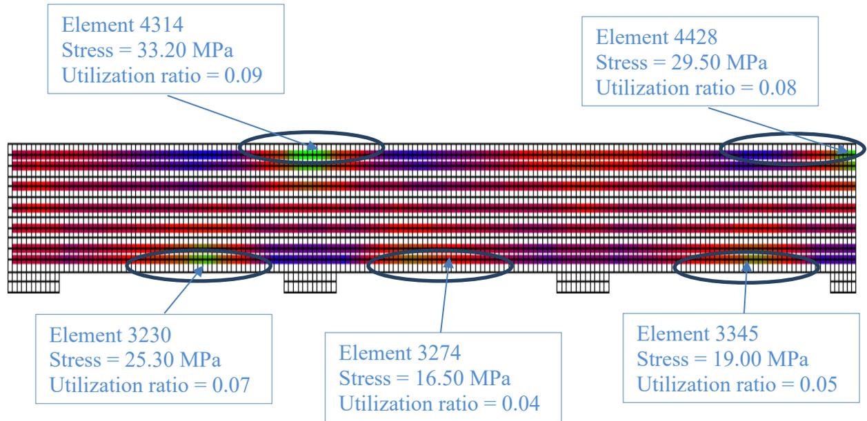
**Figure 6-59:** Average reinforcement stresses and utilization ratio at factored load, Bridge 5
