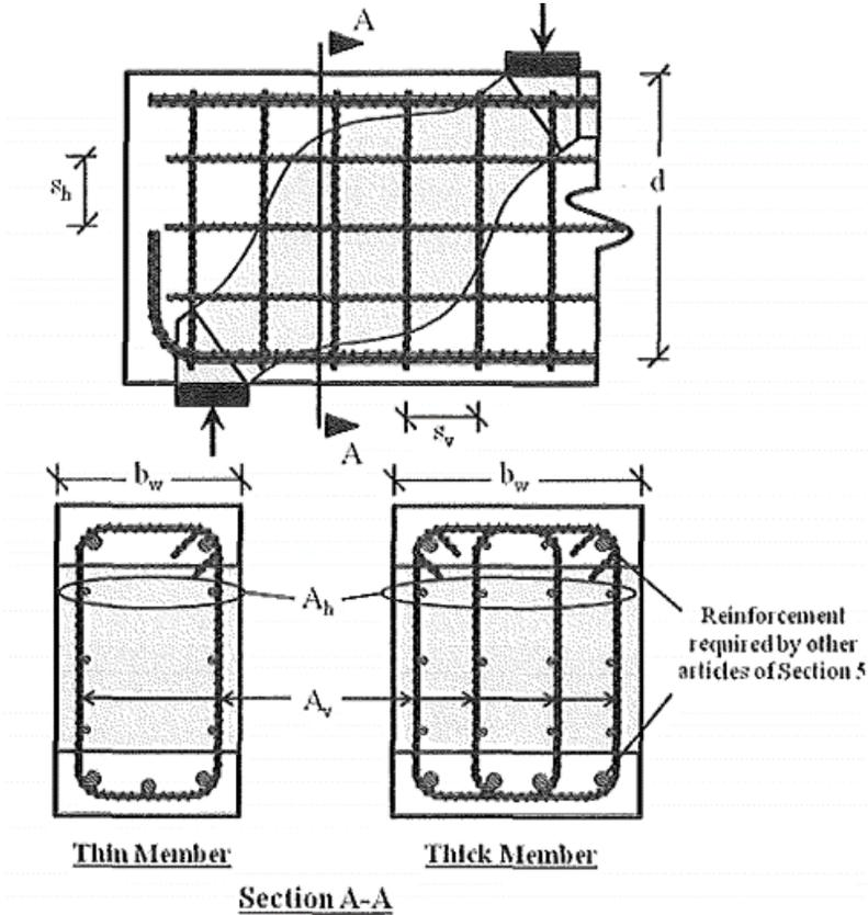
**Figure 8-3:** Distribution of crack control reinforcement (AASHTO Figure C5.8.2.6-1)
