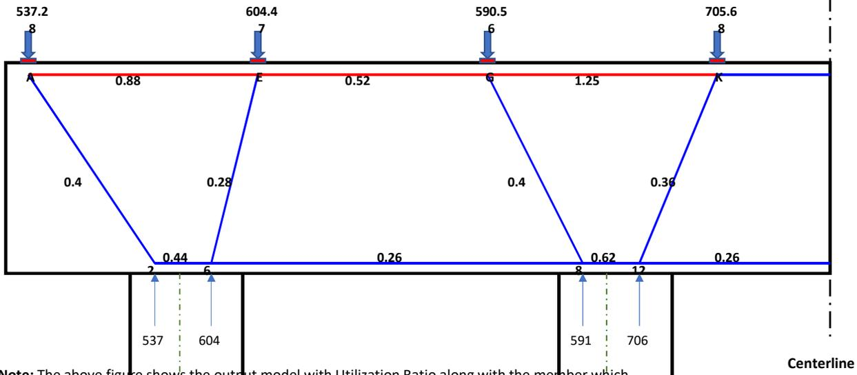
**Note:** The above figure shows the output model with Utilization Ratio along with the member which are color coded. The node numbers are also printed for every node. This output model is based on below calculation details.
