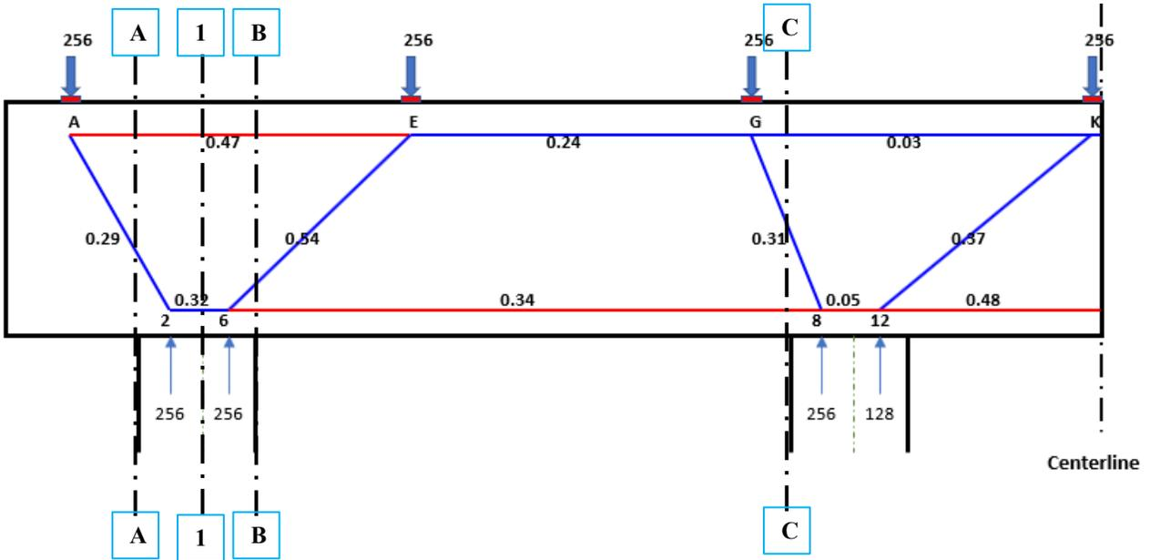
**Figure 7-7:** Utilization ratios calculated from STM-CAP for Bridge 1
