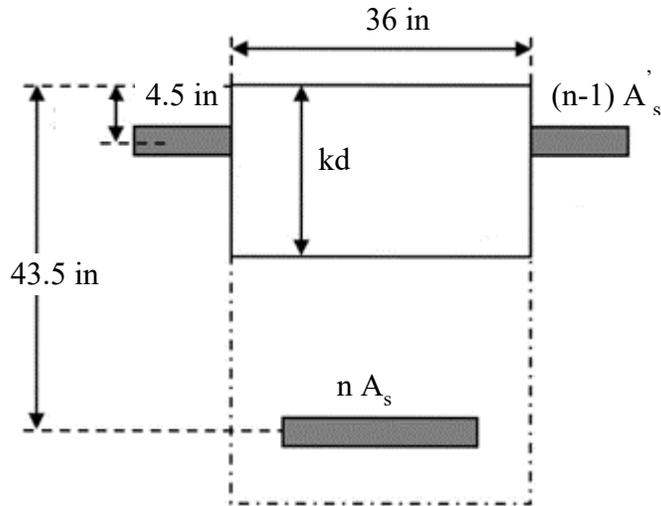
**Figure 7-4:** Cracked, transformed section properties
