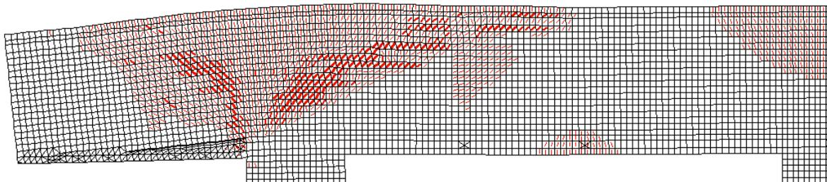
**Figure 6-24:** Cracking pattern at failure load for Bridge 1
