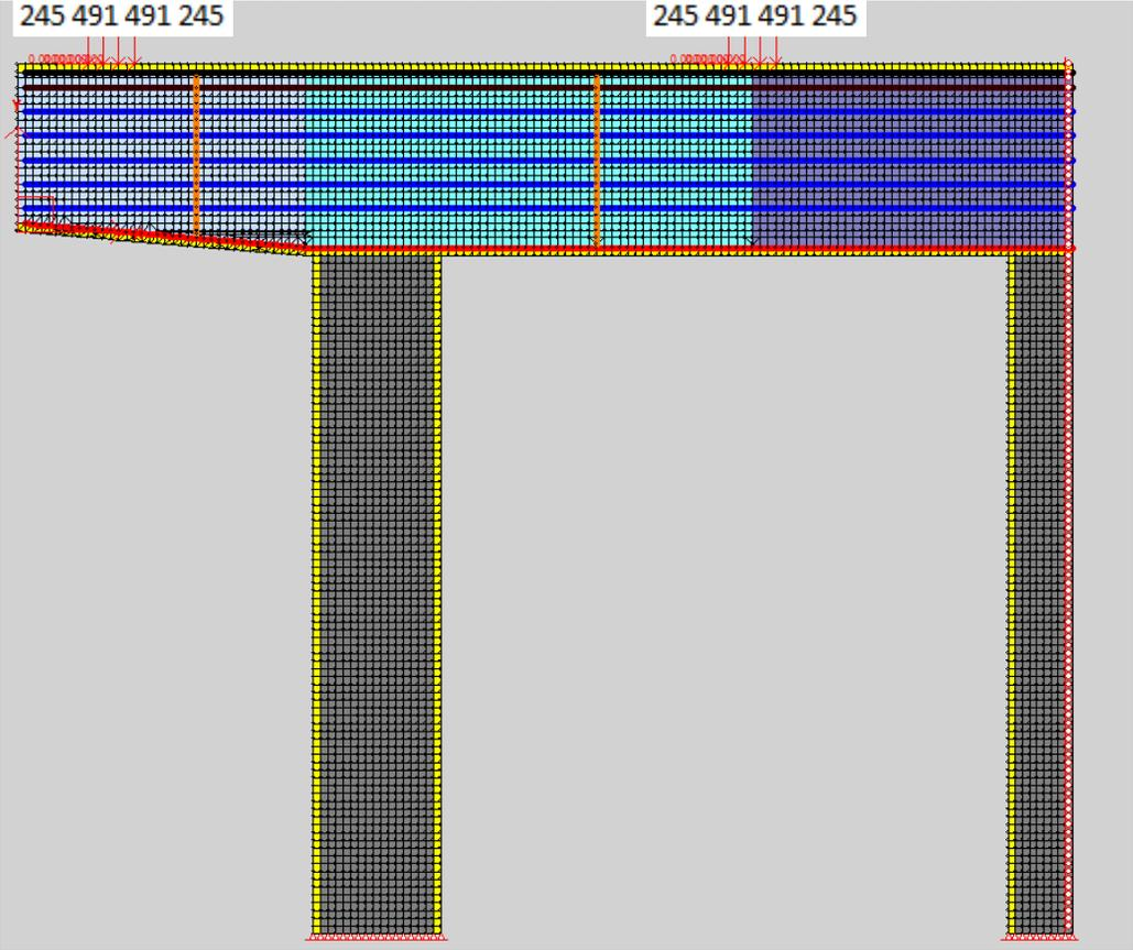
**Figure 6-18:** Cap beam model in VecTor2 for Bridge 1
