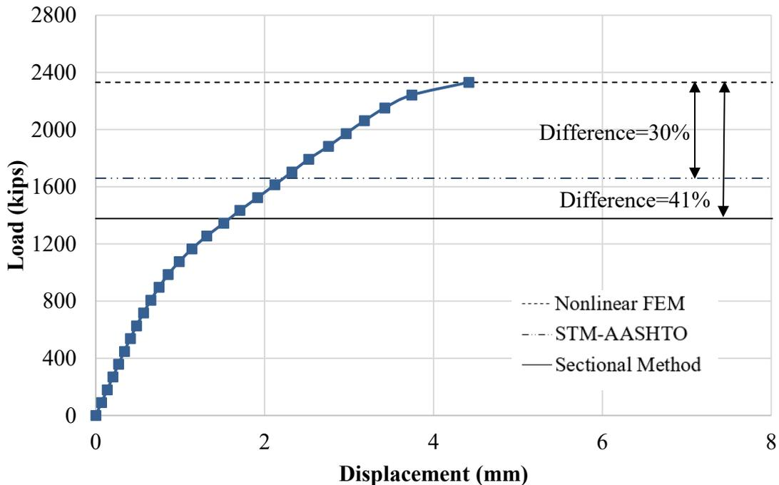
**Figure 6-54:** Load vs displacement response of cap beam for Bridge 4
