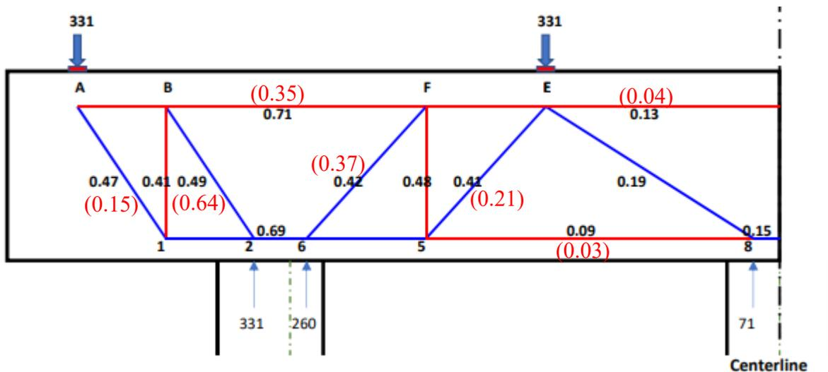
**Figure 6-23:** Utilization ratio from the STM-AASHTO and nonlinear FEM for Bridge 1
