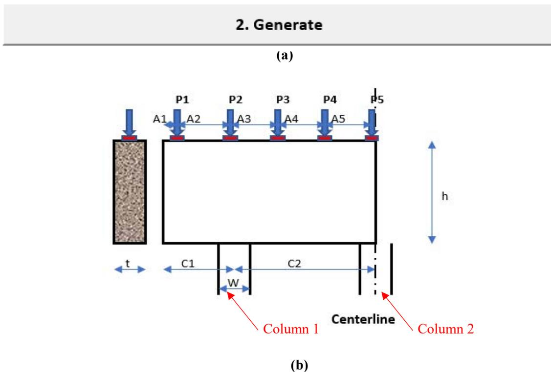
**Figure 4-5:** (a) '2. Generate' button; (b) automated drawing showing the input variables
