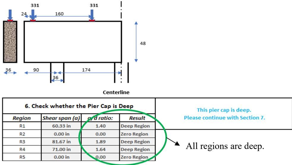
**Figure 5-2:** STM-CAP deep beam check (all units are in inches) for Bridge 1
