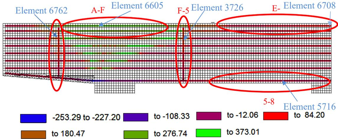
**Figure 6-21:** Average Reinforcement stresses at failure load for Bridge 1
