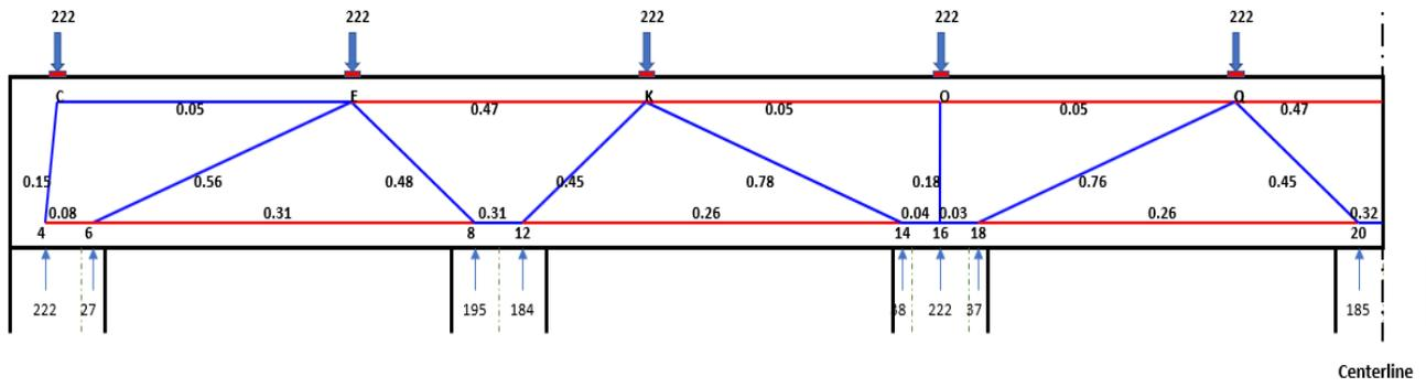
Figure 5-27: STM-CAP output model with utilization ratios for Bridge 5
