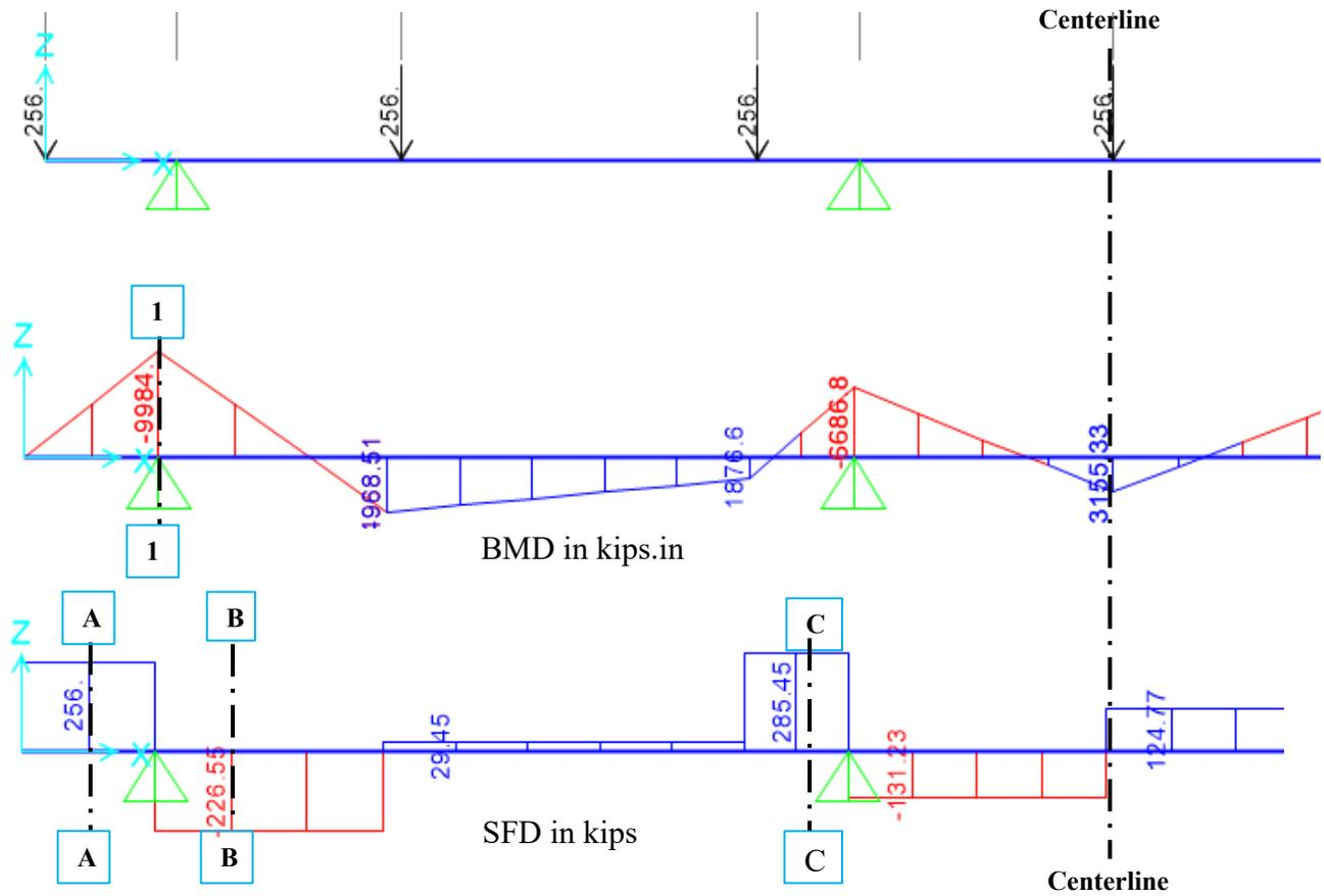
**Figure 7-2:** Bridge 1 pier cap BMD and SFD using SAP2000
