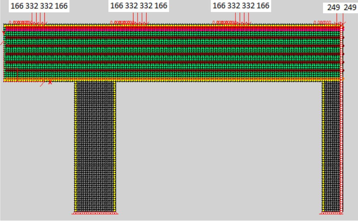
Figure 6-29: Cap beam model in VecTor2 for Bridge 2
