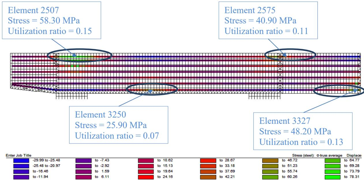
**Figure 6-41:** Average reinforcement stresses and utilization ratio at factored load, Bridge 3
