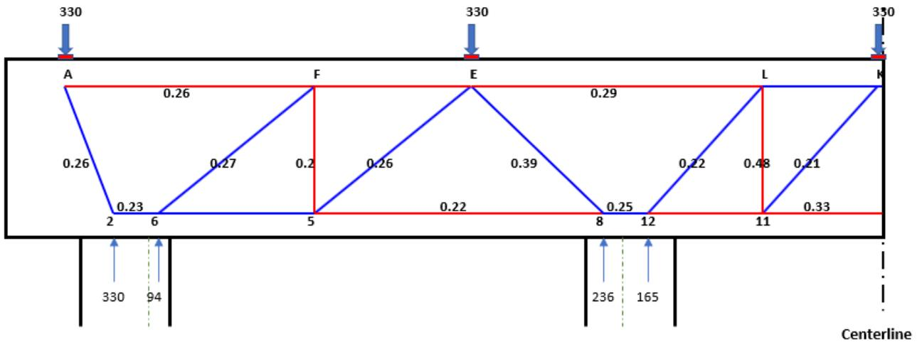
Figure 5-39: STM-CAP output model with utilization ratios for Bridge 7
