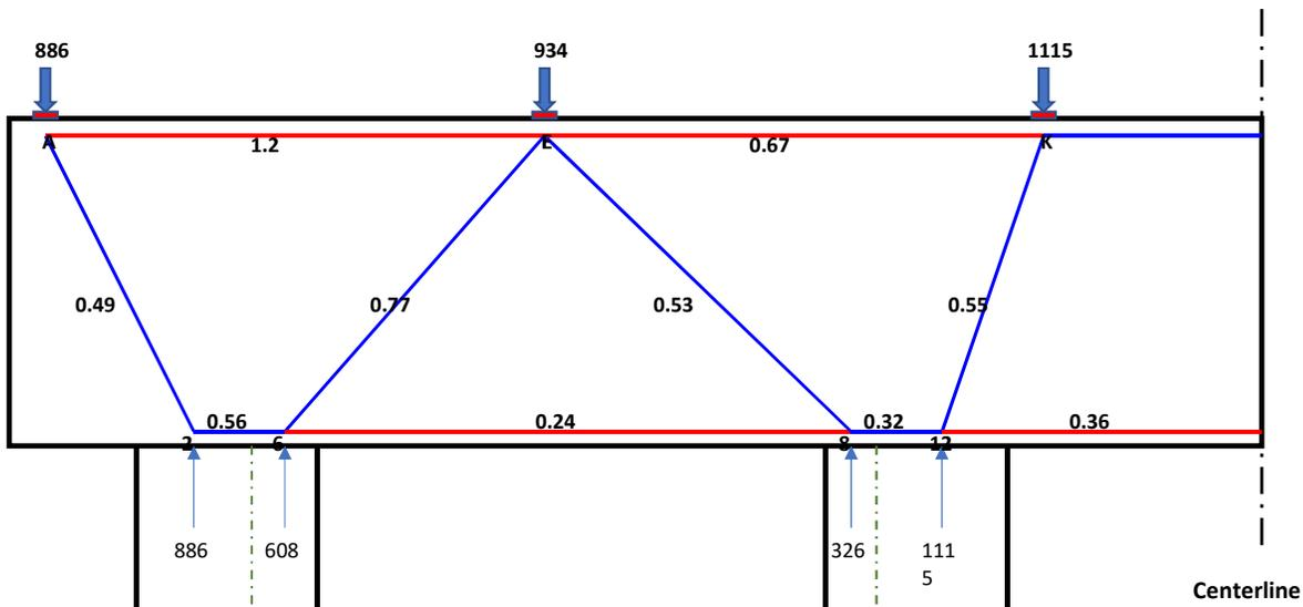
**Note:** The above figure shows the output model with Utilization Ratio along with the member which are color coded. The node numbers are also printed for every node. This output model is based on below calculation details.
