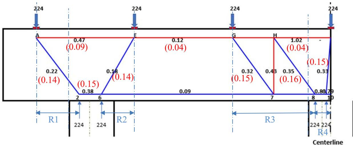
**Figure 6-33:** Utilization ratio from the STM-AASHTO and nonlinear FEM for Bridge 2
