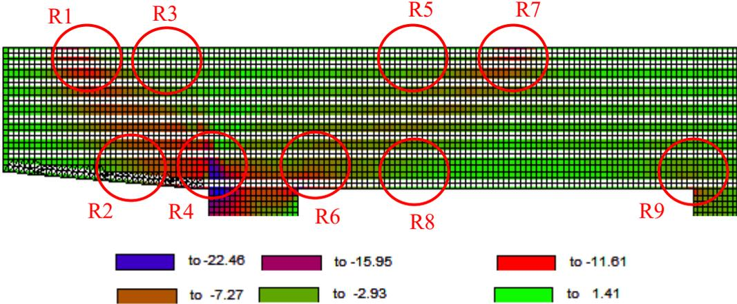
**Figure 6-8:** Concrete stress at failure for Bridge 1
