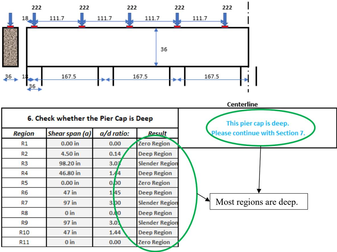
Figure 5-26: STM-CAP deep beam check (all units are in inches) for Bridge 5
