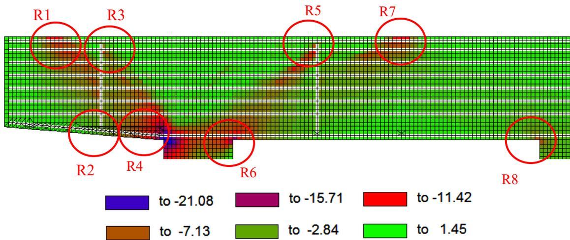
**Figure 6-19:** Concrete stress at failure for Bridge 1
