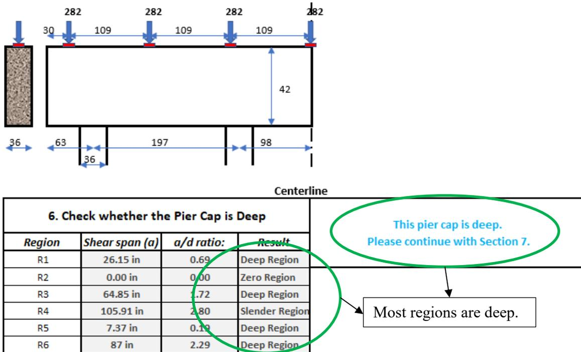
**Figure 5-14:** STM-CAP deep beam check (all units are in inches) for Bridge 3
