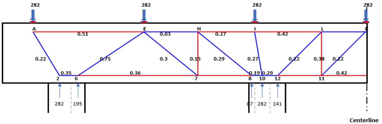
Figure 5-15: STM-CAP output model with utilization ratios for Bridge 3
