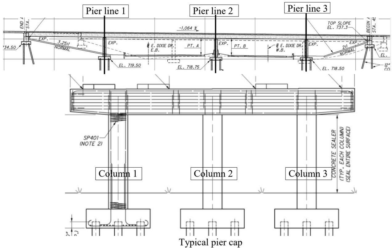
**Figure 5-1: Pier cap details for Bridge 1**
