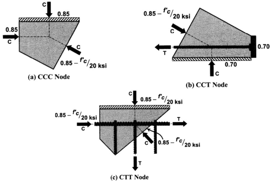
**Figure 8-2:** Concrete efficiency factor (AASHTO Figure and Table C5.8.2.5.3a-1)
