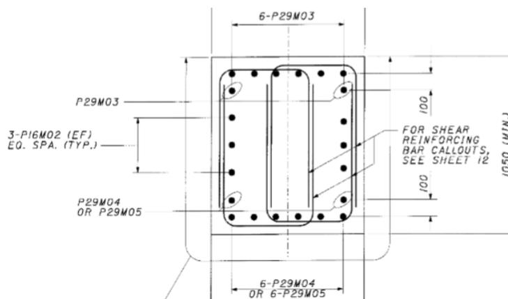
**Figure 6-38:** Section A-A of the beam for Bridge 3
