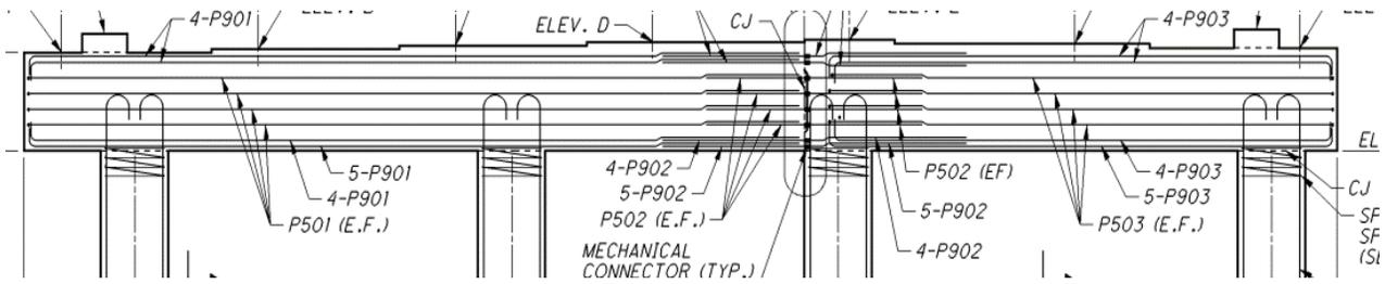
Figure 5-19: Pier cap elevation for Bridge 4
