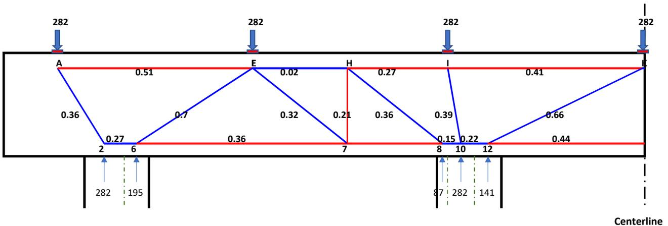
**Note:** The above figure shows the output model with Utilization Ratio along with the member which are color coded. The node numbers are also printed for every node. This output model is based on below calculation details.
