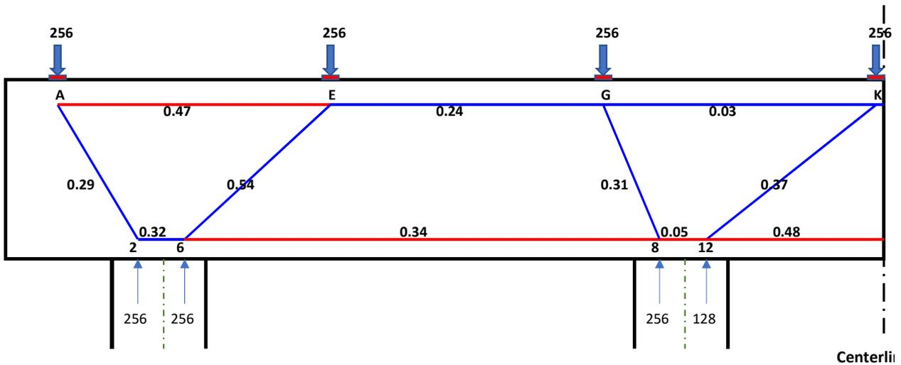
**Note:** The above figure shows the output model with Utilization Ratio along with the member which are color coded. The node numbers are also printed for every node. This output model is based on below calculation details.
