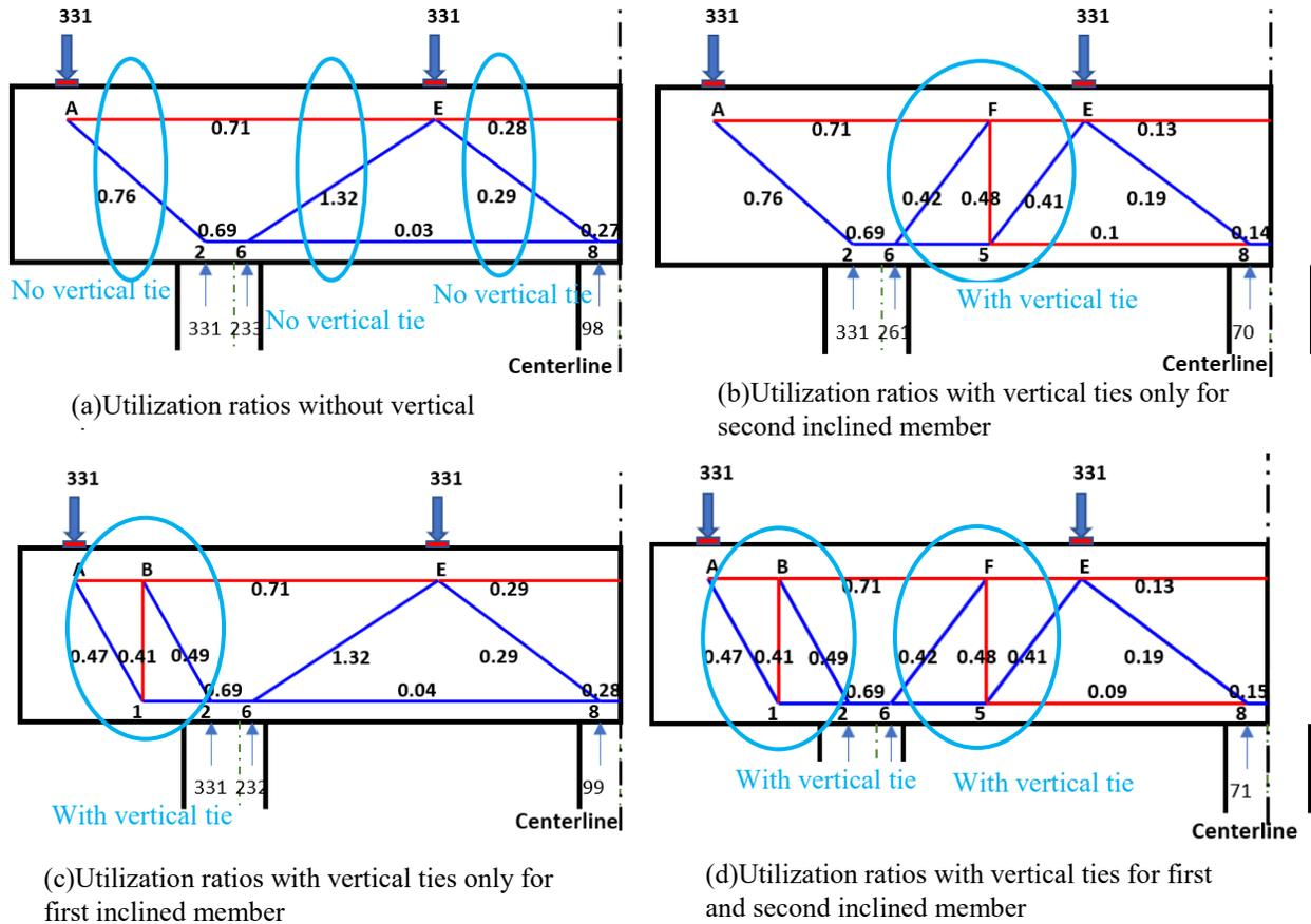
**Figure 4-23:** Optimization of utilization ratios with various truss models.
