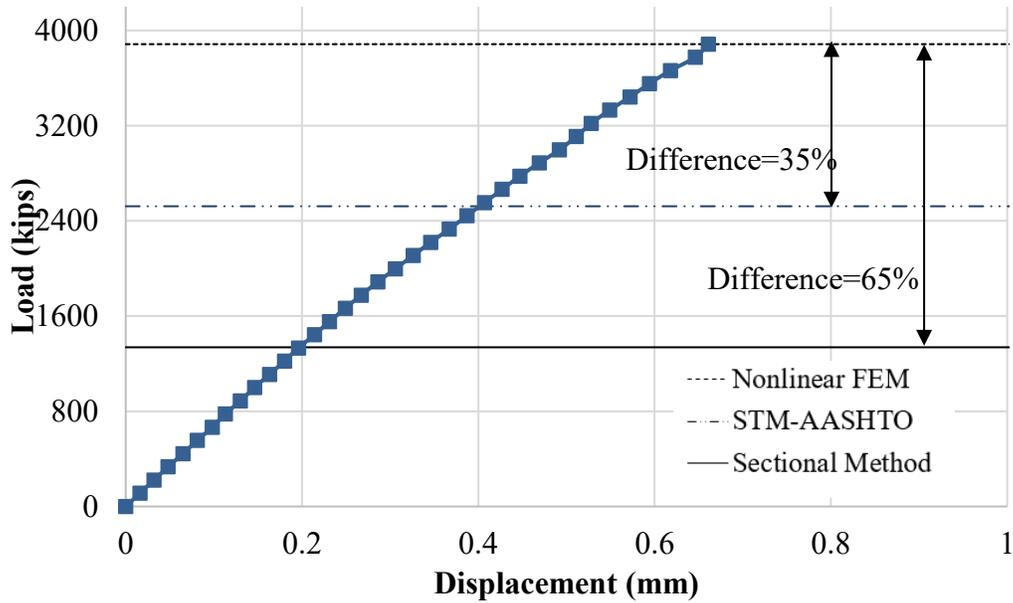
**Figure 6-63:** Load vs displacement response of cap beam for Bridge 5
