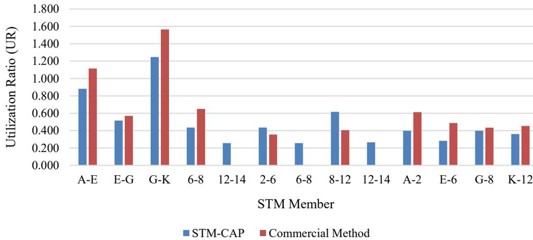
**Figure 9-4:** STM-CAP and commercial method UR comparison Pier Cap 1
