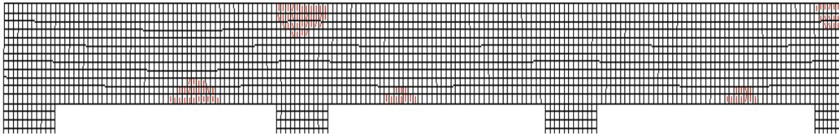
**Figure 6-62:** Cracking pattern at factored load for Bridge 5
