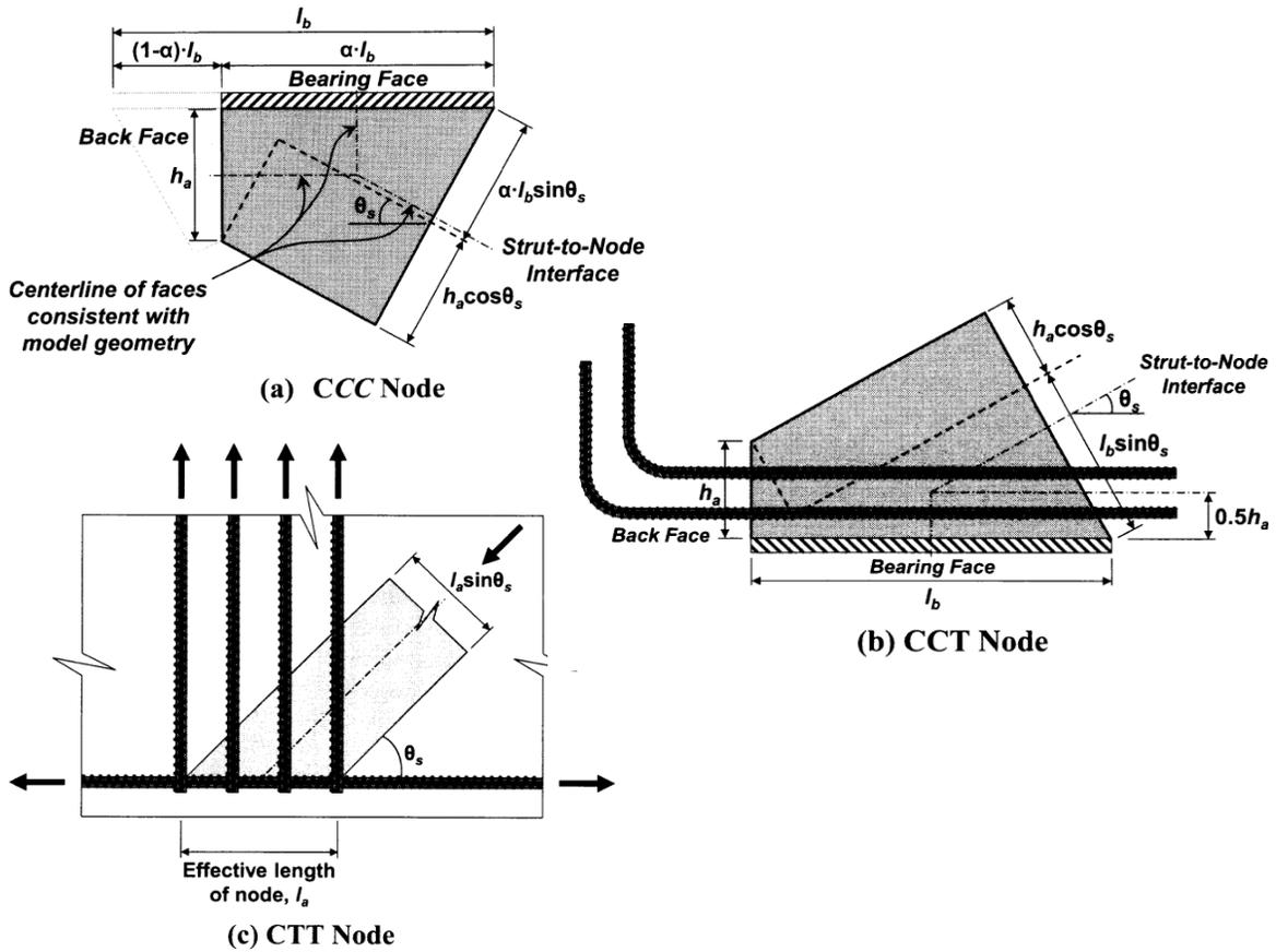
**Figure 8-1:** Nodal geometry and width of the node faces (AASHTO Figure 5.8.2.2-1)
