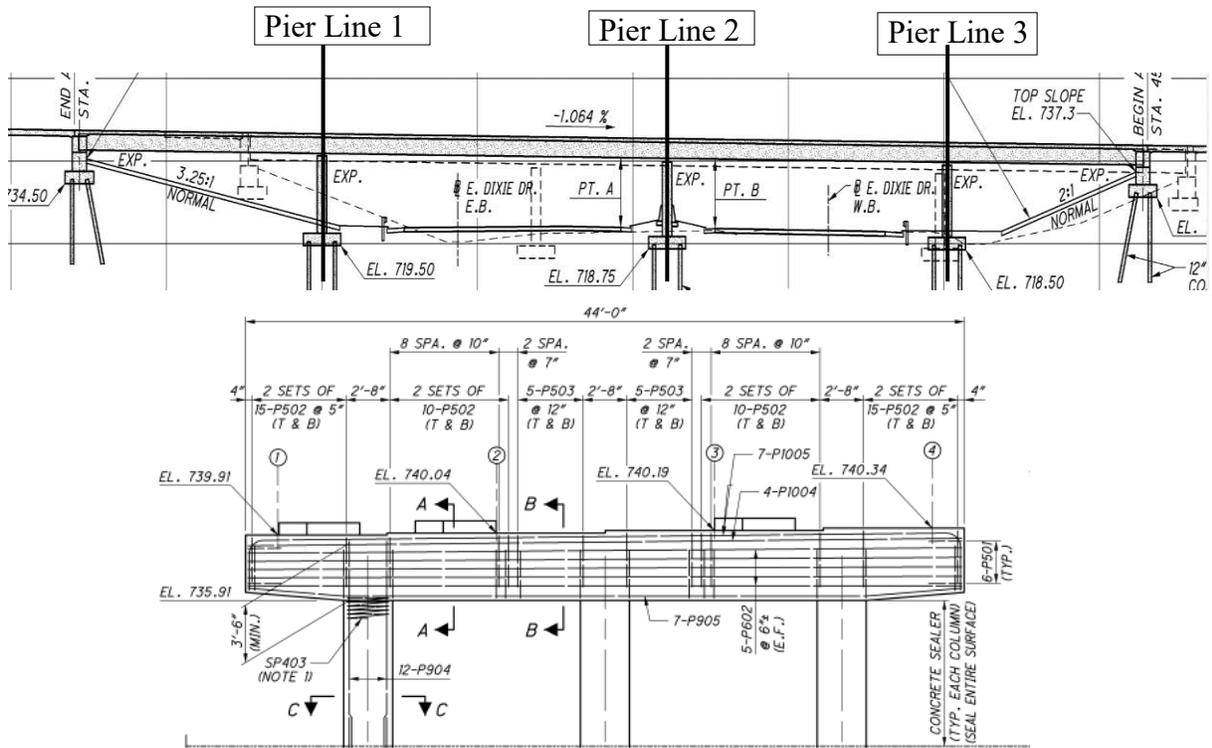
Figure 6-2: Pier cap details for Bridge 1
