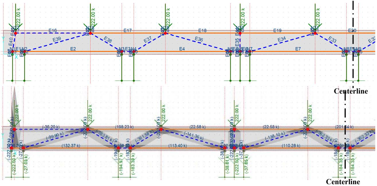
**Figure 5-29:** CAST model for the strut-and-tie method for Bridge 5
