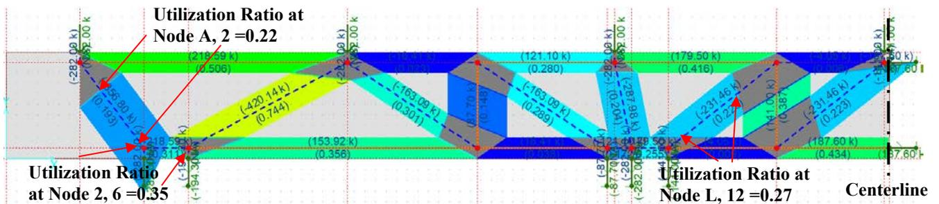
**Figure 5-18:** CAST analysis output for Bridge 3
