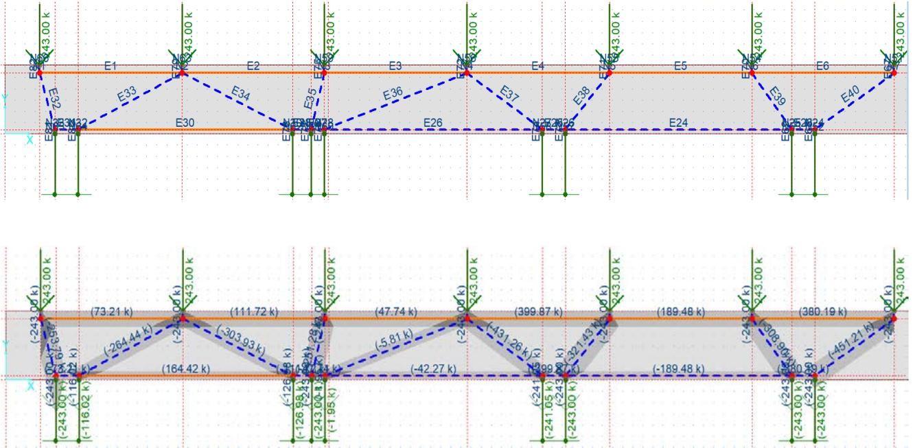
**Figure 5-35:** CAST model for the strut-and-tie method for Bridge 6
