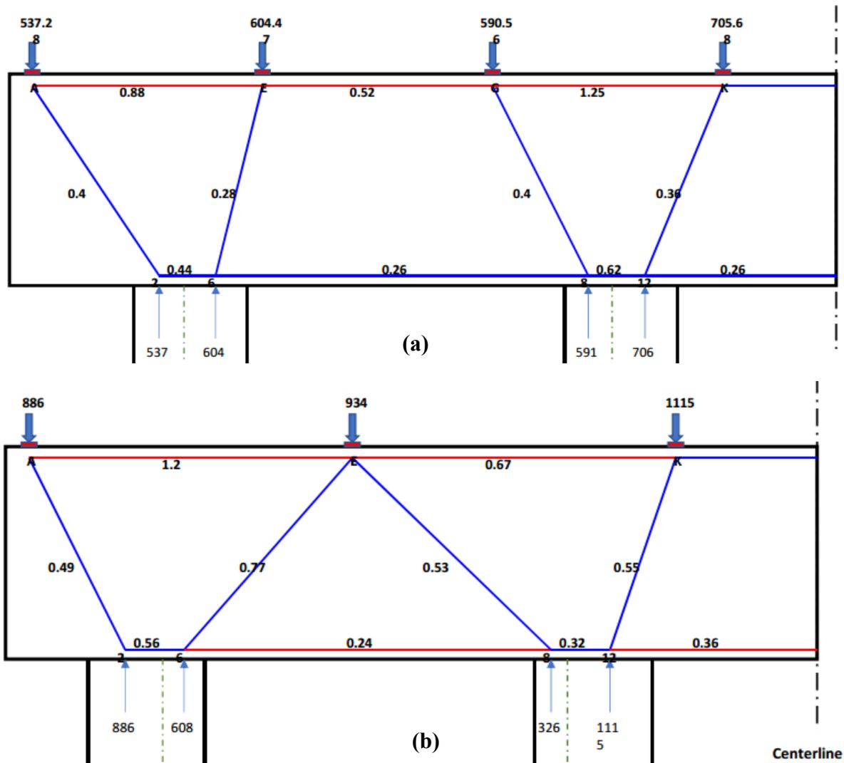
Figure 9-3: STM-CAP utilization ratio for (a) Pier Cap 1; (b) Pier Cap 2
