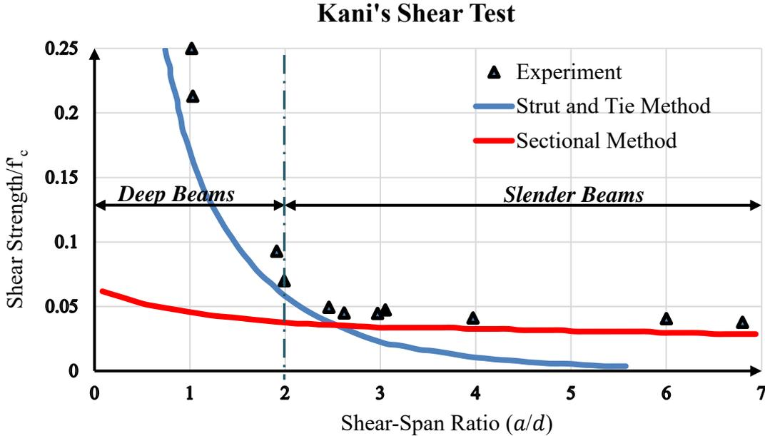
**Figure 2-2:** Shear strength vs  $a/d$  ratio (Kani, 1964)
