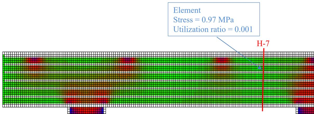
**Figure 6-32:** Smearred reinforcement stresses and utilization ratio at factored load, Bridge 2
