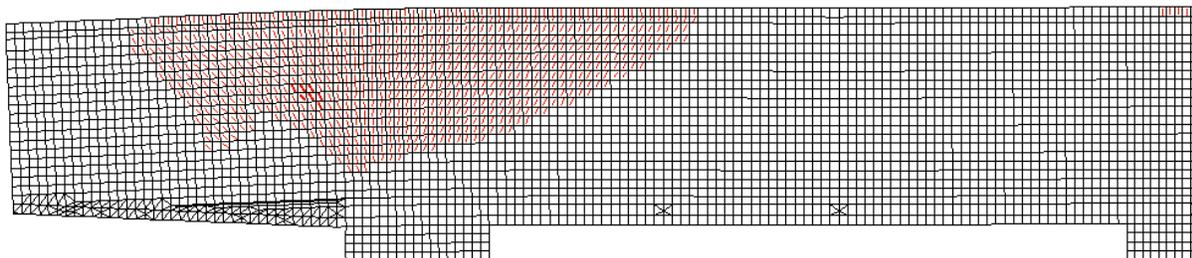
**Figure 6-25:** Cracking pattern at factored load for Bridge 1
