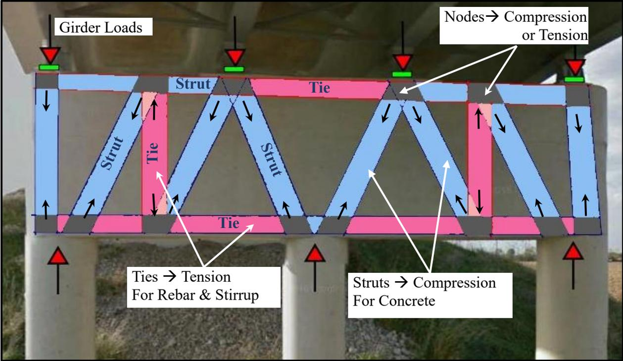
**Figure 3-4:** Strut-and-tie model idealization in real-life scenario
