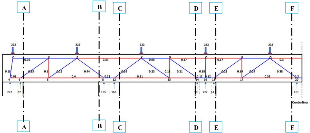
Figure 7-16: Utilization ratios calculated from STM-CAP for Bridge 4
