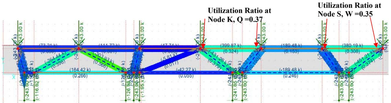
**Figure 5-36:** CAST analysis output for Bridge 6
