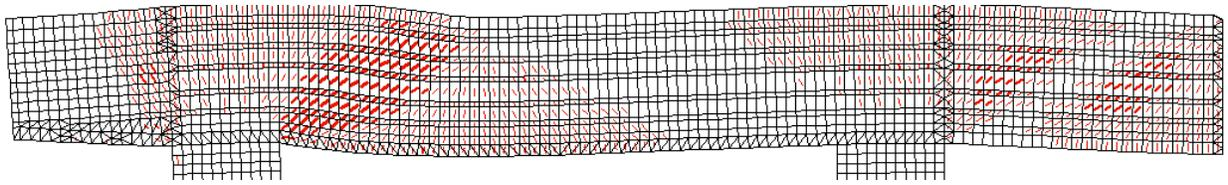
**Figure 6-43:** Cracking pattern at failure load for Bridge 3
