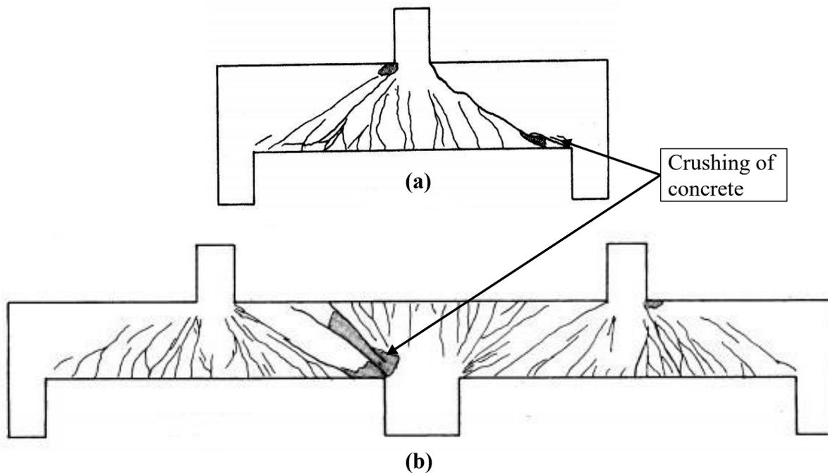
**Figure 2-3:** Typical failure in (a) simply supported; (b) continuous cap (Rogowsky, 1983)
