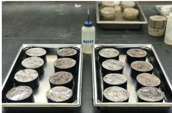
Figure 3.7: Water absorption test setup
