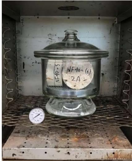
Figure 3.6: Concrete discs put in desiccator for conditioning
