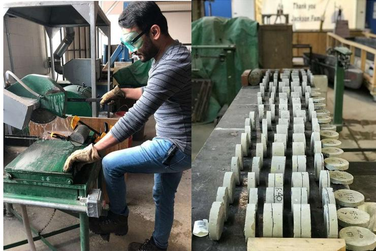
Figure 3.2: (a) Water-cooled diamond studded saw cutter (b) and discs sawn using saw-cutter.
