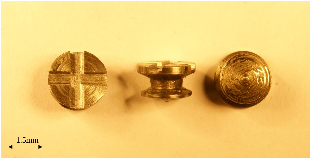
Figure 1-4. Friction stir rivet
