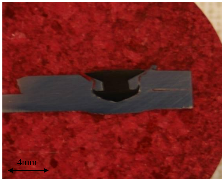
Figure 2-10. Damaged rivet bottom flange
