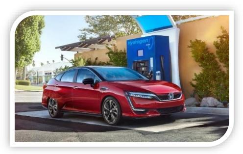
The 2020 Honda Clarity Fuel Cell Vehicle is fed by a 103kw fuel cell stack and 1.7kwh lithium ion battery pack, and yields a rating of 360 mpg/69 city/67 highway.
