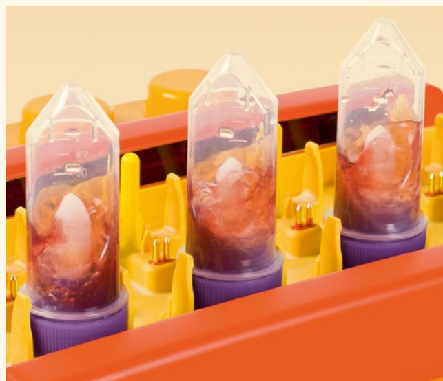
Figure 2: gentleMACS Tubes processing samples on the gentleMACS Octo Dissociator.
