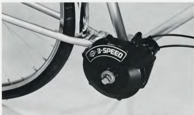
**STEP THREE:** Install transmission onto mainshaft
