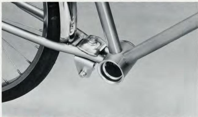
**STEP ONE:** Remove existing chain guard, pedals, crank, large sprocket bearings and cones.
