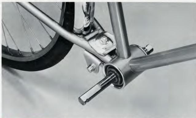
**STEP TWO:** Install new mainshaft utilizing existing bearings and cones.
