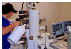
SEM with a STEM detector, EDS, and EBIC applications
