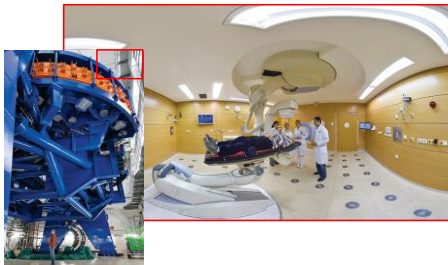
Radiation treatment room in the Heidelberg Ion-Beam Therapy Center HIT. The beam exits the gantry (weighs ~670 tons, RT room on top). Two rotation systems and digital X-rays are used to optimize the position of the patient guided by the images taken before irradiation.
