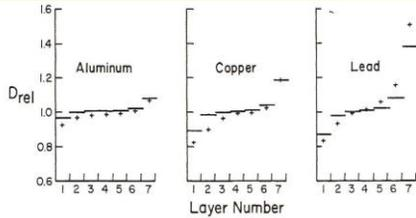
FIGURE 10.10. The average dose to a given layer of a seven-layer stack of LiF dosimeters divided by the equilibrium LiF dose, as calculated using the Kearsley model (bars) and as measured by Ogunleye et al. (+) for Al, Cu, and Pb walls. (After Kearsley, 1984b. Reproduced with permission from E. E. Kearsley and The Institute of Physics, U.K.)
