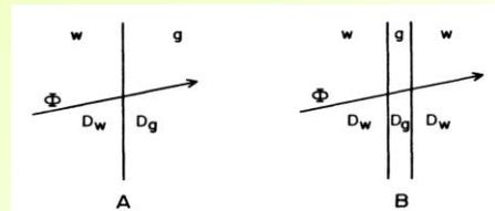
(A) A fluence  $\Phi$  of charged particles crossing an interface between media w and g
