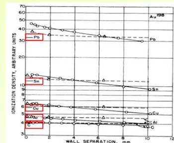
Comparison of measured ionization densities (solid curves) in flat air-filled ion chambers having various wall materials and adjustable gap widths, with Bragg-Gray theory (tick marks at left) and Spencer theory (dashed curves), for  $^{198}\text{Au}$   $\gamma$  rays
