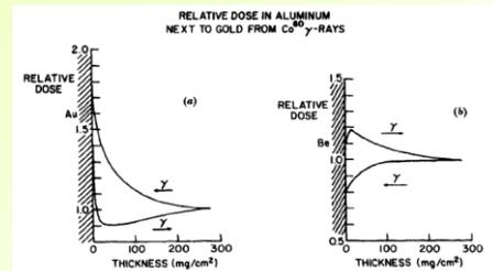
FIGURE 10.12. Variation of dose and electron fluence in aluminum as a function of distance from an interface with (a) gold, (b) beryllium. Arrows indicate the direction of  $^{60}\text{Co}$   $\gamma$  rays. (After Wall and Burke, personal communication, 1976.)
