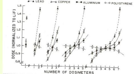
FIGURE 10.8. Relative absorbed dose in individual TLD layers in the experiment described in Fig. 10.7.  $^{60}\text{Co}$   $\gamma$ -rays pass from left to right in relation to this graph. (After Ogunleye et al., 1980. Reproduced with permission of The Institute of Physics, U.K.)
