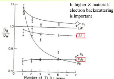
FIGURE 10.9. Comparison of the Burlin theory (solid curves) with the experiment referred to in Figs. 10.7 and 10.8. The application of the theory in this case, as described in the text, differs from that of Ogunleye et al. (1980).
