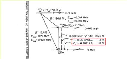
FIGURE 5.9. Atomic energy-level diagram for  $^{137}\text{Cs} \rightarrow ^{137}\text{Ba}$ , illustrating competition between  $\gamma$ -ray emission and internal conversion. Percentages all refer to disintegrations of parent atoms of  $^{137}\text{Cs}$ . ( $\alpha/\gamma = 0.0916$ ,  $R/(L + M + \dots) = 4.41$ .)
