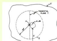
FIGURE 4.1. Radiation equilibrium. Extended volume  $V$  contains a homogeneous medium and a homogeneous isotropic source distribution. Radiation equilibrium will exist in the smaller internal volume  $v$  if the maximum distance ( $d$ ) of primary rays plus their secondaries is less than the minimum separation ( $s$ ) of  $v$  from the boundary of  $V$ . Neutrons are ignored. (See text.)
