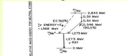
FIGURE 5.8. Atomic energy-level diagram for  $\beta^{+}$  and EC disintegration of  $^{22}_{11}\text{Na}$  ( $\tau_{1/2} = 2.60 \text{ y}$ ) to  $^{22}_{10}\text{Ne}$ . ( $E_{\beta^{+}})_{\max} = 0.546 \text{ MeV}$ ;  $E_{\gamma} = 0.216 \text{ MeV}$ .
