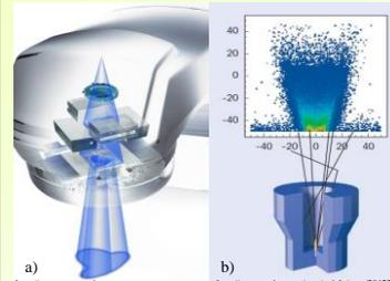
Azimuthal symmetry: a) accelerator beam after primary collimator; b) brachytherapy surface applicator
