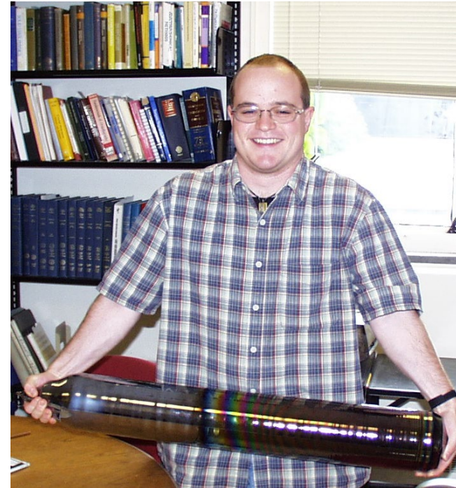
Laif Alden with a Si single crystal grown by the Czochralski method
