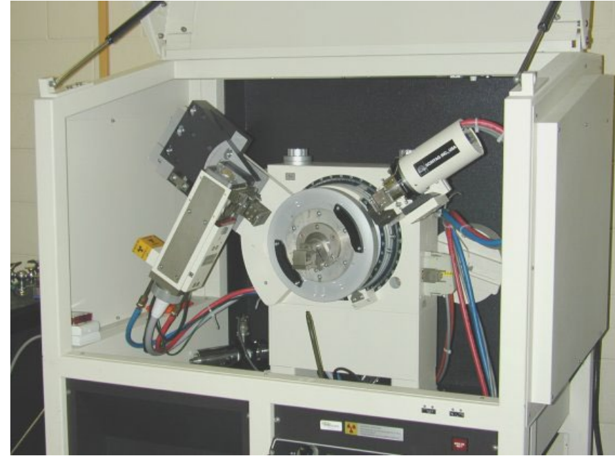
Scintag theta-theta diffractometer with Peltier cooled solid-state detector
