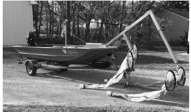
Boat and nets used to sample rivers for grass carp eggs and larvae.
