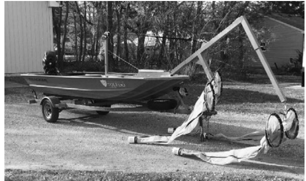
Boat and nets used to sample rivers for grass carp eggs and larvae.
