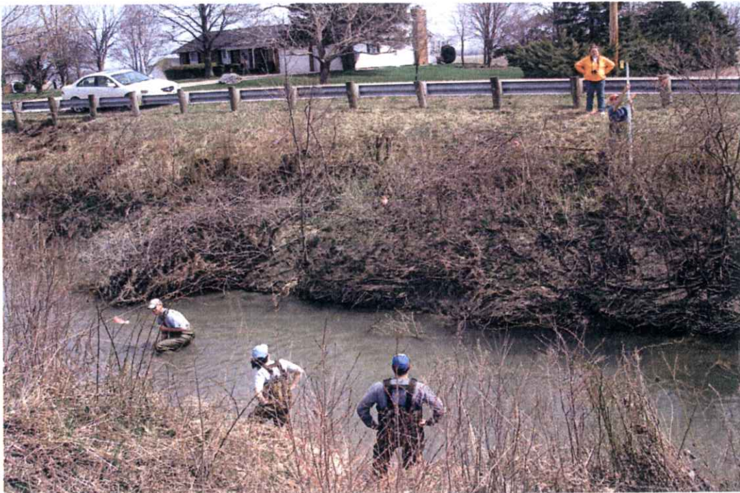
PHOTO 6: University of Toledo students surveying cross section at Field Site 2.
