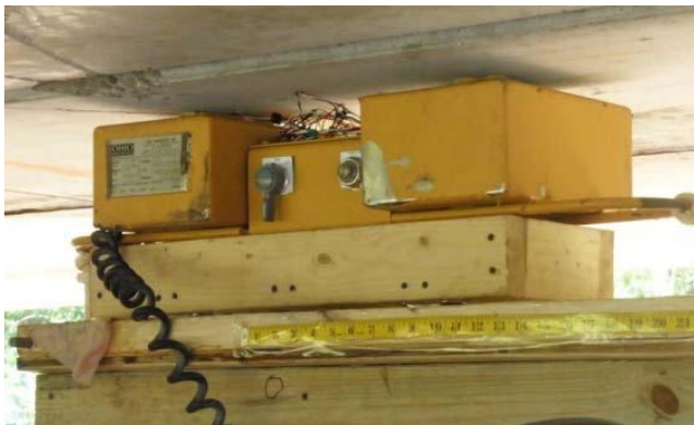
IMF sensing equipment, electromagnet with Hall sensors on pole face
