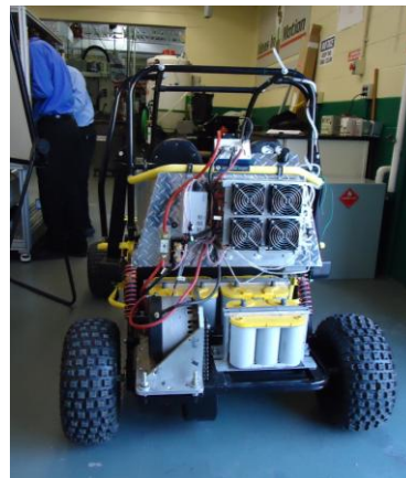
The back of the hydrogen fuel cell battery hybrid go-kart. The hydrogen cylinders filled from the automated fueling station are behind the fan units above the batteries.
