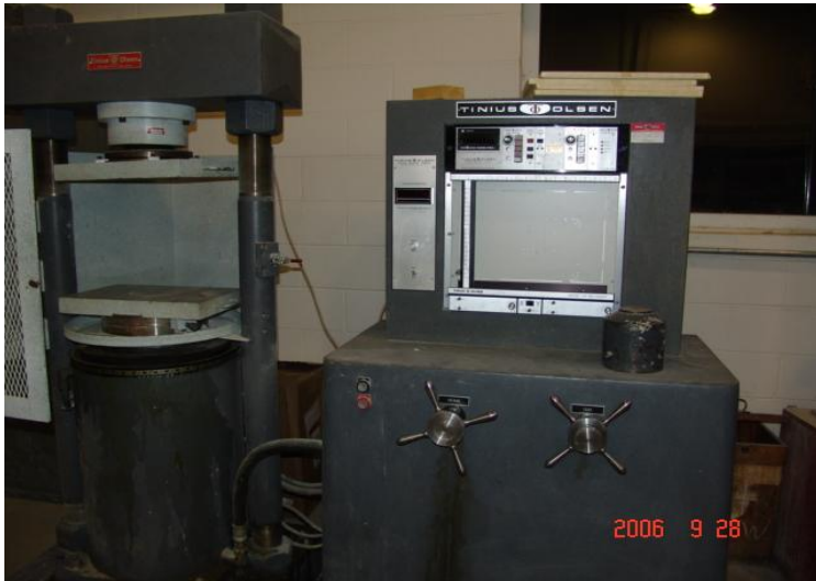
Concrete Compression 400 kip machine.
